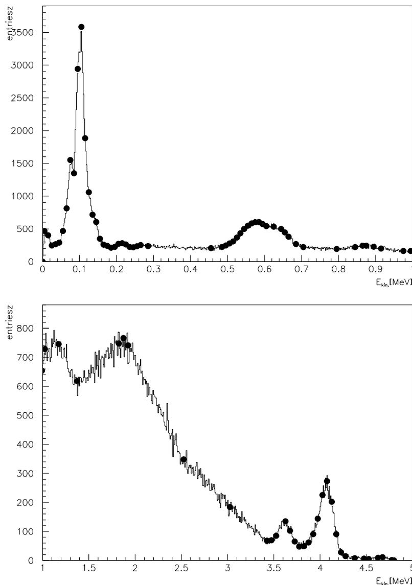
**Figure 3: Comparison of data and Monte Carlo for photon energy distributions for radiative capture of 15 MeV neutrons on Uranium ( $^{238}\text{U}$ ). The points are evaluated data, the histogram is the Monte Carlo prediction.**
