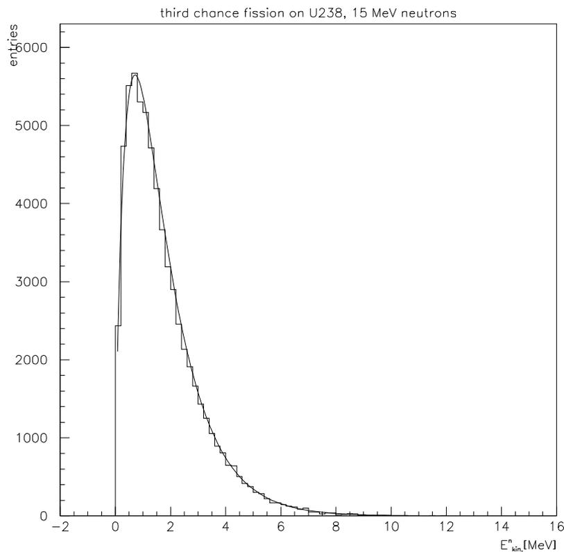
**Figure 4: Comparison of data and Monte Carlo for fission neutron energy distributions for induced fission by 15 MeV neutrons on Uranium ( $^{238}\text{U}$ ). The curve represents evaluated data and the histogram is the Monte Carlo prediction.**
