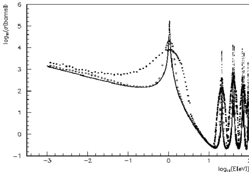
**Figure 1: neutron capture cross-section on Plutonium at several temperatures. The material, energies, and temperatures have been chosen to mirror the standard BROADR verification plot.**
