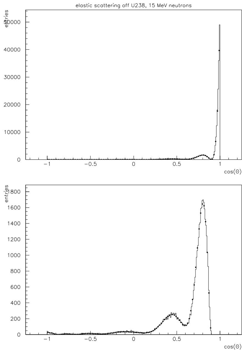
**Figure 2: Comparison of data and Monte Carlo for the angular distribution of 15 MeV neutrons scattered elastically off Uranium ( $^{238}\text{U}$ ). The points are evaluated data, and the histogram is the Monte Carlo prediction. The lower plot excludes the forward peak, to better show the Frenel structure of the angular distribution of the scattered neutron.**
