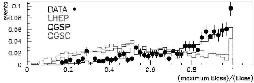
**Figure 2:** This plot shows results from a ATLAS pixel test-beam, using 180 GeV pions. The signal ratio between the hottest pixel to all signal in the cluster of active pixels is shown[7].
