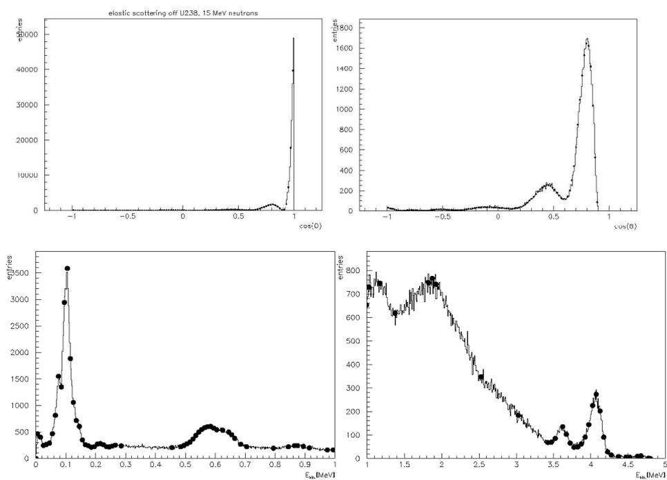
**Figure 4: Comparison of the sampling result of the neutron transport code with the cross-sections from G4NDL3.7. The top plots show elastic scattering angular distributions, left with, and right without the forward peak. The lower plots show the energy of gammas from neutron capture.**
