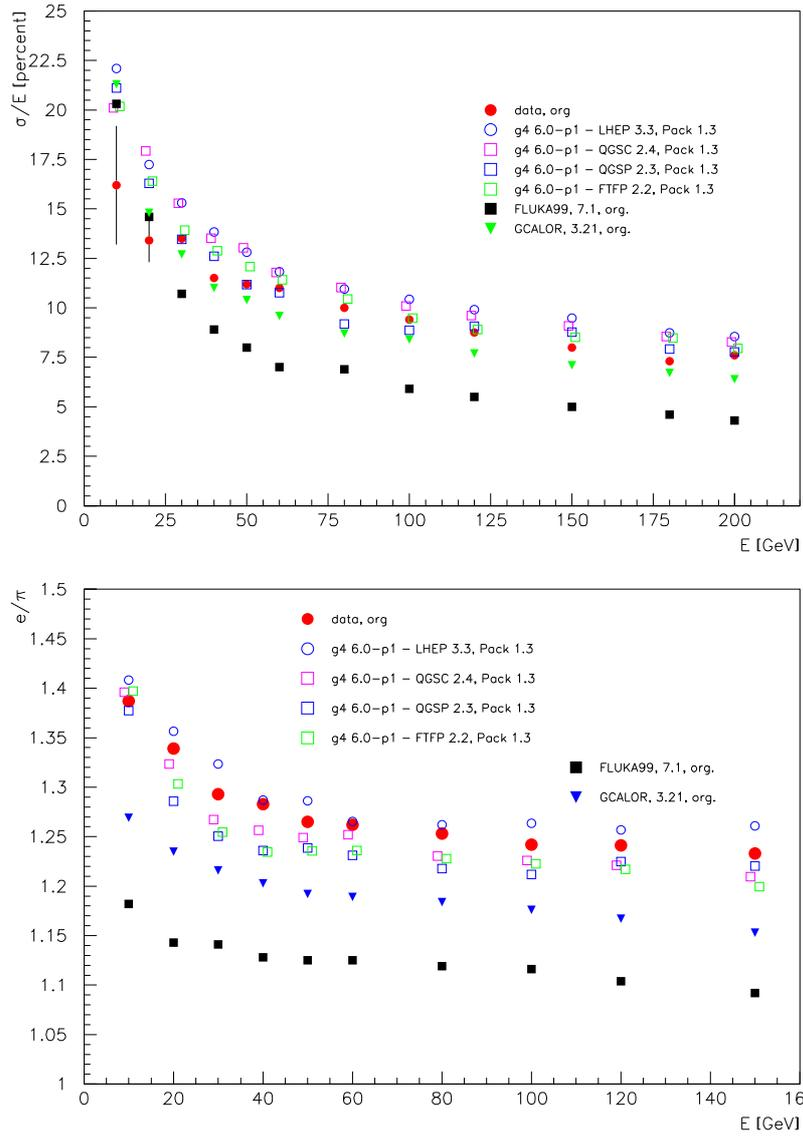
**Figure 1: The energy resolution and the signal ratio of electrons to pions in the ATLAS End-Cap hadronic calorimeter as predicted with QGSP and LHEP. Data are taken from [6]**
