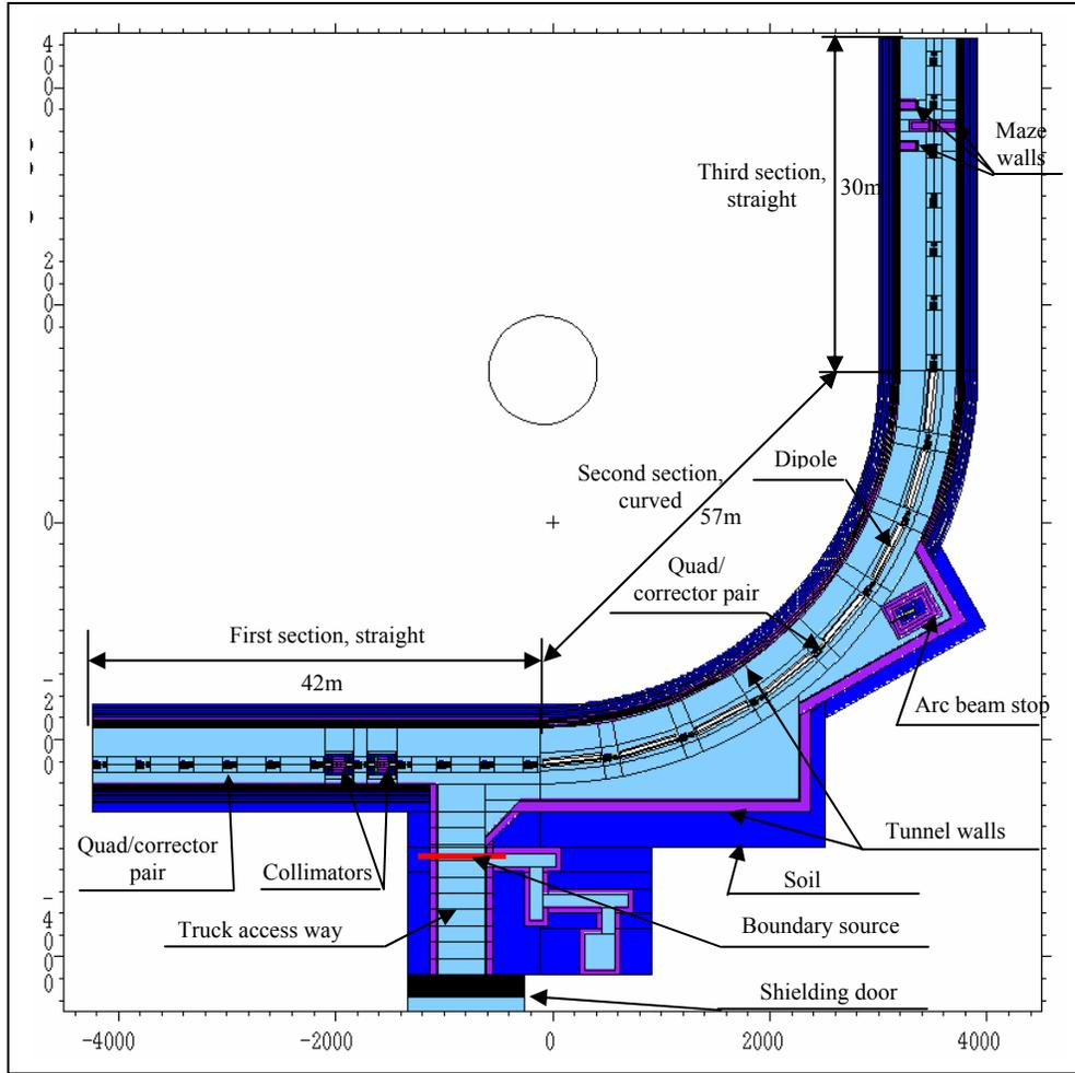
**Figure 1. MCNPX model for HEBT**
