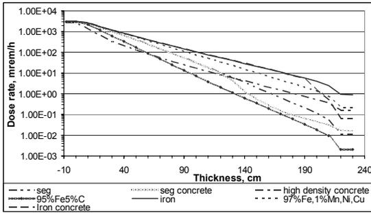
**Figure 2.** Dose rate distribution inside a shielding door made from different materials, calculated by Monte Carlo code MCNPX; mrem/h.
