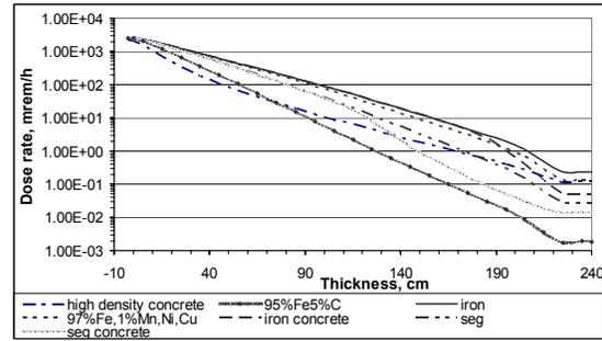
**Figure 3.** Dose rate distribution inside a shielding door made from different materials, calculated by discrete ordinates code DORT; mrem/h.
