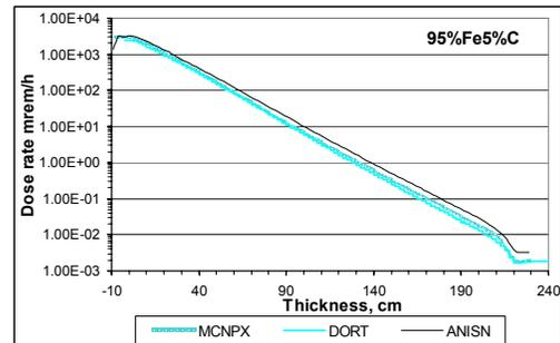
**Figure 7.** Dose rate distribution inside a cast-iron shielding door, calculated by Monte Carlo code MCNPX and discrete ordinates code DORT; mrem/h.
