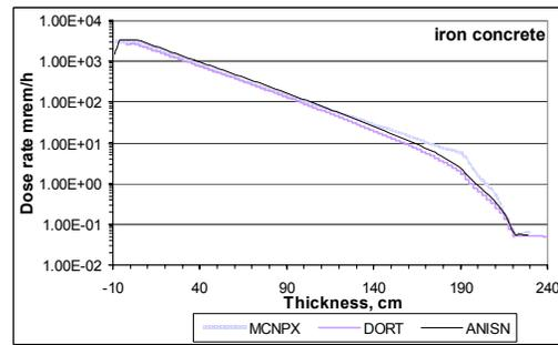
**Figure 5.** Dose rate distribution inside a shielding door of 1.9 m iron followed by 0.3 m concrete, calculated by Monte Carlo code MCNPX and discrete ordinates code DORT; mrem/h.
