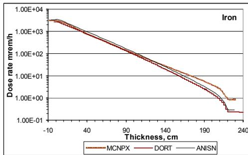
**Figure 4.** Dose rate distribution inside an iron shielding door, calculated by Monte Carlo code MCNPX and discrete ordinates code DORT; mrem/h.
