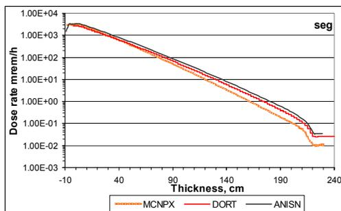
**Figure 8.** Dose rate distribution inside the SEG steel shielding door, calculated by Monte Carlo code MCNPX and discrete ordinates code DORT; mrem/h.
