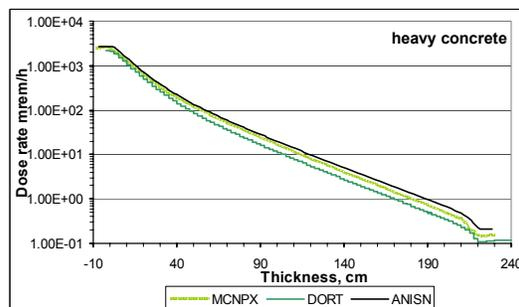
**Figure 9.** Dose rate distribution inside a high density concrete shielding door, calculated by Monte Carlo code MCNPX and discrete ordinates code DORT; mrem/h.
