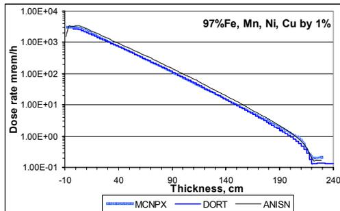
**Figure 6.** Dose rate distribution inside a steel shielding door, calculated by Monte Carlo code MCNPX and discrete ordinates code DORT; mrem/h.
