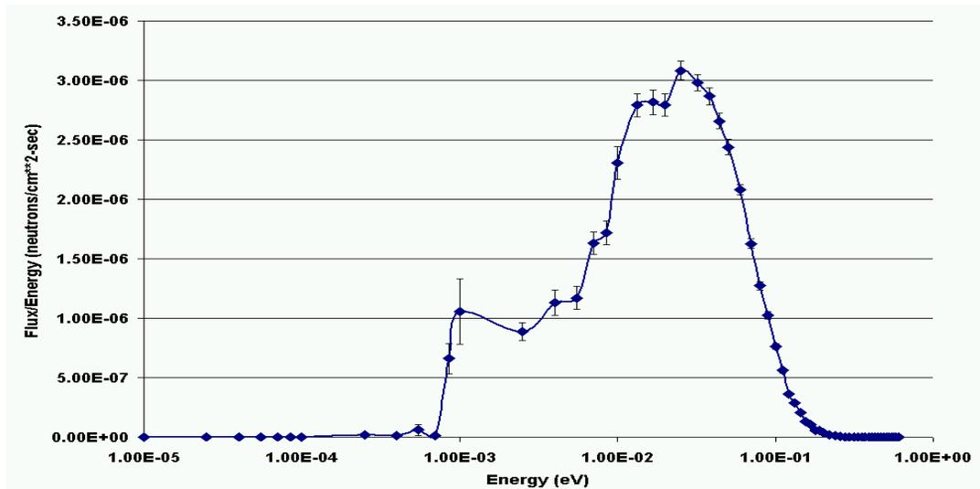
Figure 12. Neutron spectrum at the entrance of the beam port 7
