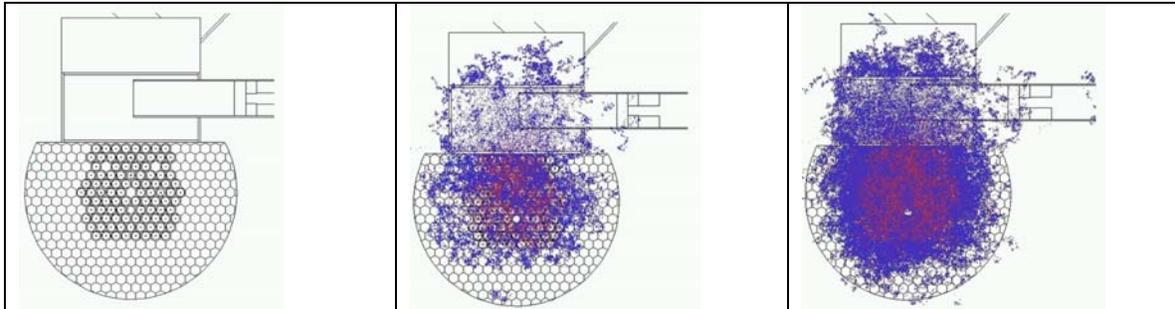
Figure 9. Neutron collision points in the combined model
