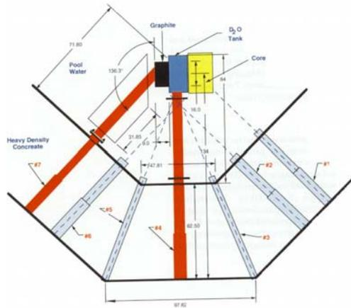
Figure 1. PSBR beam port layout with D2O tank and graphite reflector
