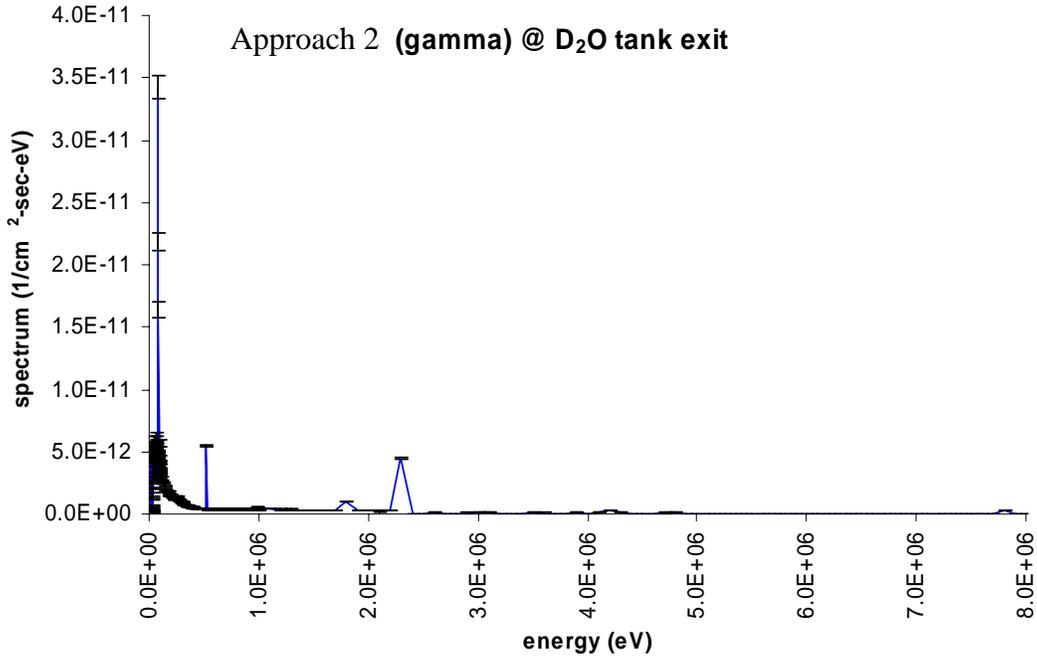
Figure 7. Gamma spectrum at the end of the beam port entry hole for Approach 2.
