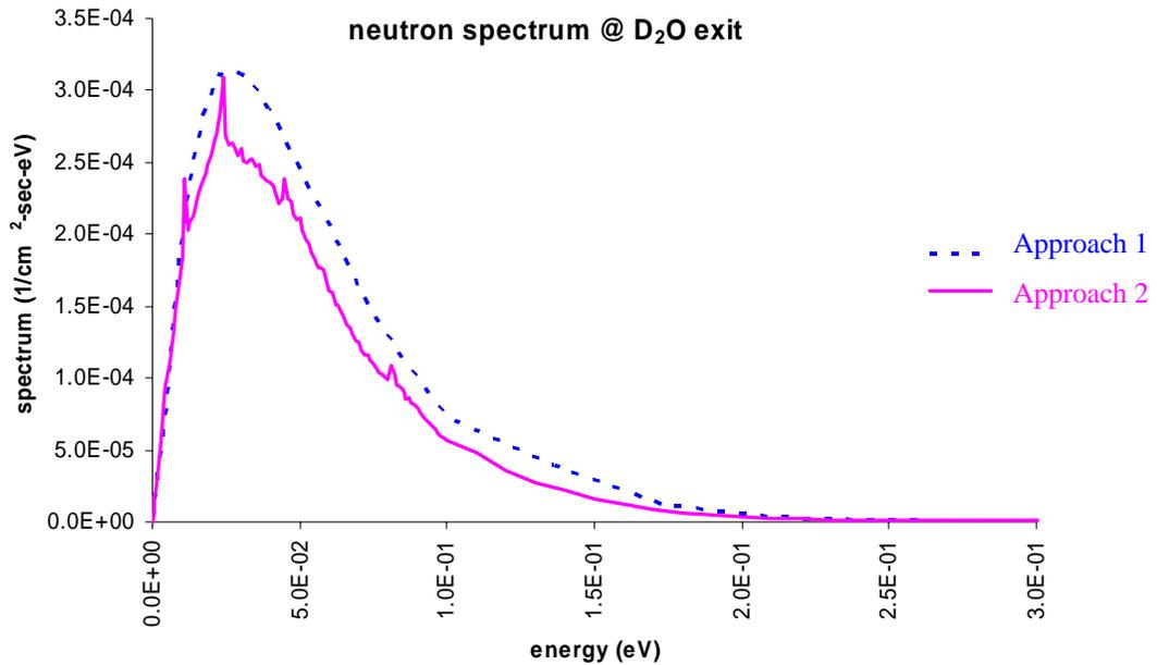
Figure 5. Neutron spectrum at the end of the beam port entry hole for both methodologies.
