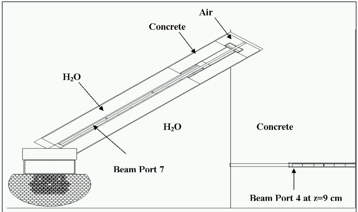
Figure 11. Beam port seven in the combined model
