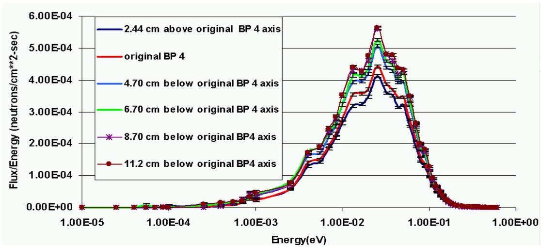
Figure 10. Neutron spectrum variance with changing the location of beam port 4
