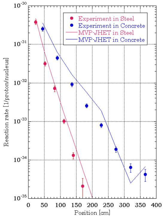
Figure 12.  $^{27}\text{Al}(n,x)^{24}\text{Na}$  reaction rates in steel and concrete by neutrons from mercury target bombarded by 2.83 GeV protons at AGS.
