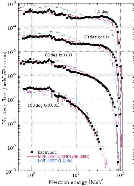
**Figure 1. Angular neutron spectra by MVP-JHET from C target irradiated by 113 MeV protons at WNR.**
