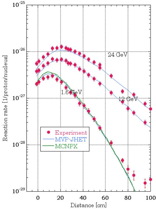
Figure 9.  $^{115}\text{In}(n,n')^{115m}\text{In}$  reaction rates on axis direction around mercury target bombarded by protons at AGS.
