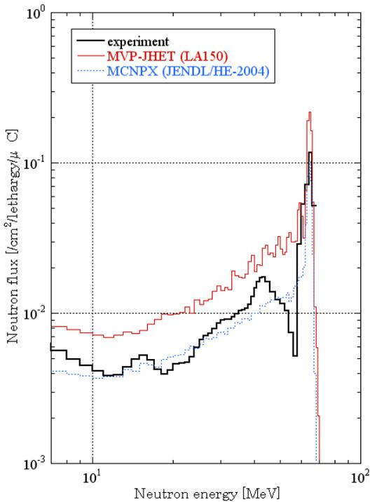
**Figure 7. Leakage neutron spectra on beam axis from Fe 130 cm assembly irradiated by neutrons of  $p_7\text{Li}$  at TIARA.**
