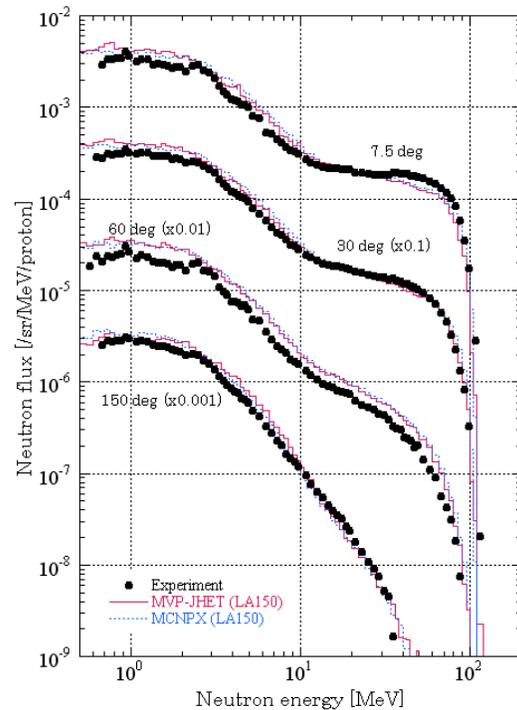
**Figure 4. Angular neutron spectra by MVP-JHET and MCNPX from Fe target irradiated by 113 MeV protons at WNR.**
