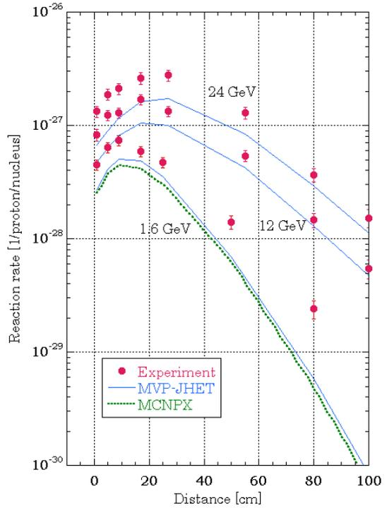
Figure 10.  $^{209}\text{Bi}(n,4n)^{206}\text{Bi}$  reaction rates on axis direction around mercury target bombarded by protons at AGS.
