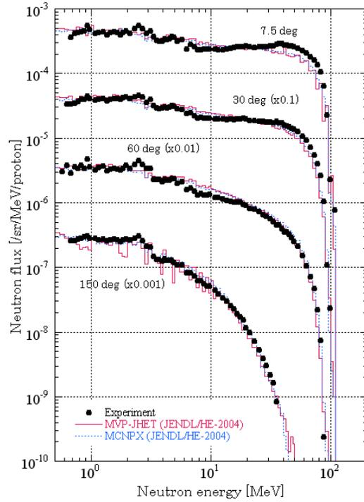
**Figure 2. Angular neutron spectra by MVP-JHET and MCNPX from C target irradiated by 113 MeV protons at WNR.**
