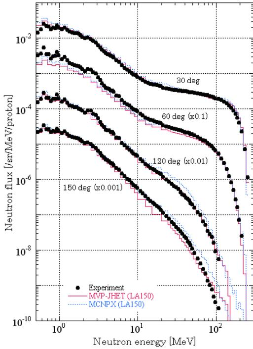
**Figure 5. Angular neutron spectra by MVP-JHET and MCNPX from Fe target irradiated by 256 MeV protons at WNR.**
