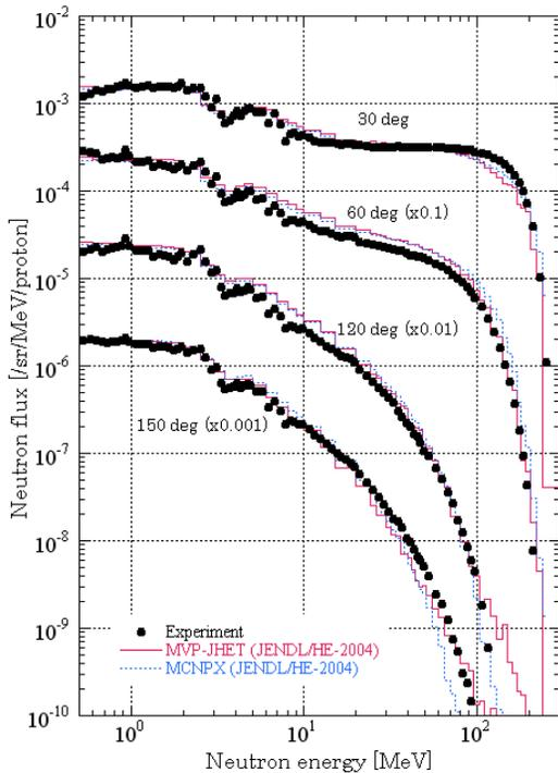
**Figure 3. Angular neutron spectra by MVP-JHET and MCNPX from C target irradiated by 256 MeV protons at WNR.**
