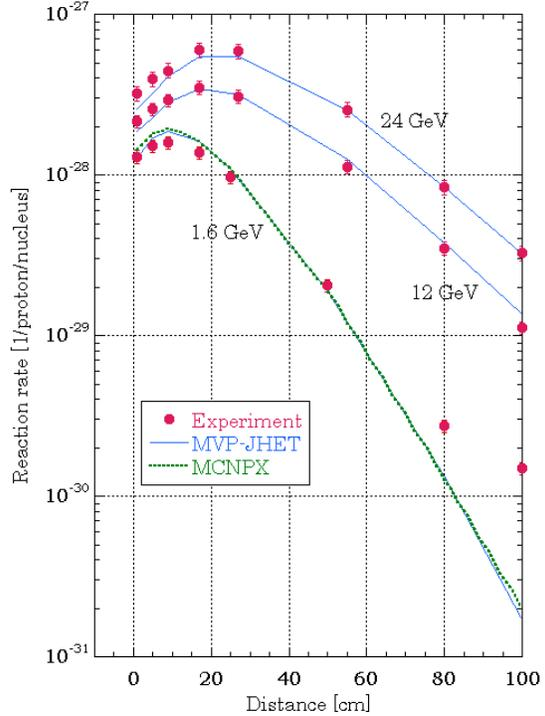
**Figure 8.  $^{27}\text{Al}(n,x)^{24}\text{Na}$  reaction rates on axis direction around mercury target bombarded by protons at AGS.**
