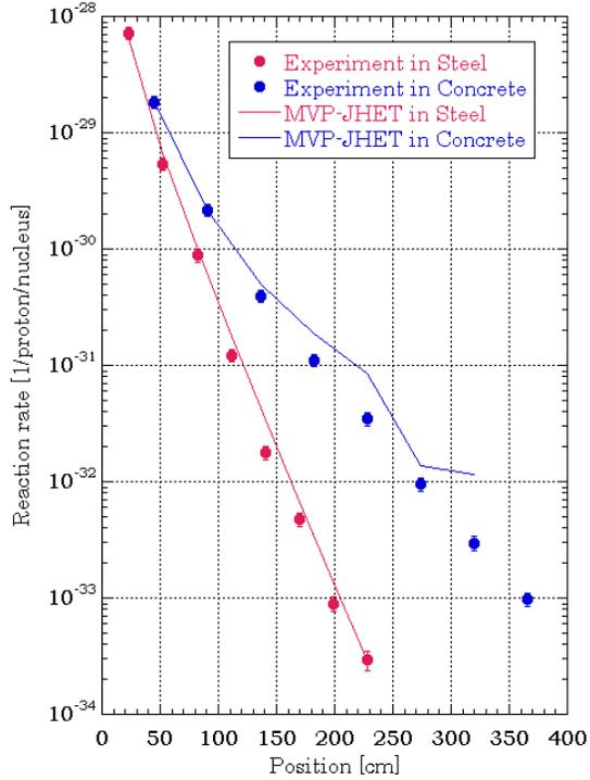
Figure 13.  $^{115}\text{In}(n,n')^{115\text{m}}\text{In}$  reaction rates in steel and concrete by neutrons from mercury target bombarded by 24 GeV protons at AGS.
