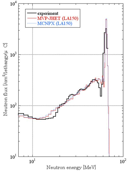
**Figure 6. Leakage neutron spectra on beam axis from Fe 40 cm assembly irradiated by neutrons of  $p_7\text{Li}$  at TIARA.**
