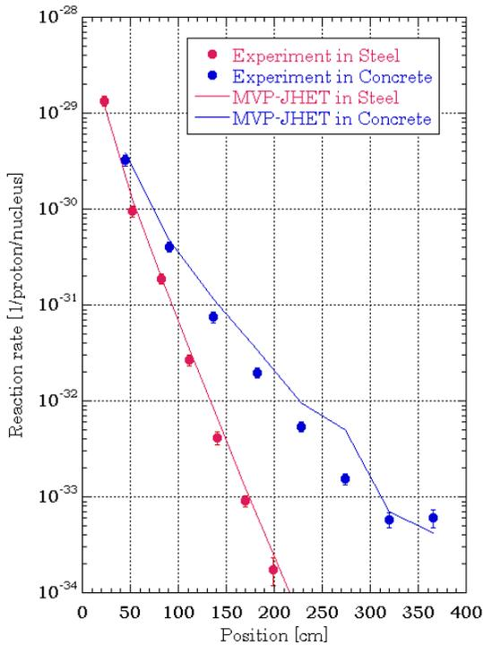
Figure 11.  $^{115}\text{In}(n,n')^{115m}\text{In}$  reaction rates in steel and concrete by neutrons from mercury target bombarded by 2.83 GeV protons at AGS.
