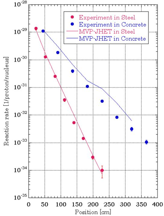
Figure 14.  $^{209}\text{Bi}(n,4n)^{209}\text{Bi}$  reaction rates in steel and concrete by neutrons from mercury target bombarded by 24 GeV protons at AGS.
