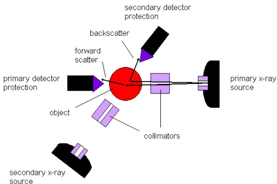
**Figure 1. Plan view of a typical Core Punch experiment at AWE**
