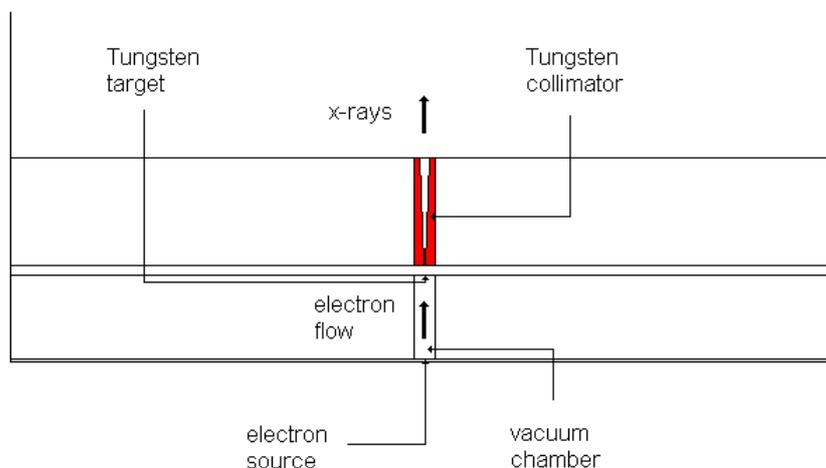
**Figure 4. Simplified LINAC source geometry**
