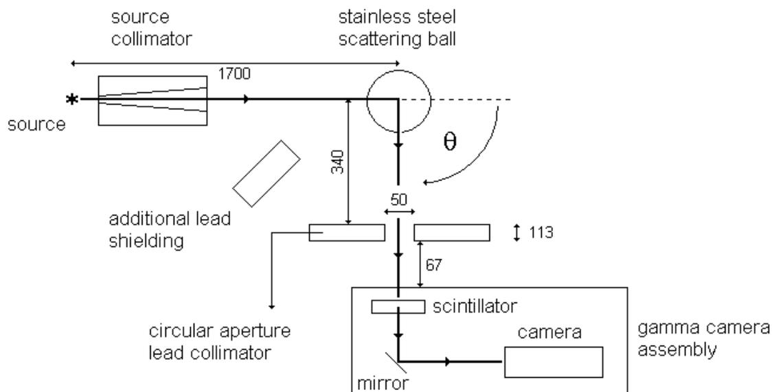
**Figure 2. Plan view of experimental geometry to investigate large angle scattering (dimensions are in mm, not to scale)**
