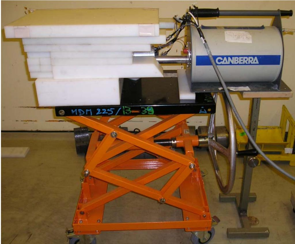
**Figure 9. Simplified experimental setup used for the Ge data test.**
