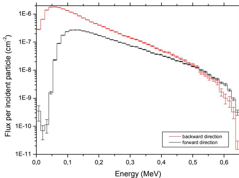
**Figure 1: Photon flux distribution at the beam stopper, forward (along) and backward (opposite) to the electron beam direction**
