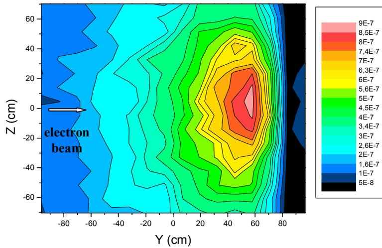
Figure 4: Photon flux impinging the lateral wall of the chamber, per incident electron
