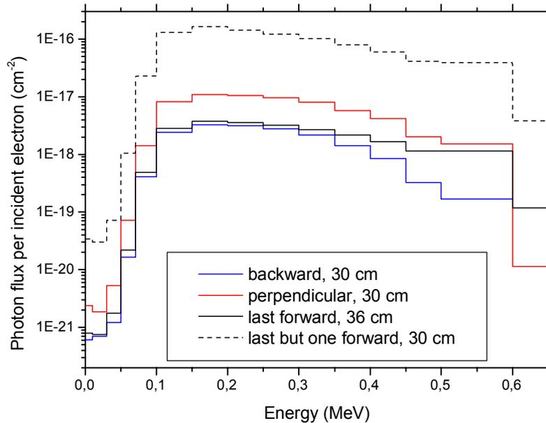
**Figure 7: Photon flux distribution per incident electron ( $\text{cm}^{-2}$ ) in different directions**
