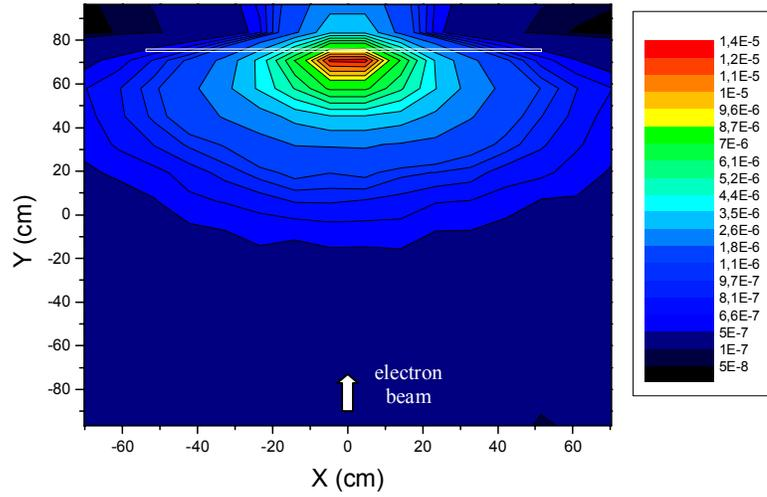
Figure 3: Photon flux per incident electron ( $\text{cm}^{-2}$ ) evaluation inside the chamber along the beam direction. The white rectangle corresponds to the beam stopper
