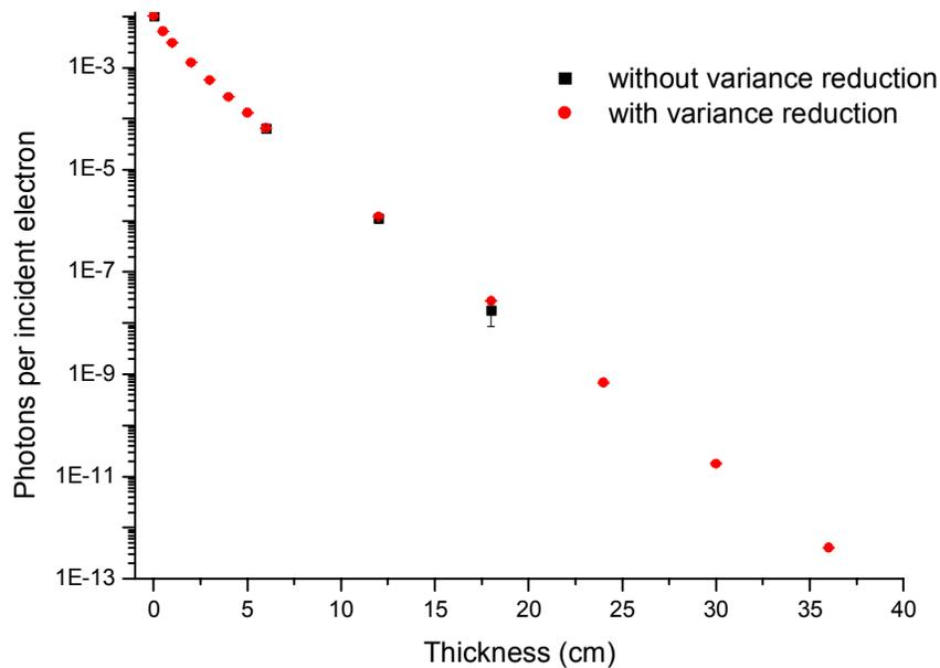
**Figure 5: Photons per incident electron. Comparison of the variance reduction results with those obtained without this technique, respectively 25 and 276 million primary electrons**
