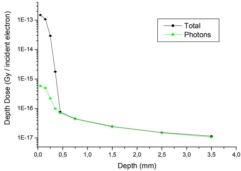
**Figure 2: Depth-dose distribution for the 650 keV/50 mA electron beam in stainless steel, showing the individual contribution from electrons and photons**
