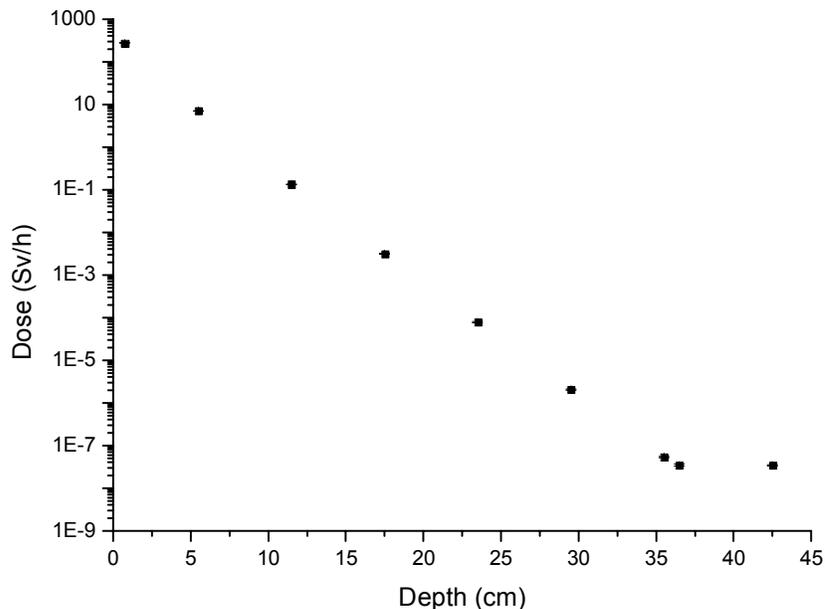
**Figure 6: Dose attenuation in the shielding (forward direction)**
