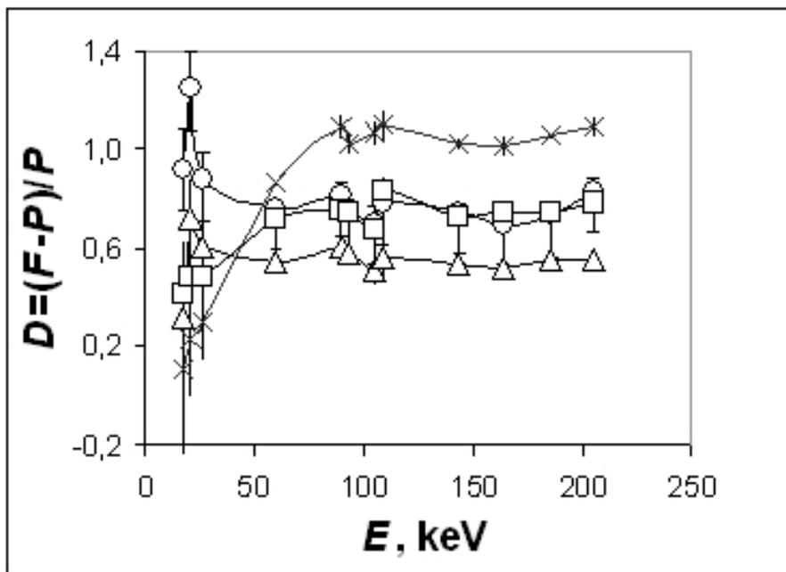
**Figure 6: Relative calculated counting efficiency for  $^{241}\text{Am}$  and  $^{235}\text{U}$  photoelectric absorption peaks for phantoms and the patient,  $D = (F - P) / P$ , where  $F$  is the result for a phantom and  $P$  is the result for the patient. ○ — the Livermore phantom, □ — the JAERI phantom, △ — the RANDO phantom, × — the Winfrith phantom.**
