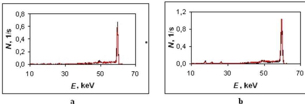
**Figure 2: Experimental (red line) and calculated (black line) spectra of the left (panel “a”) and right (panel “b”) Canberra germanium detectors during measurement of  $\gamma$ -radiation emitted by  $^{241}\text{Am}$  inserted into the lungs of the Livermore plastic phantom.**
