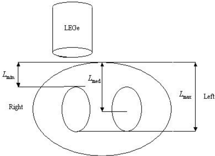
**Figure 5: Scheme of principal distances from lungs to the front surface of thorax during whole body counting with low-energy germanium detector (LEGe).  $L_{\min}$  is the minimal distance between source (lung) and front surface, it determines counting efficiency for low energies. For higher energies, maximal distance  $L_{\max}$  and median  $L_{\text{med}}$  are also essential.**
