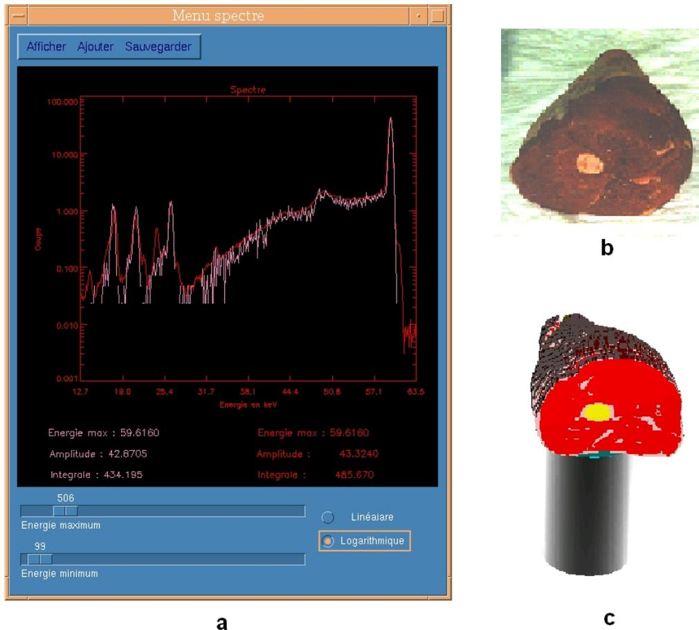
**Figure 3: Panel “a”:** experimental (red line) and calculated (pink line) pulse-height-spectra from point  $^{241}\text{Am}$  source of 32 kBq, placed into mouton meat sample counts per second per channel. Panel “b”: photo of the sample. Panel “c” – Sabrina visualization of MCNP geometry (including the detector), created by  $\text{CEDIPE}$ .
