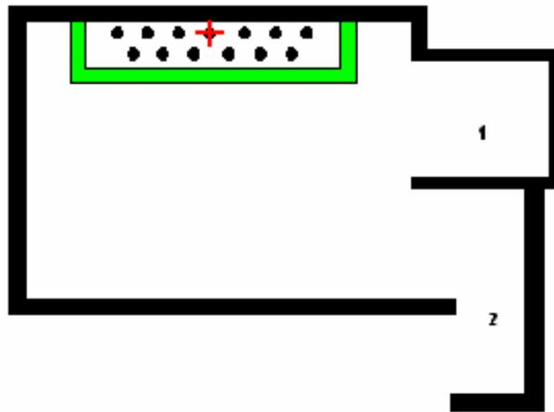
**Figure 1: Horizontal layout of the facility** The green area corresponds to the C-shape barrier and the black circles correspond to the cylindrical tubes. The cross represents the storage location of the  $^{241}\text{AmBe}$  source.
