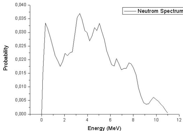
**Figure 5: Probability distribution vs. Energy Bin for the neutron source.**
