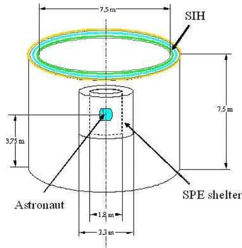
**Figure 1: Vehicle concept: model of the SIH and SPE shelter of the Inflatable Habitat Module.**
