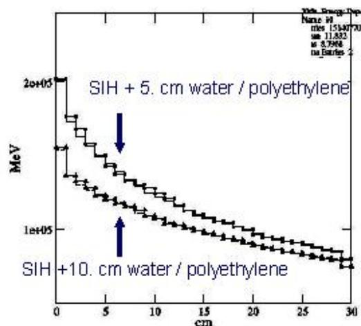
**Figure 6: Energy deposit in the astronaut concept resulting from GCR protons, in the experimental set-up shown in figure 3, in different shielding configurations (indicated by the arrow in the figure); the energy deposit is calculated with respect to the depth in the astronaut concept.**
