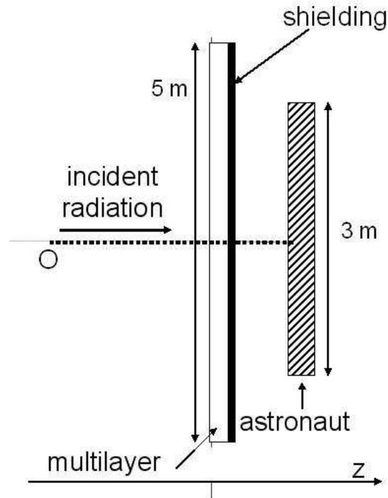
**Figure 3: Geant4 model of the Simplified Inflatable model complemented by a shielding layer; multilayer refers to the SIH structure.**
