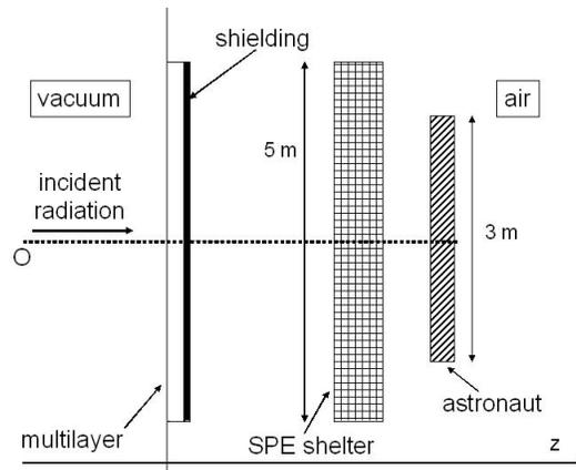
**Figure 4: Geant4 model of the SIH model complemented by a shielding layer and an additional SPE shelter; multilayer refers to the SIH structure.**
