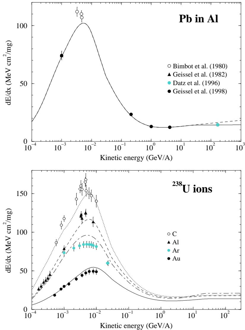
**Figure 4: Calculated (lines) ionization loss vs. experimental data (symbols) for lead ions in aluminum (top) and uranium ions in several targets (bottom) [17]. For lead ions the dashed line indicates calculation for pointlike projectiles.**
