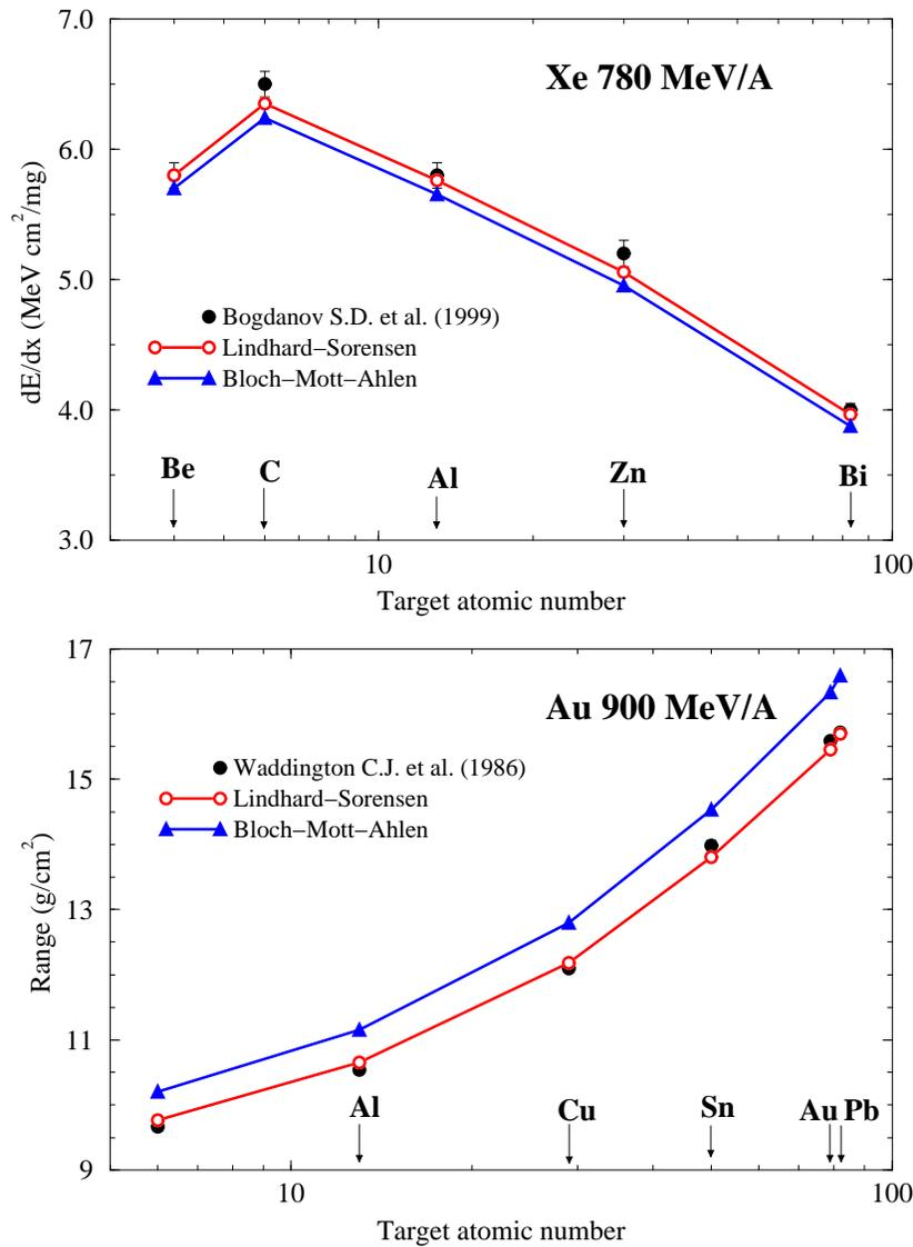
**Figure 3: Calculated (lines with symbols) ionization loss and range of relativistic heavy ions in various targets vs. experimental data (pure symbols) [16]. The corrections to the ionization logarithm,  $\Delta L$ , were calculated following the Lindhard- Sørensen and Bloch-Mott-Ahlen formalisms (see above).**
