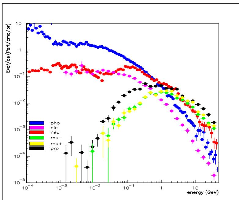
Figure 2. Spectral fluences of different particles as calculated by FLUKA for flight N. 3.
