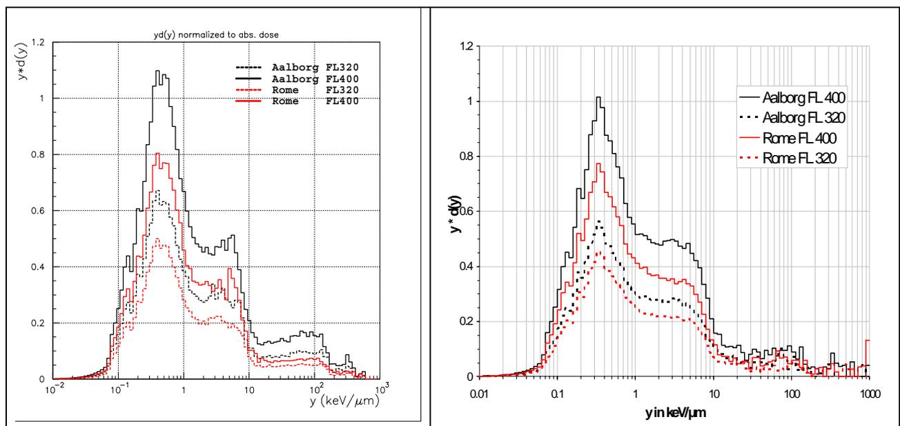
**Figure 4. Microdosimetric spectra distribution  $y \cdot d(y)$  for the 4 considered flights: simulation (left) and measurements (right). The integral of each curve is normalized to the absolute values of the absorbed dose rate.**
