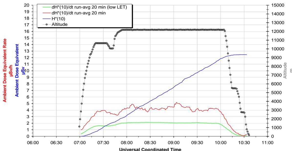
**Figure 1. Flight (3) profile over Rome as a function of time.**
