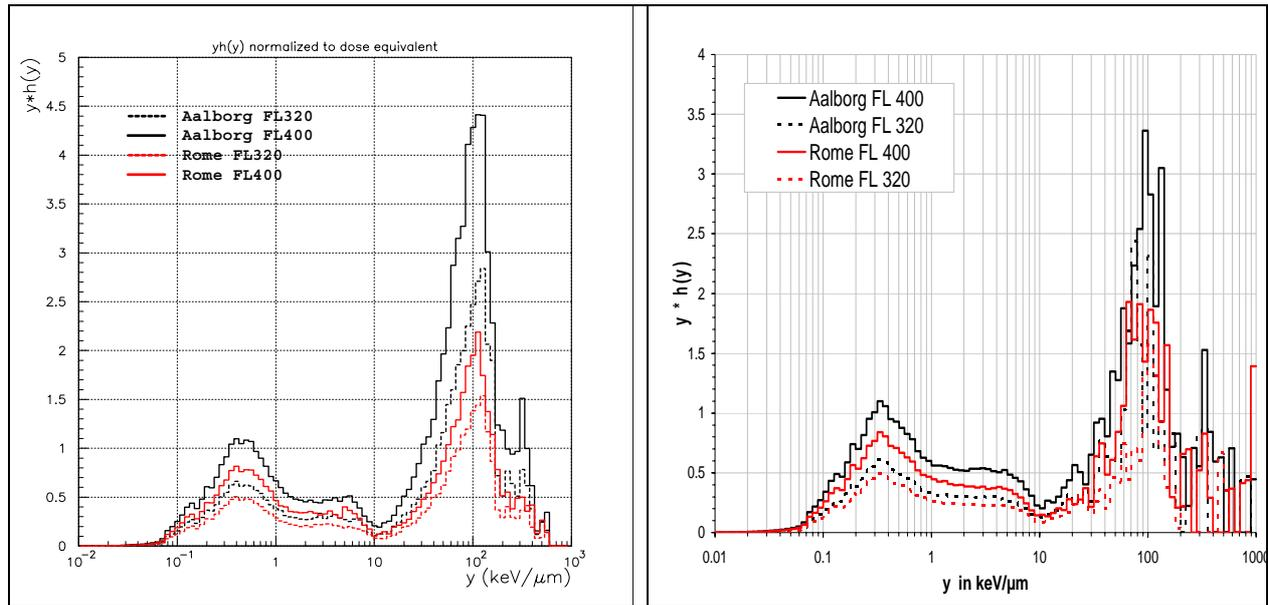
**Figure 5. Microdosimetric spectra distribution  $y \cdot h(y)$  for the 4 considered flights: simulation (left) and measurements (right). The integral of each curve is normalized to the absolute values of the dose equivalent rate.**
