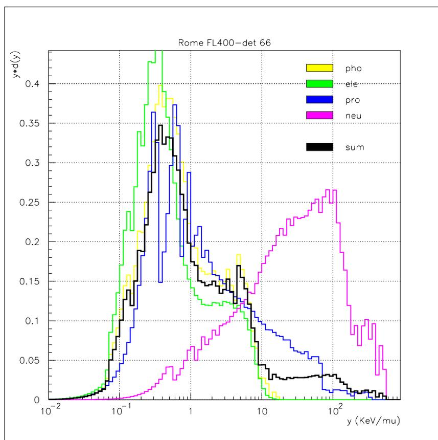
**Figure 3. Microdosimetric spectra  $y \cdot d(y)$  for each particle as seen by the FLUKA simulated TEPC for flight N. 3.**
