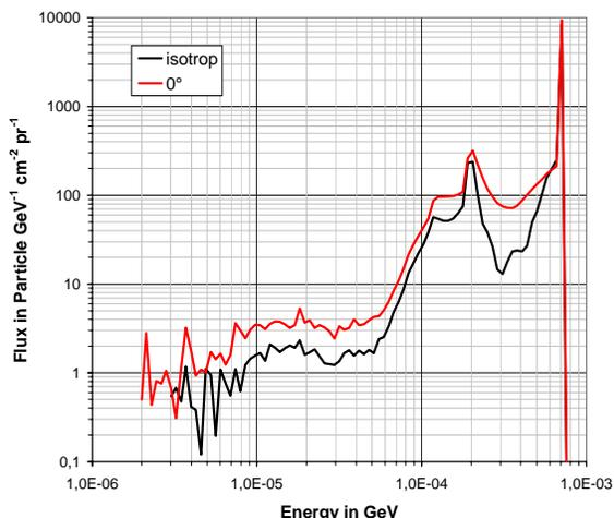
**Figure 5: Photon flux per source particle inside the TEPC for <sup>137</sup>Cs as a function of energy. Comparison of a parallel beam and isotropic field.**
