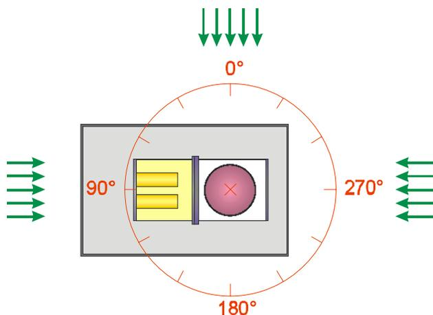
Figure 2: Definition of the beam directions.
