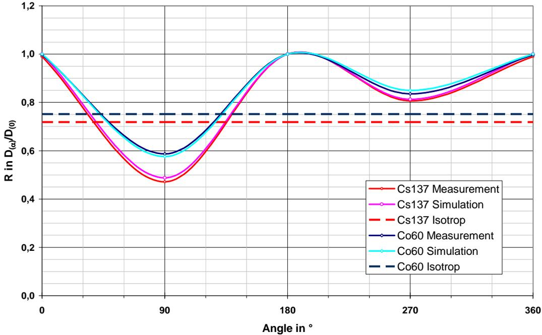
**Figure 4: Relative energy deposition of different neutron source energies as a function of the incoming beam direction. For comparison the values for the isotropic field are added as dashed lines.**
