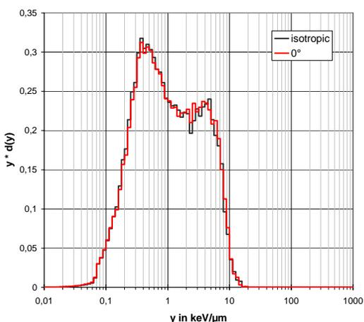
**Figure 7: Comparison of the normalized microdosimetric spectra of parallel beam and isotropic field conditions for a <sup>137</sup>Cs source.**
