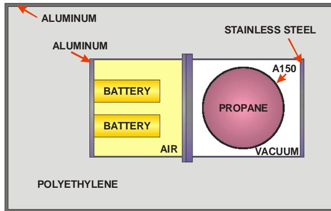
Figure 1: FLUKA simulation geometry.
