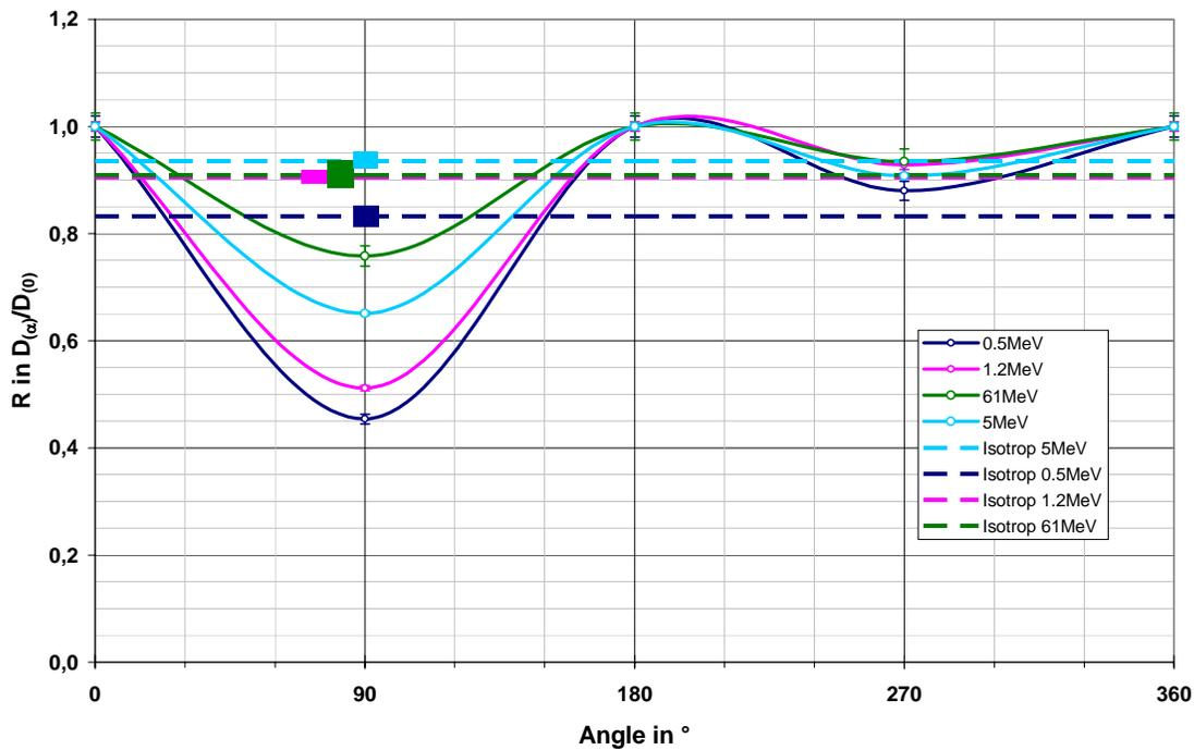
**Figure 9: Relative energy deposition of different neutron source energies as a function of the incoming beam direction. For comparison the values for the isotropic field including their error bars are added as dashed lines.**
