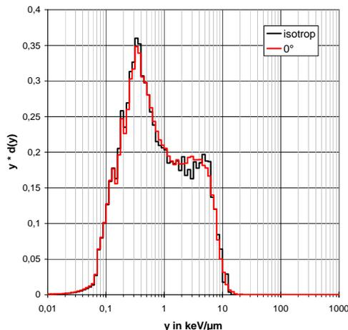
**Figure 8: Comparison of the normalized microdosimetric spectra of parallel beam and isotropic field conditions for a <sup>60</sup>Co source.**
