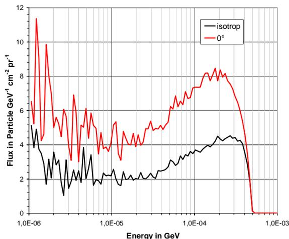
**Figure 6: Electron flux per source particle inside the TEPC for <sup>137</sup>Cs as a function of energy. Comparison of a parallel beam and isotropic field.**
