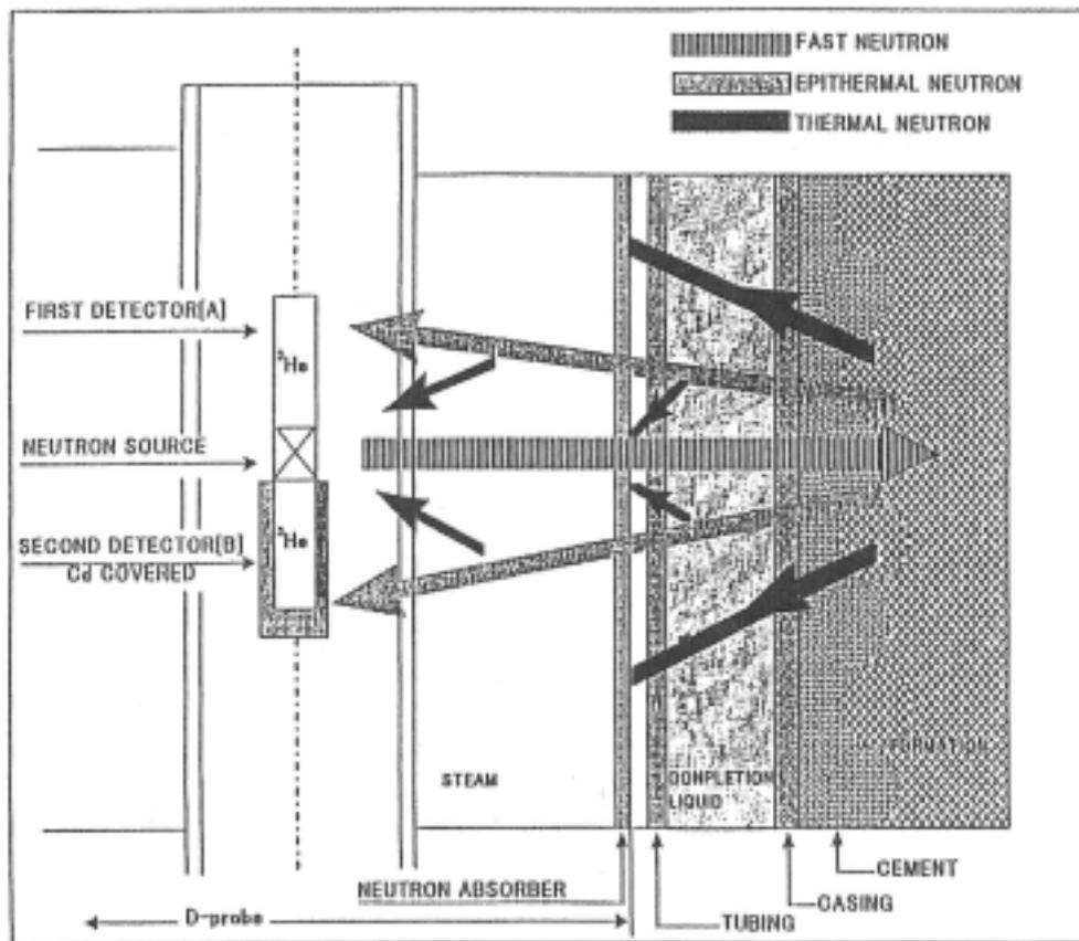
**Figure 2. Behavior of Neutrons Around D-Probe**
