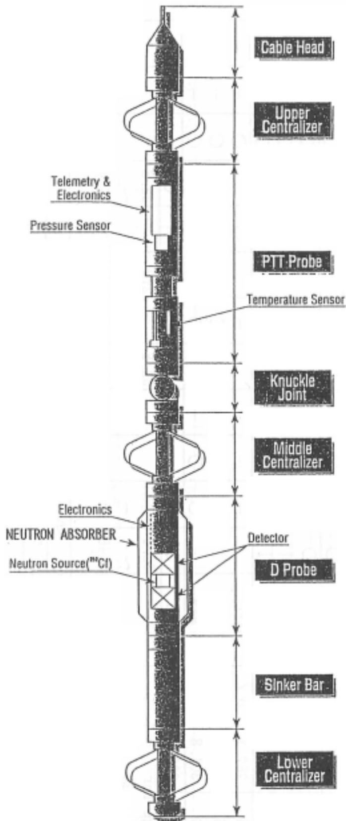
**Figure 1. Configuration of PTD Tool**
