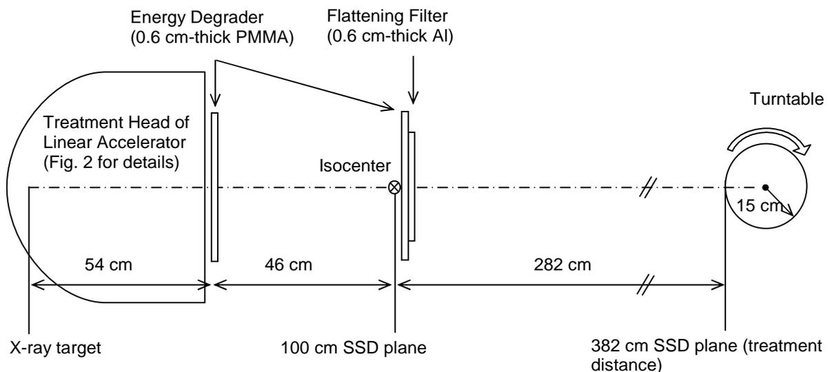
**Figure 1. Schematic diagram of the total skin electron irradiation (TSEI) unit at the University of Alabama at Birmingham. The patient, on a turntable, is treated with a single electron field from a linear accelerator. The energy degrader is located at either of two positions arrowed.**
