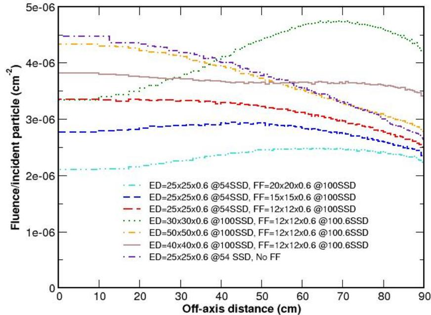
**Figure 3.** Monte Carlo-calculated beam profiles at 382 cm SSD for six sets of PMMA energy degraders and aluminum flattening filters, and for an energy degrader only (i.e., no flattening filter). In legend, ED and FF stand for energy degrader and flattening filter, respectively.
