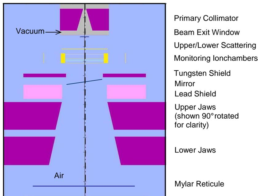
**Figure 2.** Schematic diagram of the accelerator treatment head assumed in Monte Carlo simulations using EGS4/BEAM [11]. The Lower Jaws are turned  $90^\circ$  for clarity.
