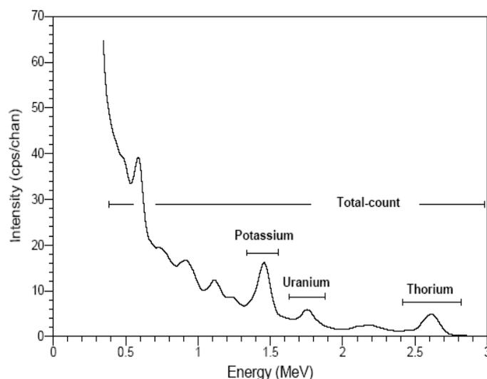
**Figure 2. Typical airborne gamma ray spectrum showing the positions of the conventional energy windows.**
