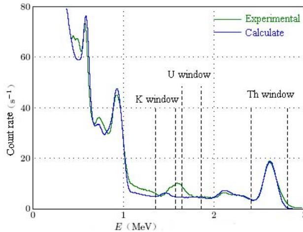
**Figure 8. The simulated and experimental energy response spectrum of detector at 1 m high of Th pad model.**
