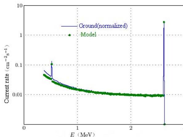
**Figure 7. The spectrum of current rate at 100m altitude of 2.615MeV gamma ray from pad and infinite homogenous ground sources.**
