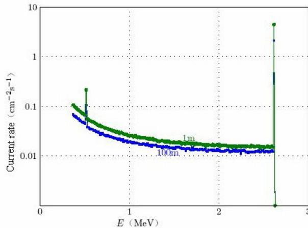
Figure 4. The current rates spectrum of 2.615Mev source at 1m and 100m altitude
