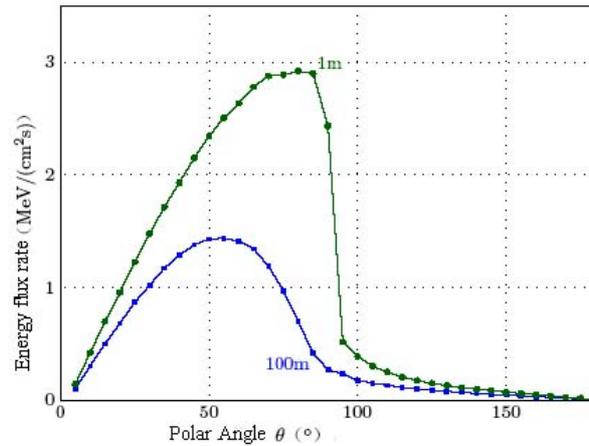
**Figure 5. Comparison of angle spectrum of energy flux rates of 2.615 MeV source at 1m and 100m altitude**
