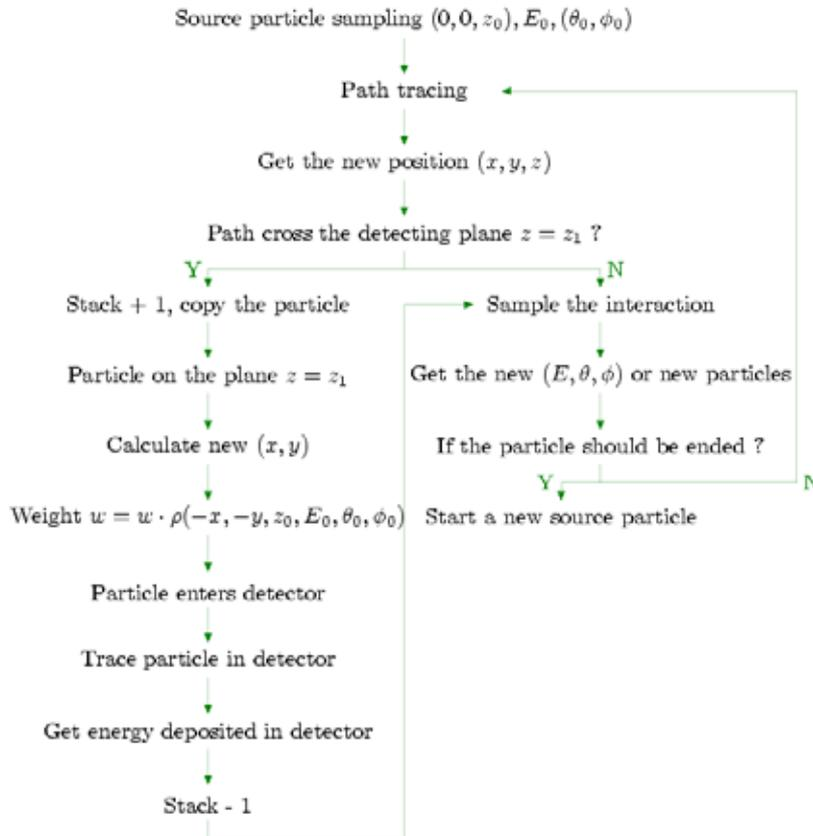
Figure 3. Flowchart of geometrical equivalent Monte Carlo simulation
