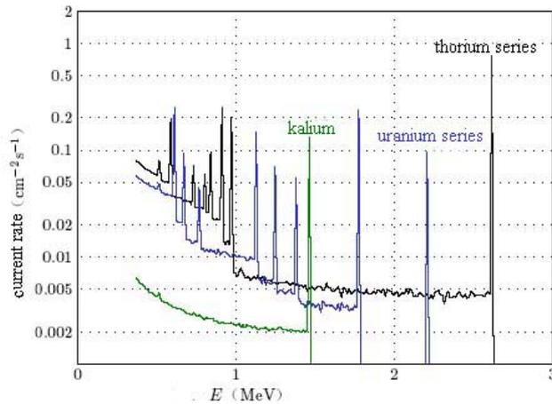
**Figure 6. The spectrum of current rate of infinite uniform ground source at 100m altitude.**
