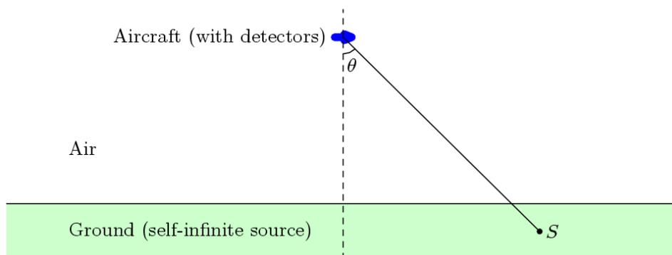
Figure 1. The schematic diagram of airborne gamma ray spectrometry system.
