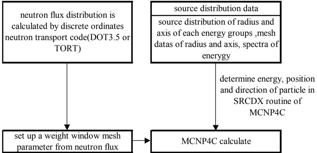
Figure 2. Flow chart of the MCNP4C calculation used weight window mesh parameter.
