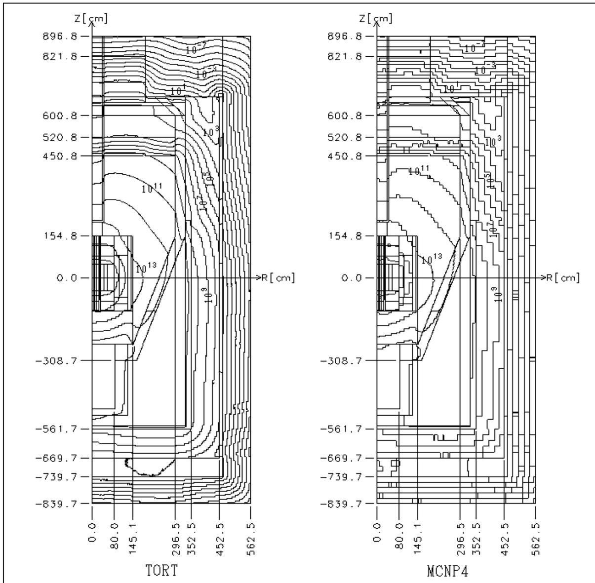
Figure 3. Contour of total neutron flux distribution
