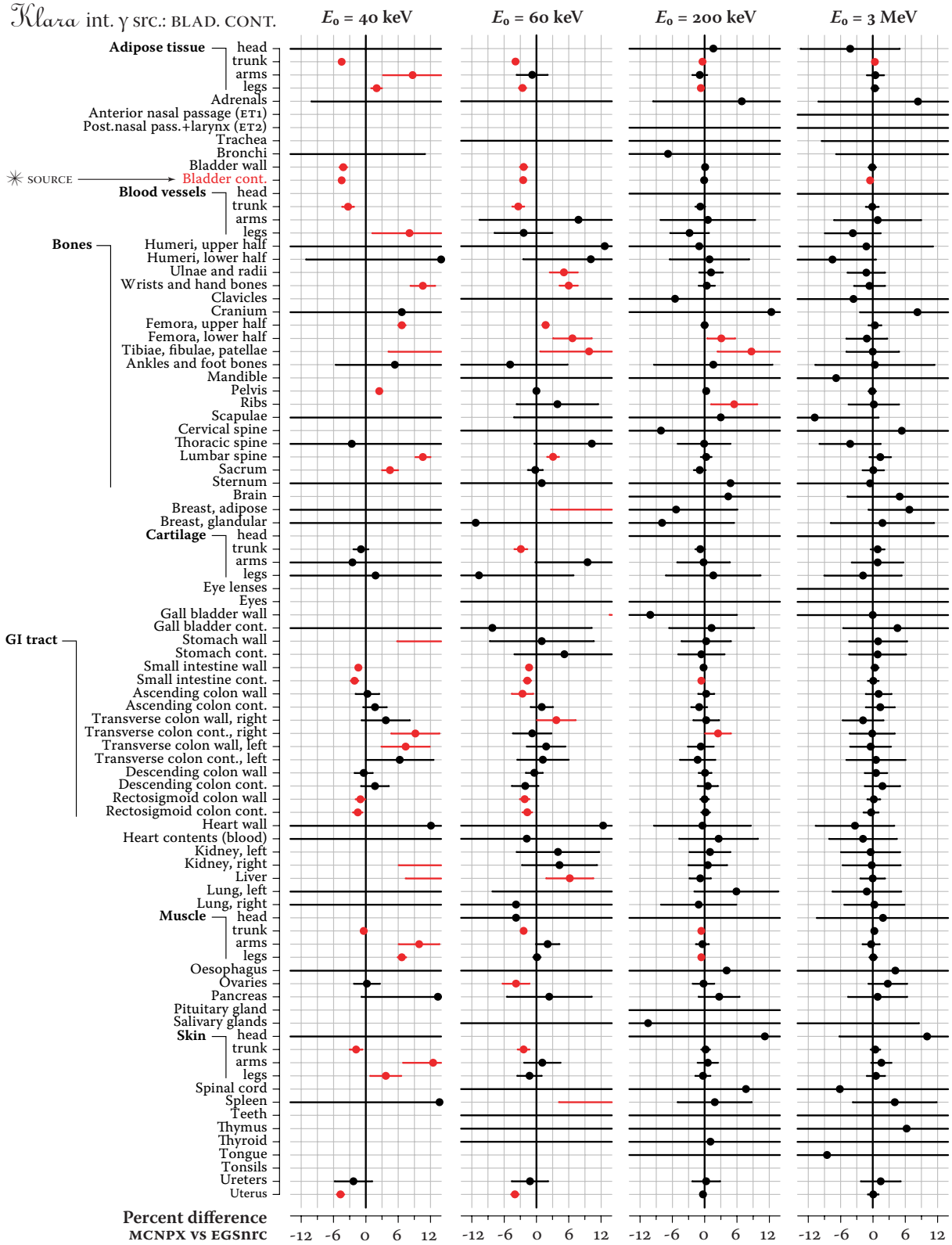
Figure 6. Comparison of organ doses calculated with MCNPX and EGSnrc for bladder content as internal photon source in the female phantom Klara . The EGSnrc results were taken as reference. Two sigma uncertainties are shown as lines. Cases of statistically significant discrepancy are shown in red.
