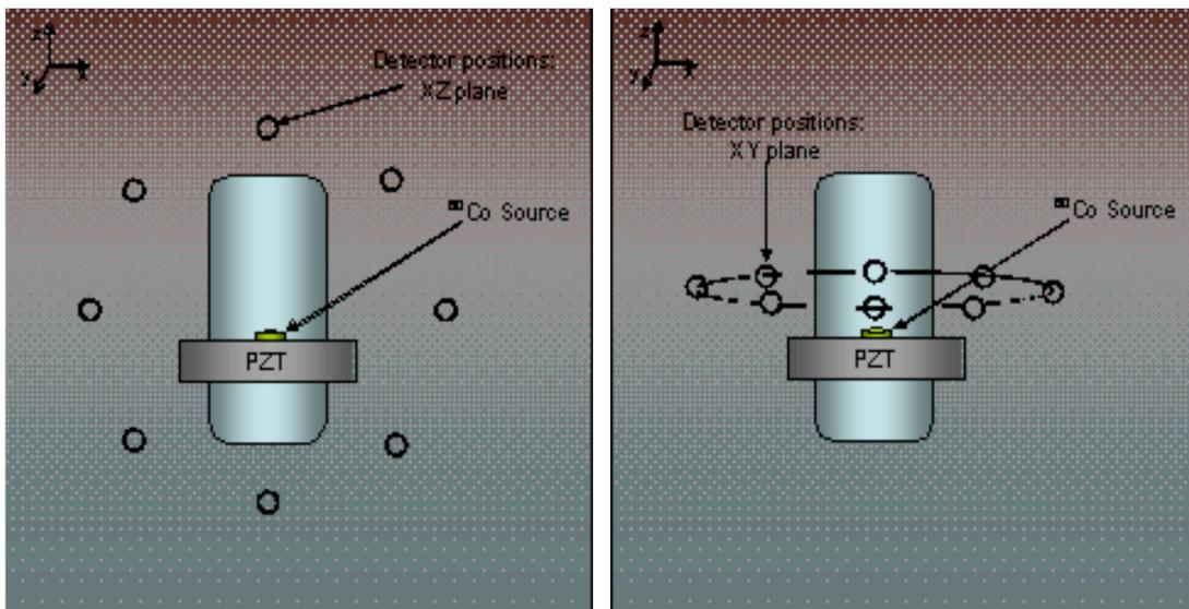
Figure 4. Detector locations for the XZ and XY planes
