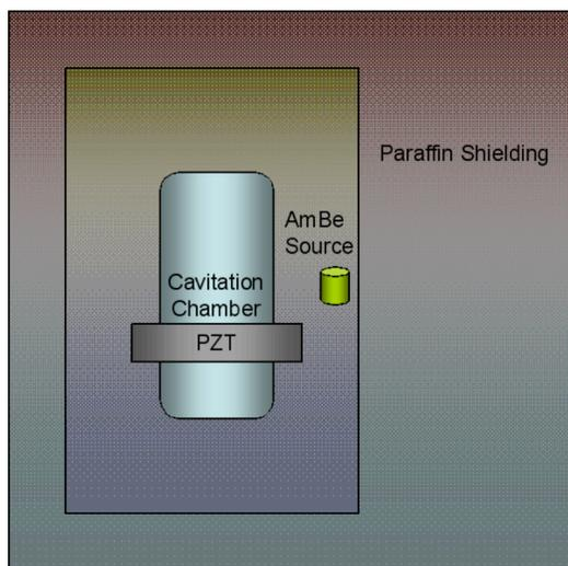
**Figure 1. Diagram of a simplified cavitation chamber, source, and paraffin shielding**
