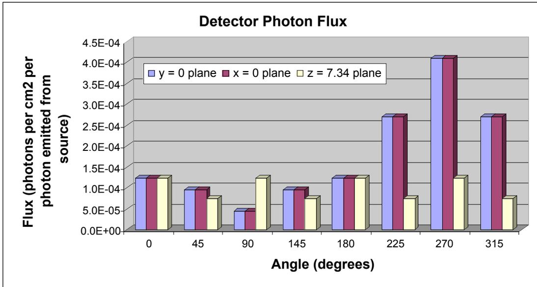
Figure 5. Relative detector flux of 662 keV gammas from  $^{60}\text{Co}$  source
