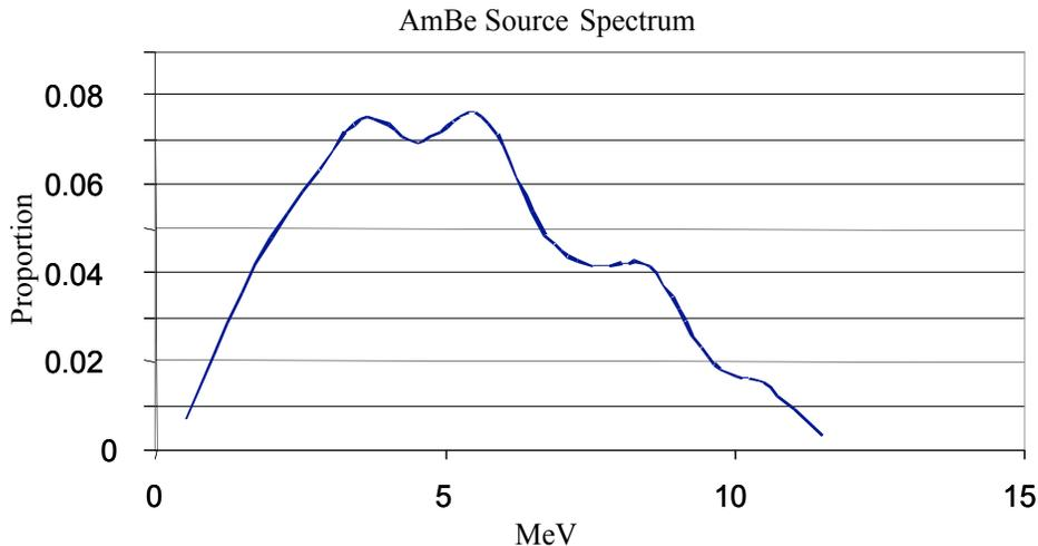
Figure 3. Neutron energy spectrum from AmBe source
