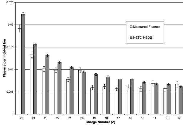
**Figure 1: Fragment Fluence Due to 1050 MeV per Nucleon <sup>56</sup>Fe on 3.5 g/cm<sup>2</sup> of Graphite**
