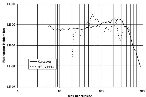
**Figure 6: Neutron Fluence Measured at 7.5-Degrees Due to 400 MeV per Nucleon  $^{12}\text{C}$  on  $35.4 \text{ g/cm}^2$  of Graphite**
