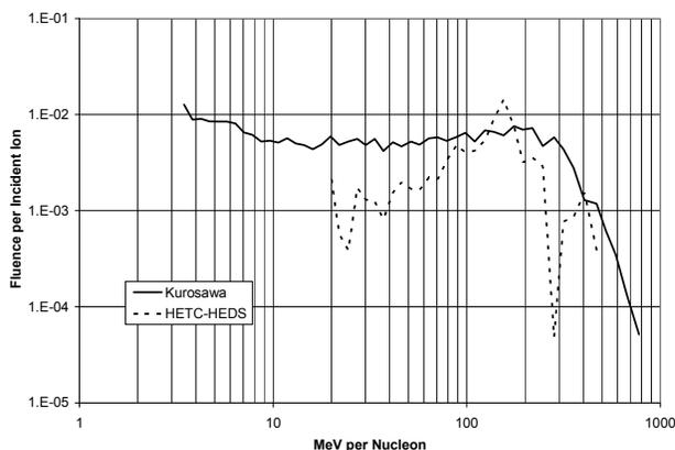
**Figure 7: Neutron Fluence Measured at 15-Degrees Due to 400 MeV per Nucleon  $^{12}\text{C}$  on  $35.4 \text{ g/cm}^2$  of Graphite**
