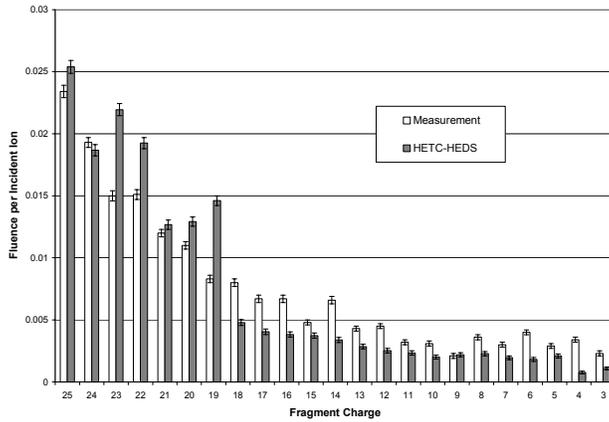
**Figure 4: Fragment Fluence Due to 1050 MeV per Nucleon  $^{56}\text{Fe}$  on  $1.94 \text{ g/cm}^2$  of Polyethylene**
