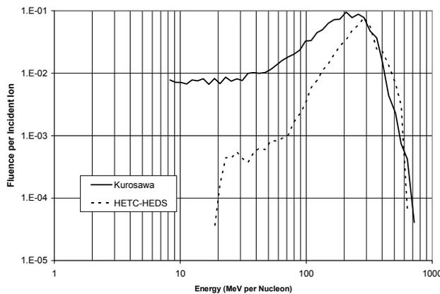
**Figure 5: Neutron Fluence Measured at 0-Degrees Due to 400 MeV per Nucleon  $^{12}\text{C}$  on  $35.4 \text{ g/cm}^2$  of Graphite**
