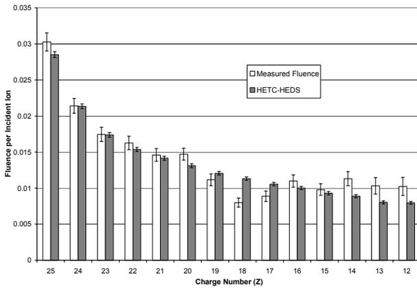
**Figure 2: Fragment Fluence Due to 1050 MeV per Nucleon <sup>56</sup>Fe on 5 g/cm<sup>2</sup> of Graphite and Epoxy**
