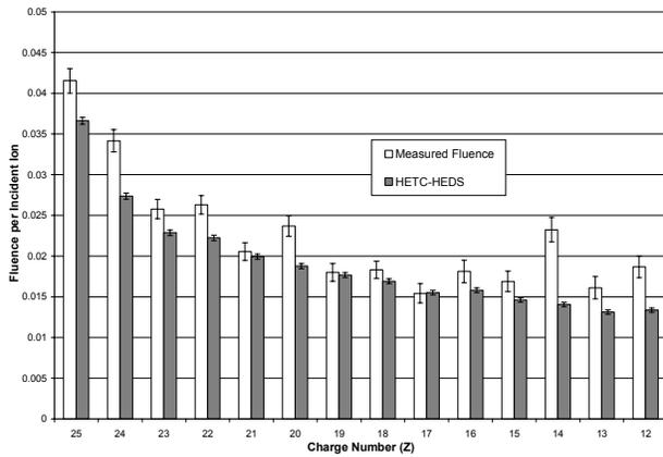
**Figure 3: Fragment Fluence Due to 1050 MeV per Nucleon <sup>56</sup>Fe on 10 g/cm<sup>2</sup> of Graphite and Epoxy**
