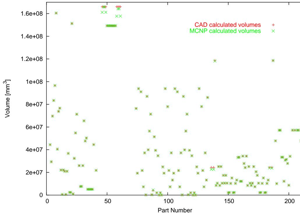
**Figure 4: Volumes of parts calculated by MCNP and CAD system.**
