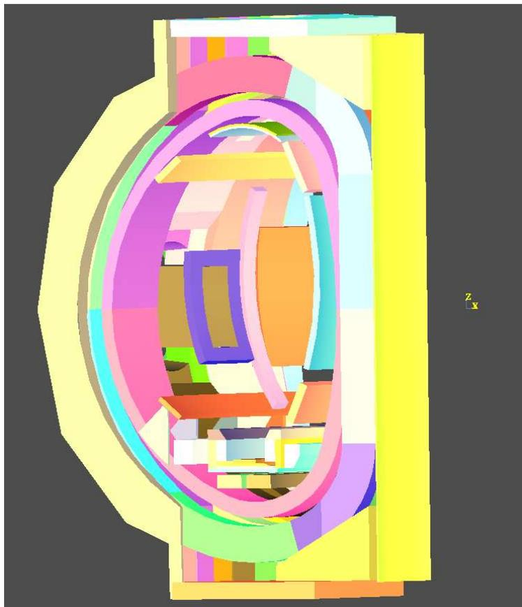
**Figure 2: CAD model of the JET torus sector.**
