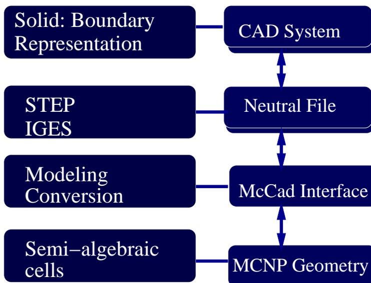
**Figure 1: Outline of the method used for CAD Interface for MCNP.**
