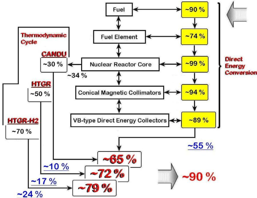
Figure 3. Energy conversion efficiency of the FFMCR system.
