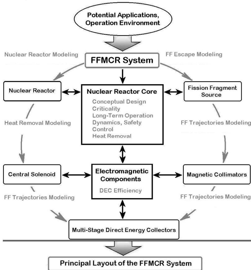
**Figure 2. Computational modeling of the FFMCR system.**
