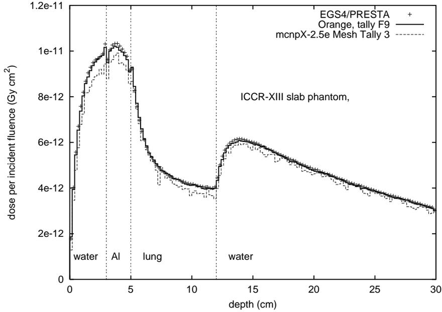
**Figure 1: Results for the dose per incident fluence for the ICCR-XIII benchmark phantom, calculated by Orange, mcnpX, and EGS4.**
