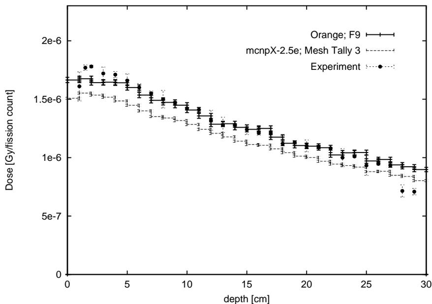
**Figure 2: Results for the dose per fission count for the high energy neutron beam experiment, as calculated by Orange, and mcnpX.**
