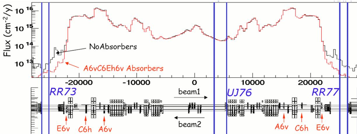
**Figure 6: All particle fluence in the IR7 tunnel versus the longitudinal distance. The effect of the additional absorbers is visible in the cold sections.**
