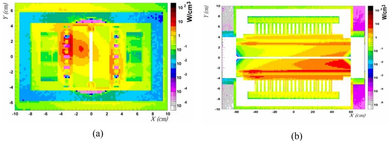
**Figure 5: Energy deposition on the secondary collimator. It is visible the hotspot from the cascade at about 1cm from the center, due to the effect of the magnetic field of the MBW and the rotation of the collimator.**
