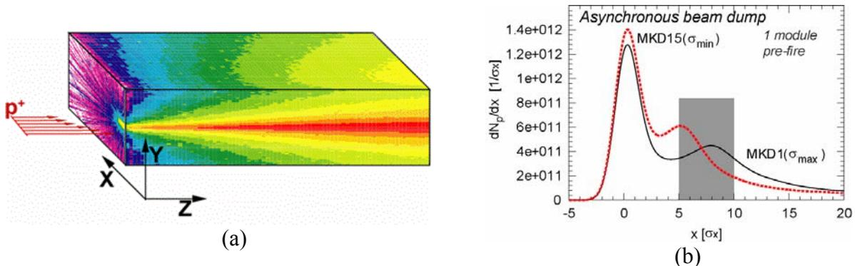
**Figure 1: (a) Simulated geometry of a single collimator jaw; (b) beam profile impacting the horizontal face of the collimator jaw.**
