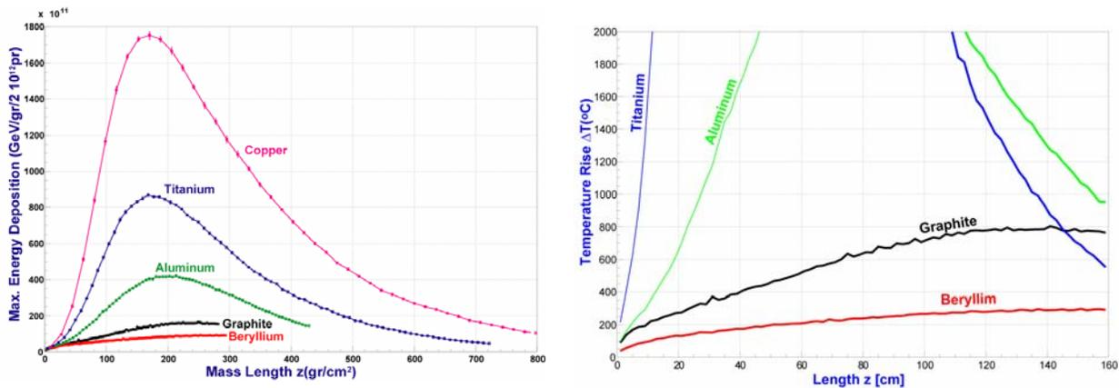
**Figure 2. (a) Trace of the maximum energy deposition on a collimator jaw per mass-length, and (b) maximum instantaneous temperature for the wrong kick scenario at 7 TeV/c.**
