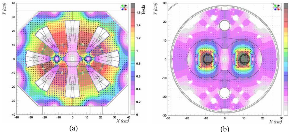
**Figure 4: Cross section of geometry and magnetic field map of (a) warm quadrupole (MQW) and (b) superconducting bending magnet (MB)**
