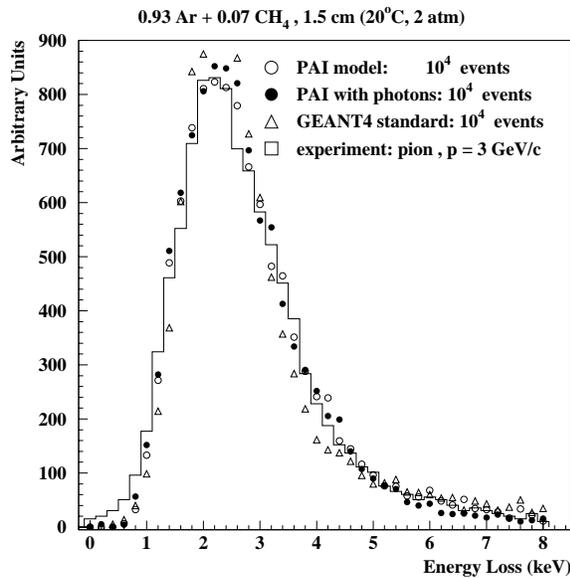
Figure 3. Geant4 simulation of the drift chamber filled with Ar/CH<sub>4</sub>: histogram – data [11], points – simulation.
