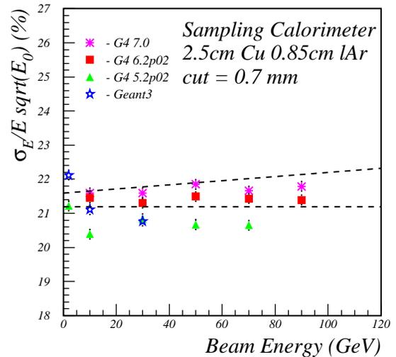
Figure 2. Energy resolution in the sampling calorimeter as a function of beam energy: dashed lines show  $1\sigma$  road of the data [4].
