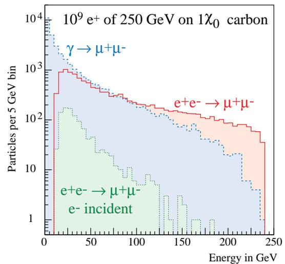
**Figure 12.** Muon energy spectrum in the beam pipe of 250 GeV linear collider. After a carbon collimator of one radiation length thick.
