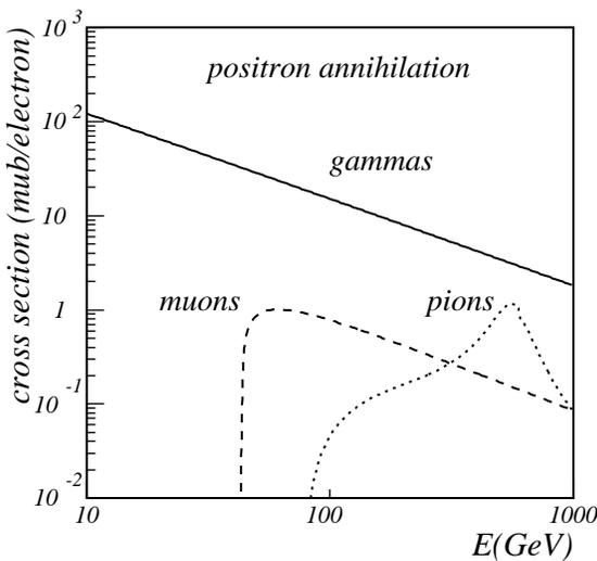
**Figure 11.** Cross sections per media electron of positron annihilation.
