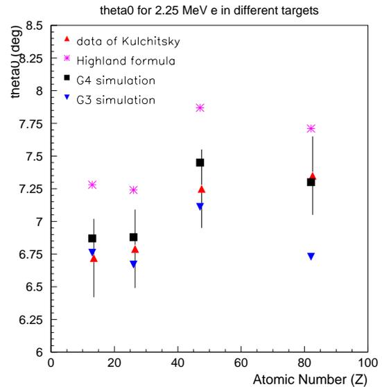
Figure 6. Multiple scattering for low energy electrons in different targets: simulations, Highland formula predictions, and the data [18].
