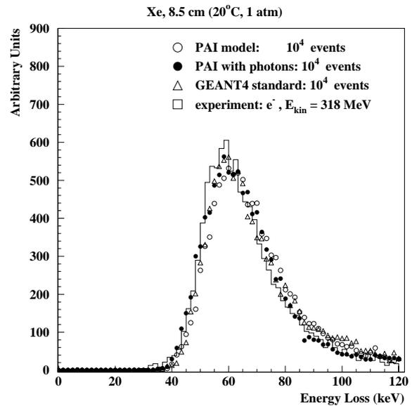
Figure 4. Geant4 simulation of the drift chamber filled by Xe: histogram – data [12], points – simulation.
