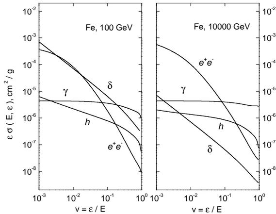
**Figure 9. Differential cross section for muon interaction processes in iron.**
