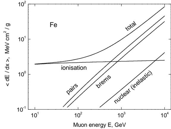
**Figure 10. Average energy loss of muons in iron.**
