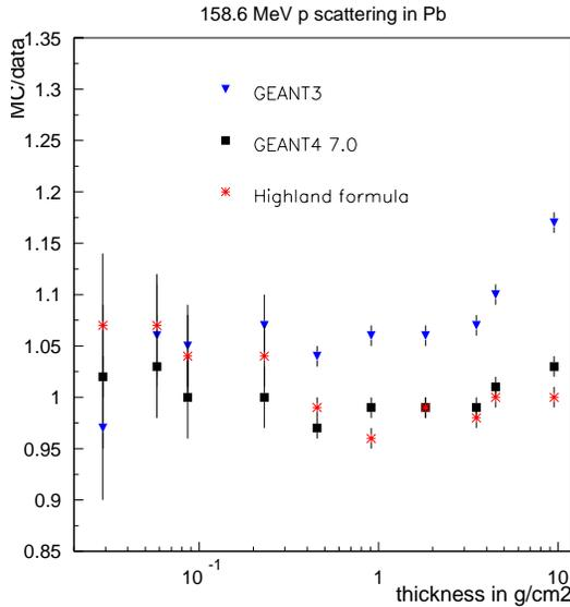
**Figure 7. Multiple scattering of 158.6 MeV protons in thin lead foil as a function of the thickness. Simulation angle is divided by the data angle [19].**
