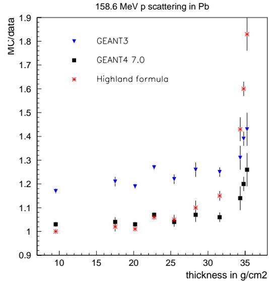
**Figure 8. Multiple scattering of 158.6 MeV protons in thick lead foil as a function of the thickness. Simulation angle is divided by the data angle [19].**
