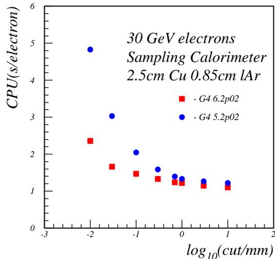
Figure 1. CPU for 2.4 GHz 512 kB PC Linux as a function of cut in range. The same value of the cut is used for gamma, electrons, and positrons.
