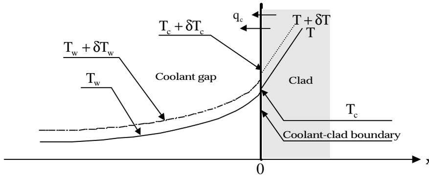
Figure 1. Coolant-clad boundary calculation scheme.
