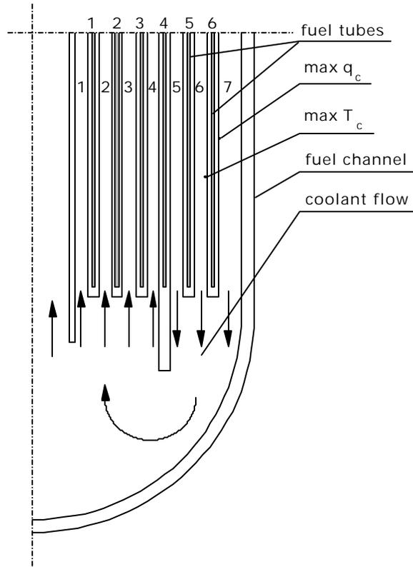
Figure 3. Schematic diagram of coolant flow through the fuel channel in MARIA reactor.
