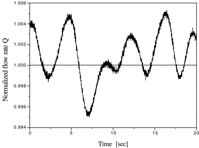
Figure 5. Time record of coolant flow fluctuations in MARIA reactor.
