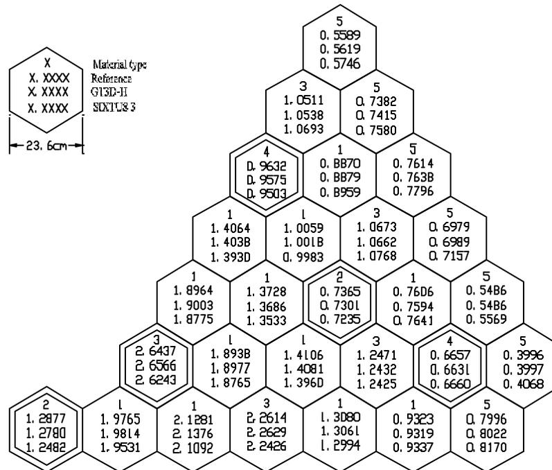
Figure 2. Radial power density distribution on lower core of the WWER-1000 problem.
