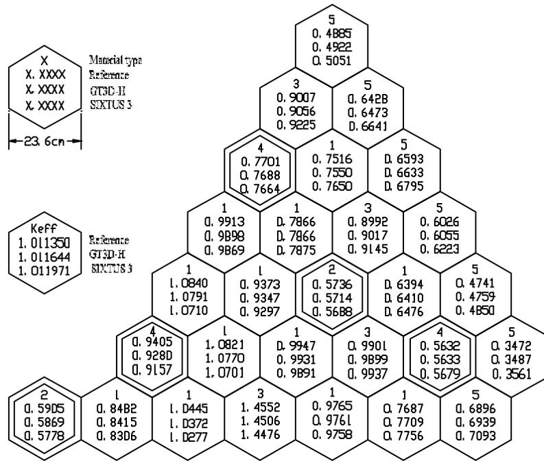
Figure 1. Radial power density distribution on upper core of the WWER-1000 problem.
