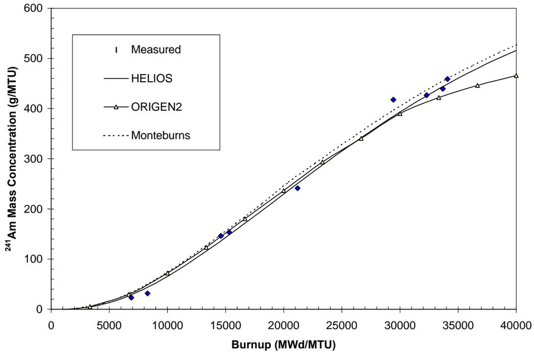
Fig. 1.  $^{241}\text{Am}$  concentration versus burnup for a Mihama Unit 3 fuel pin (calculated and measured).
