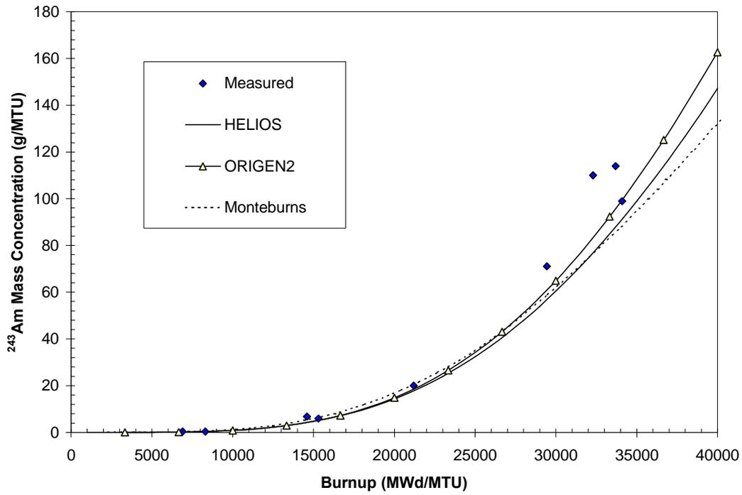
Fig. 2.  $^{243}\text{Am}$  concentration versus burnup for a Mihama Unit 3 fuel pin (calculated and measured).
