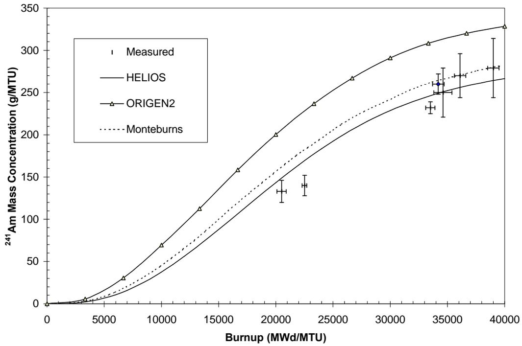
Fig. 3.  $^{241}\text{Am}$  concentration versus burnup for a VVER-440 fuel pin (calculated and measured).
