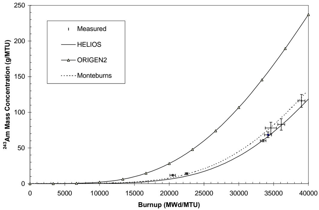
Fig. 4.  $^{243}\text{Am}$  concentration versus burnup for a VVER-440 fuel pin (calculated and measured).
