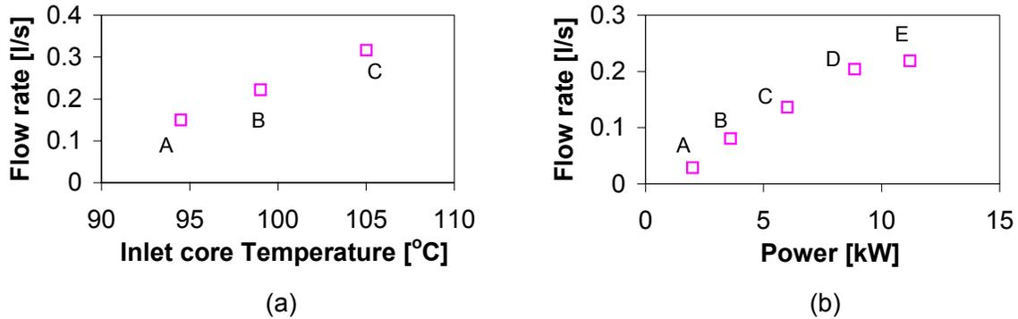
**Figure 4:** Flow rate as a function of the controlled variable in the performed two series of measurements. The flow rate increases both for decreasing subcooling at constant power (a) and for increasing power at constant subcooling (b).
