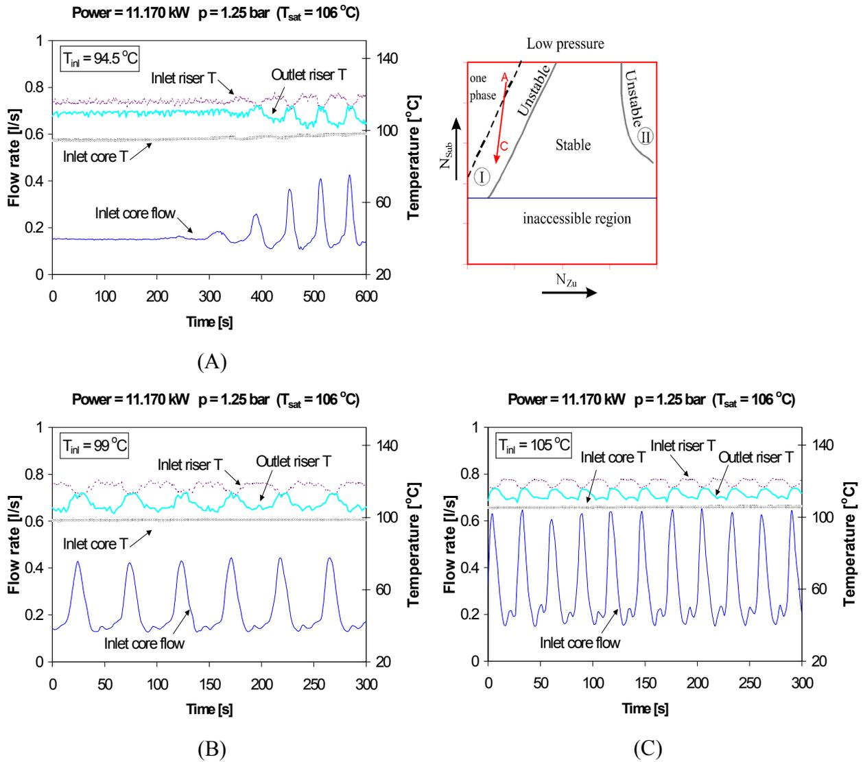
**Figure 5:** Time traces recorded at constant power and decreasing subcooling. At the top right the path followed on the stability map passing from case A to C is shown.
