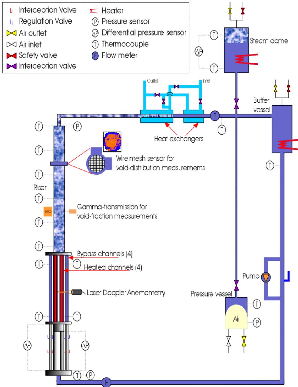
**Figure 1:** Scheme of the CIRCUS facility (not to scale). The main instrumentation is also shown.
