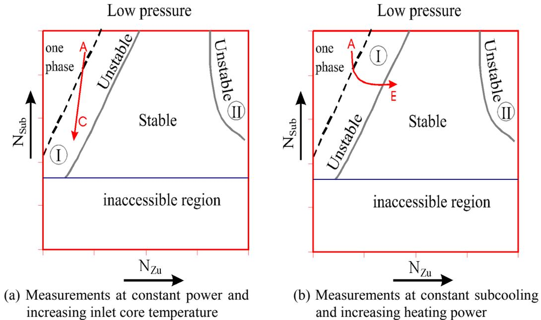
**Figure 3:** Indicative path (red) followed on the stability map in the first (a) and in the second (b) series of measurements, performed at constant power and at constant subcooling, respectively. In both cases the measurement started from the stable one-phase flow region.
