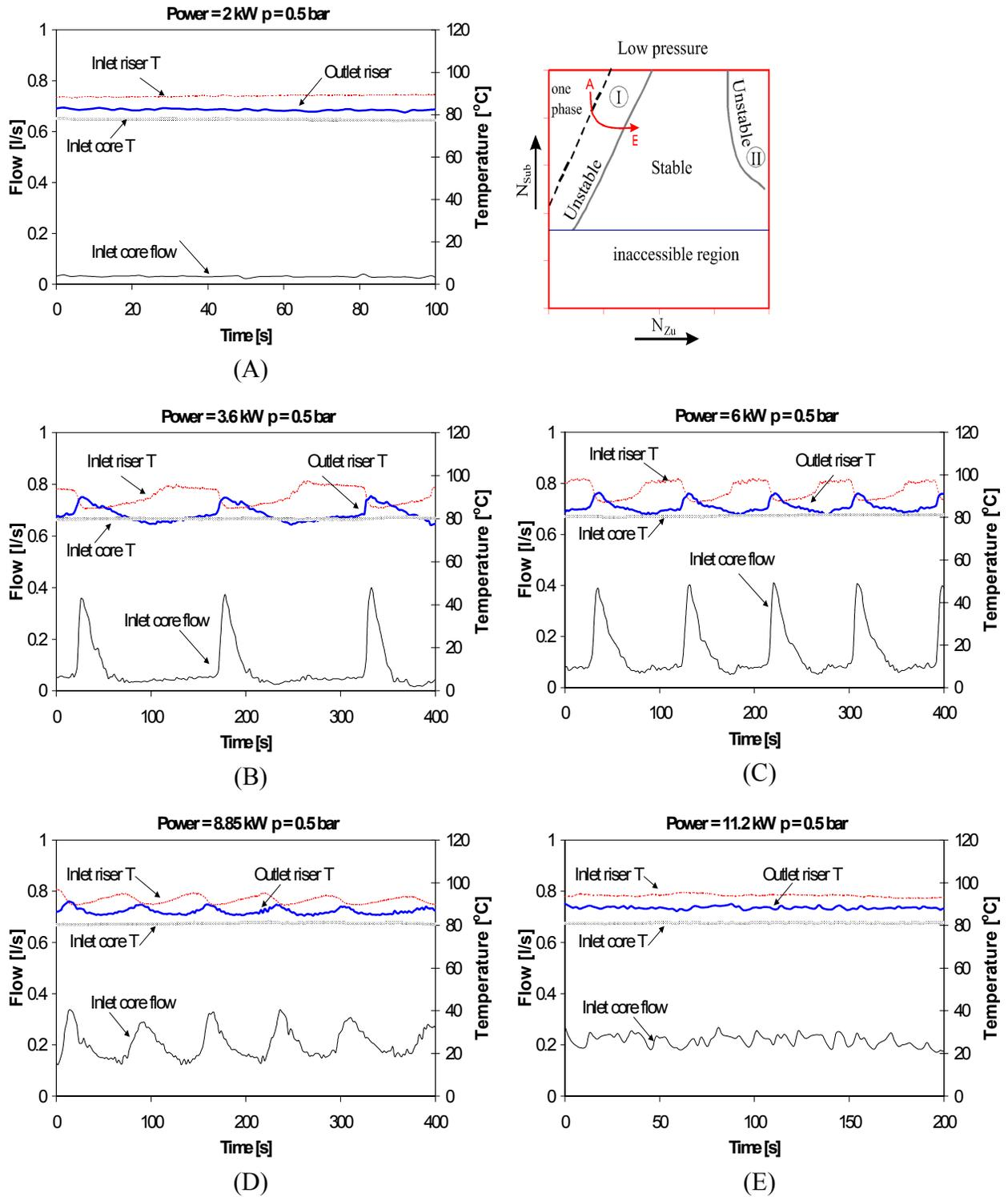
**Figure 6:** Time traces recorded at constant subcooling and increasing power level. At the top right the path followed on the stability map passing from case A to E is shown.
