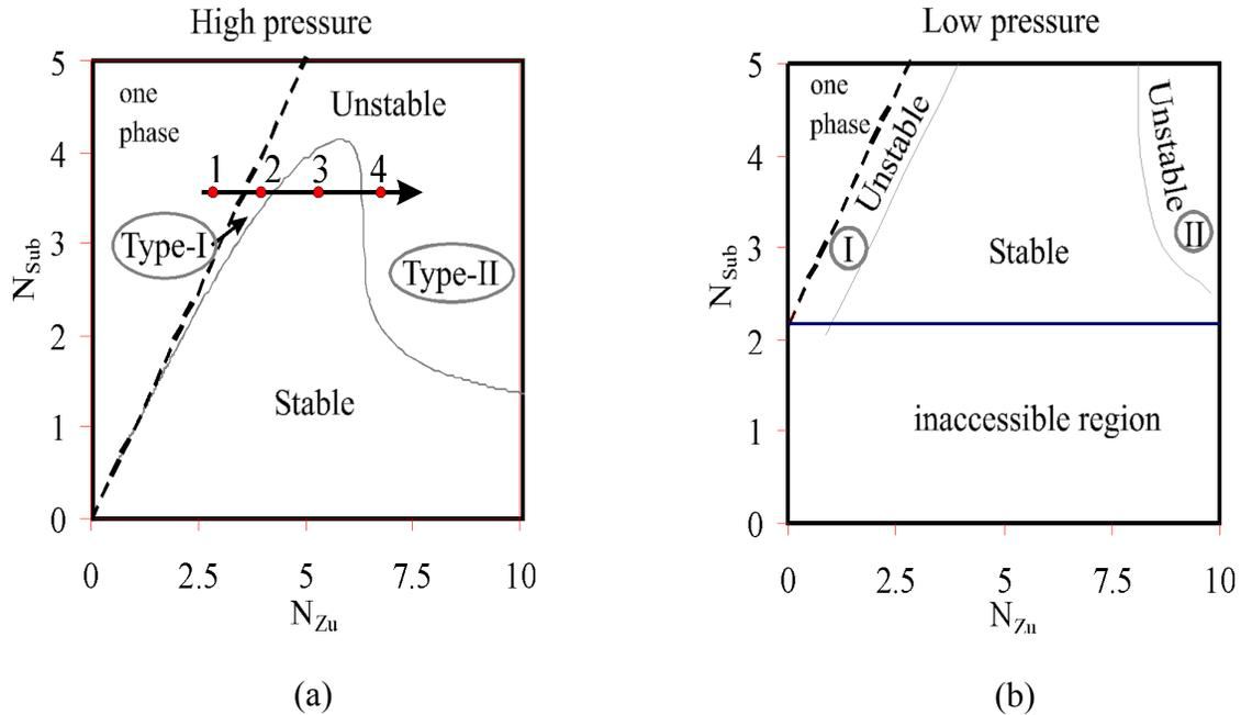
**Figure 2:** Dimensionless stability maps for a thermalhydraulic natural circulation system without (a) and with (b) flashing.
