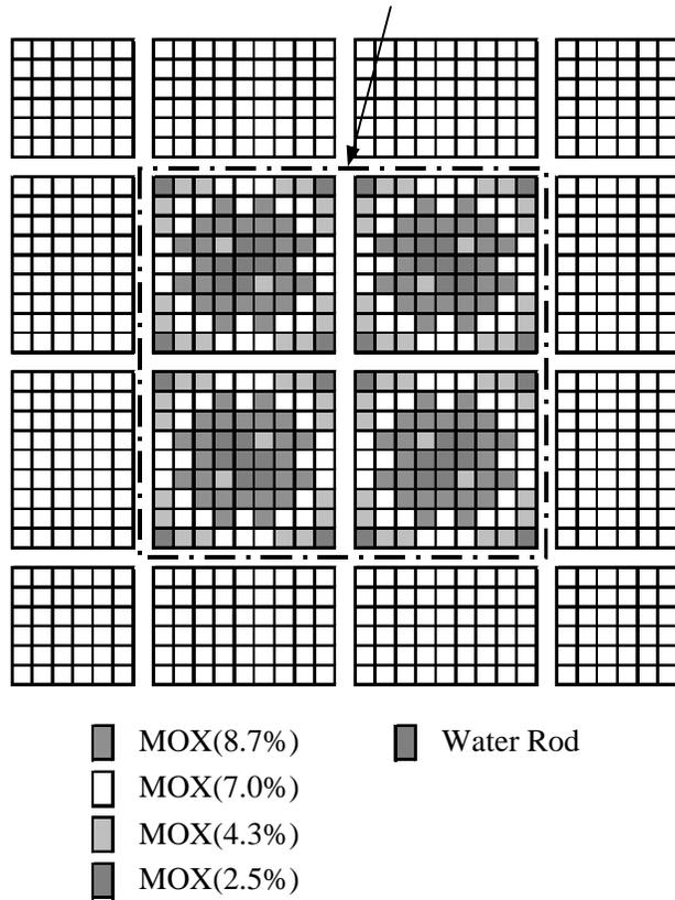
Figure 6. Core Configuration of Reference Core in BWR-Cold
