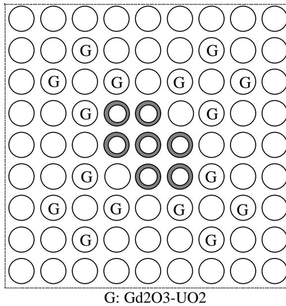
Figure 4. Location of Gd<sub>2</sub>O<sub>3</sub>-UO<sub>2</sub> Fuel Rods
