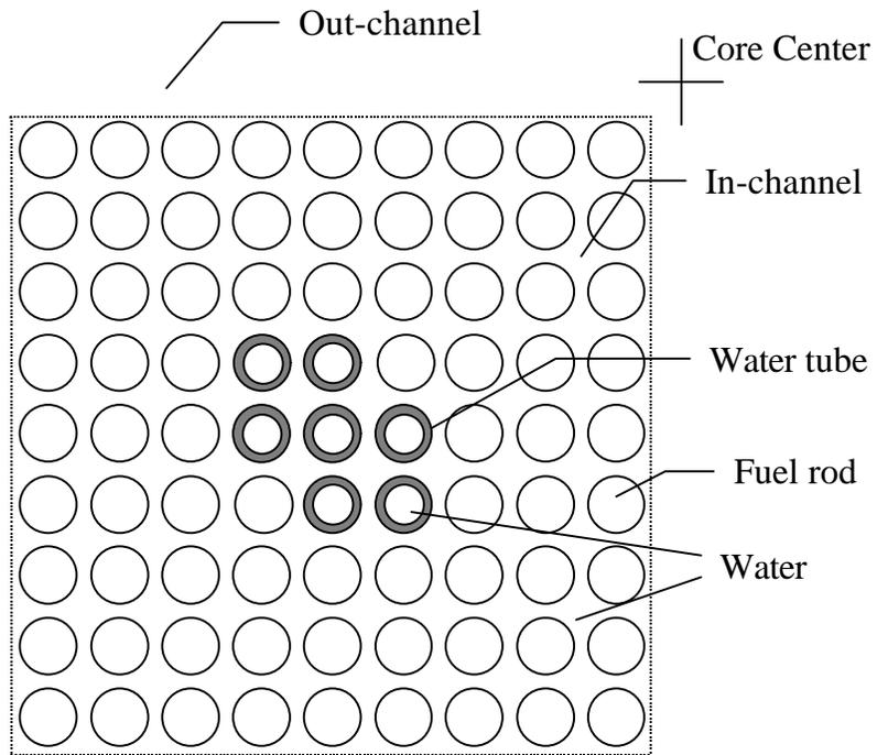
Figure 3. Configuration of Fuel Assembly in Experiments
