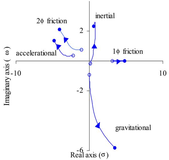
Figure 5b. The locus of the complex vectors of the different pressure drop transfer functions at operating conditions along the dynamic (Type-II) SB.
