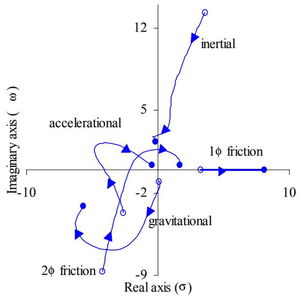
Figure 6b. The locus of the pressure drop transfer functions along the SB of the natural circulation thermalhydraulic subsystem. The arrows show the direction of moving from the Type-II to the Type-I SB.
