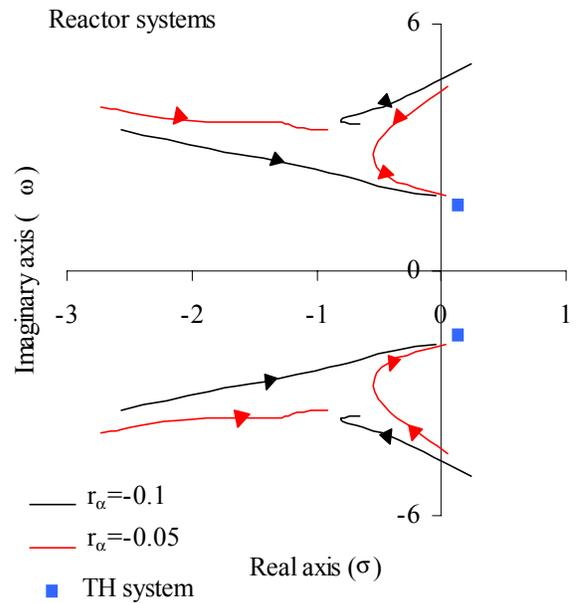
Figure 8b. Poles of the reactor systems along the same trajectory of operating points for two different void reactivity feedback coefficients.
