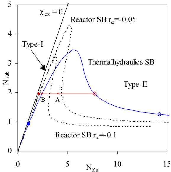
Figure 6a. The SB of the thermalhydraulic subsystem of Dodewaard (blue solid line) and SB's of coupled reactor systems with different void coefficients (dashed lines).
