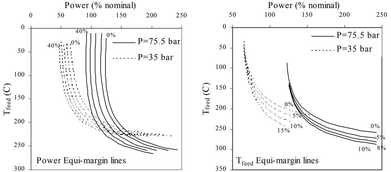
Figure 3. The power stability margins lines (0%, 10%, 20%, 30%, 40% lines from right to left, left figure) and the feedwater temperature margin lines (right figure) change with the system pressure. The curves are shown in the Power –  $T_{\text{feed}}$  plane.
