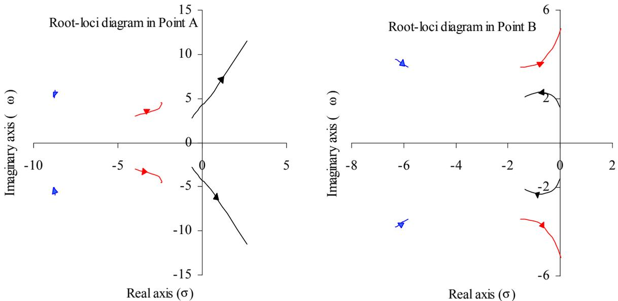
Figure 7. Root-loci diagram of a natural circulation reactor using the void coefficient as parameter. The Type-II oscillations are destabilized in point A in figure 6a (left figure), while in point B the Type-I oscillations are stabilized (right figure) by increasing void feedback. Arrows indicate the direction of increasing void coefficient (only the complex conjugate pole pairs are shown).
