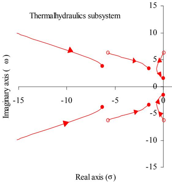
Figure 8a. Poles of the natural circulation thermalhydraulics subsystem as moving along the red trajectory in figure 6a from the Type-II to the Type-I region.
