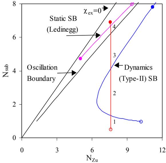
Figure 4a. Dynamic and static SB's of a forced circulation two-phase flow channel.
