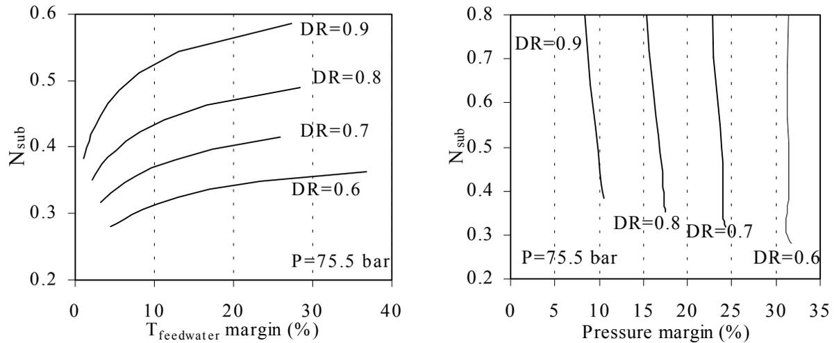
Figure 2. Operational stability margins in terms of the feedwater temperature (left figure) and the system pressure (right figure) along different equi-DR lines.
