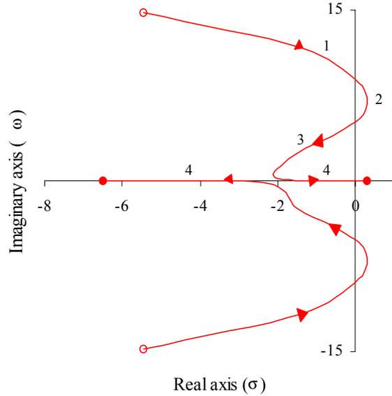
Figure 4b. The complex conjugate pole pair of the system along the red trajectory of operating points in figure 4a. The third, real, pole of the system is not depicted being irrelevant for the stability.
