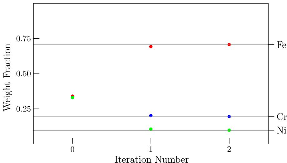
Figure 1: Convergence of the fixed point iteration to the composition of a stainless steel. Red points are Fe fraction, blue are Cr, and green are Ni; the grey lines represent the correct composition of the sample.
