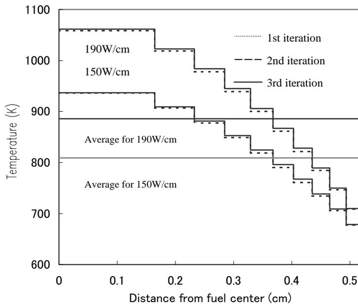
Fig.4 Temperature distribution within a UO<sub>2</sub> fuel
