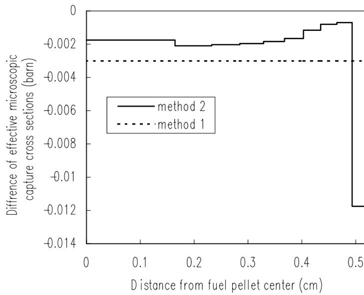
Fig.7 Difference of  $^{238}\text{U}$  capture cross sections between 0.5sec and 1.0sec
