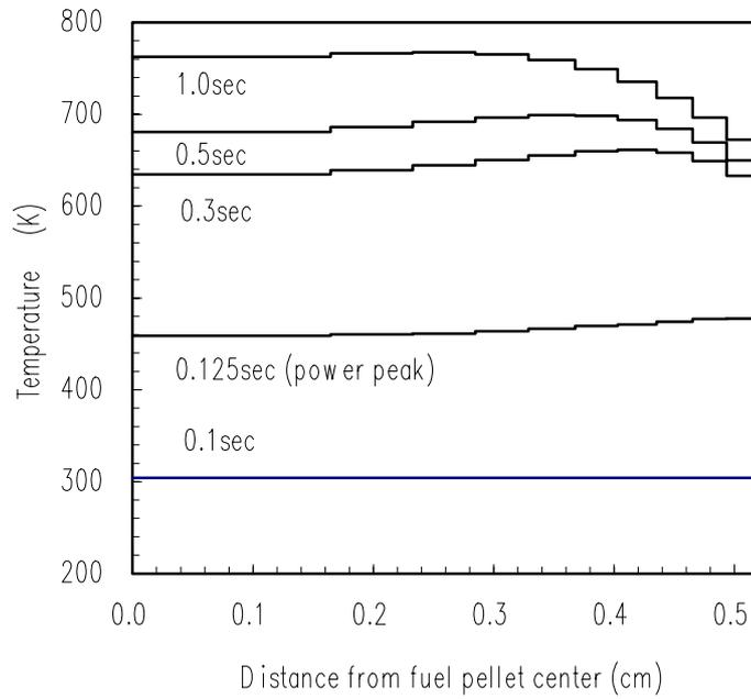
Fig.6 Temperature distribution in fuel pellet at each time step
