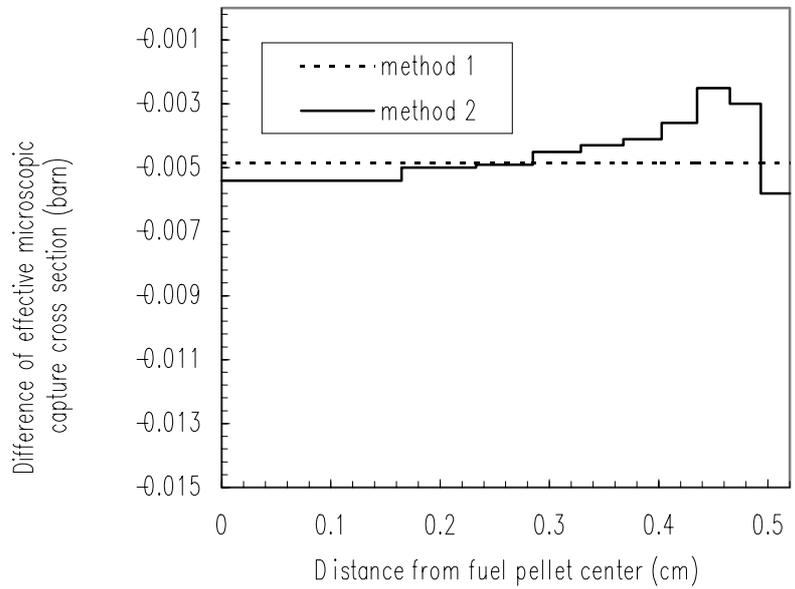
Fig.3 Difference between  $^{238}\text{U}$  capture cross sections for linear heat-generation rates for 150 and 190 W/cm
