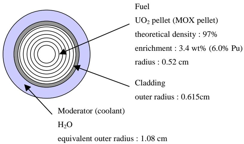
Fig.1 Calculational geometry
