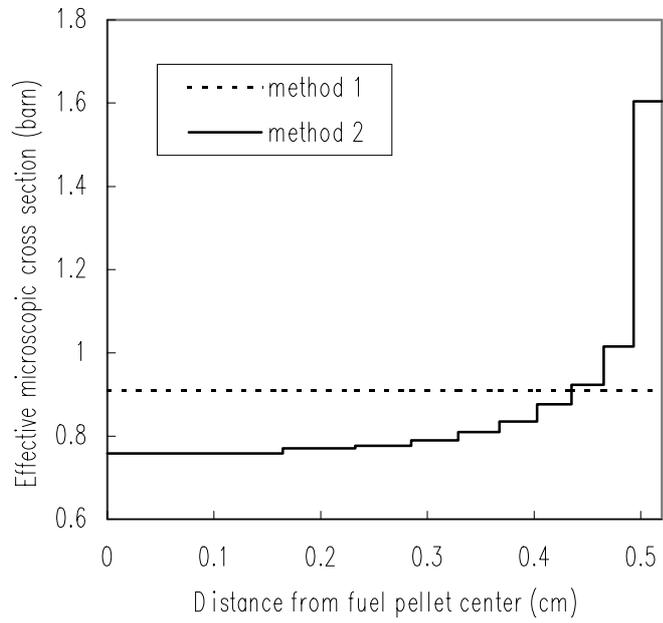
Fig.2 Space dependent  $^{238}\text{U}$  capture cross sections in fuel pellet
