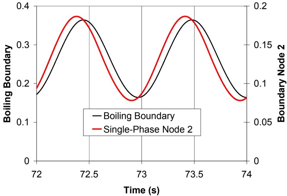
Figure 2. Dimensionless boiling boundary and single-phase boundary of node 2 (both normalized to core length) during limit cycle oscillation.
