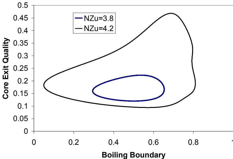
Figure 4. Limit cycle oscillations shown in the boiling boundary - core exit quality parameter space. As the Zuber number increases no sign of period doubling is observed.
