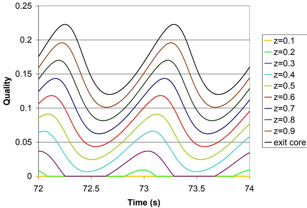
Figure 3. Quality at different axial positions during limit cycle oscillation. The quality increases with the axial position. The line for  $z=0.1$  coincides with the x-axis.
