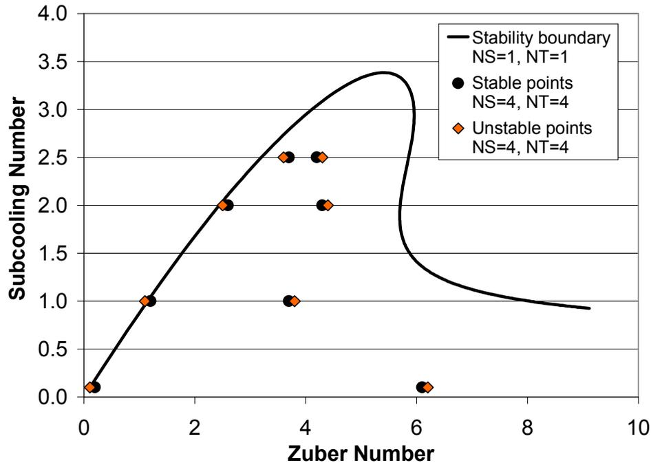
Figure 1. Marginal stability boundary of the boiling channel with riser determined with one node in the single-phase region (NS=1) and one node in the two-phase region (NT=1) compared with stable and unstable operating points according to the model with 4 nodes in both regions.
