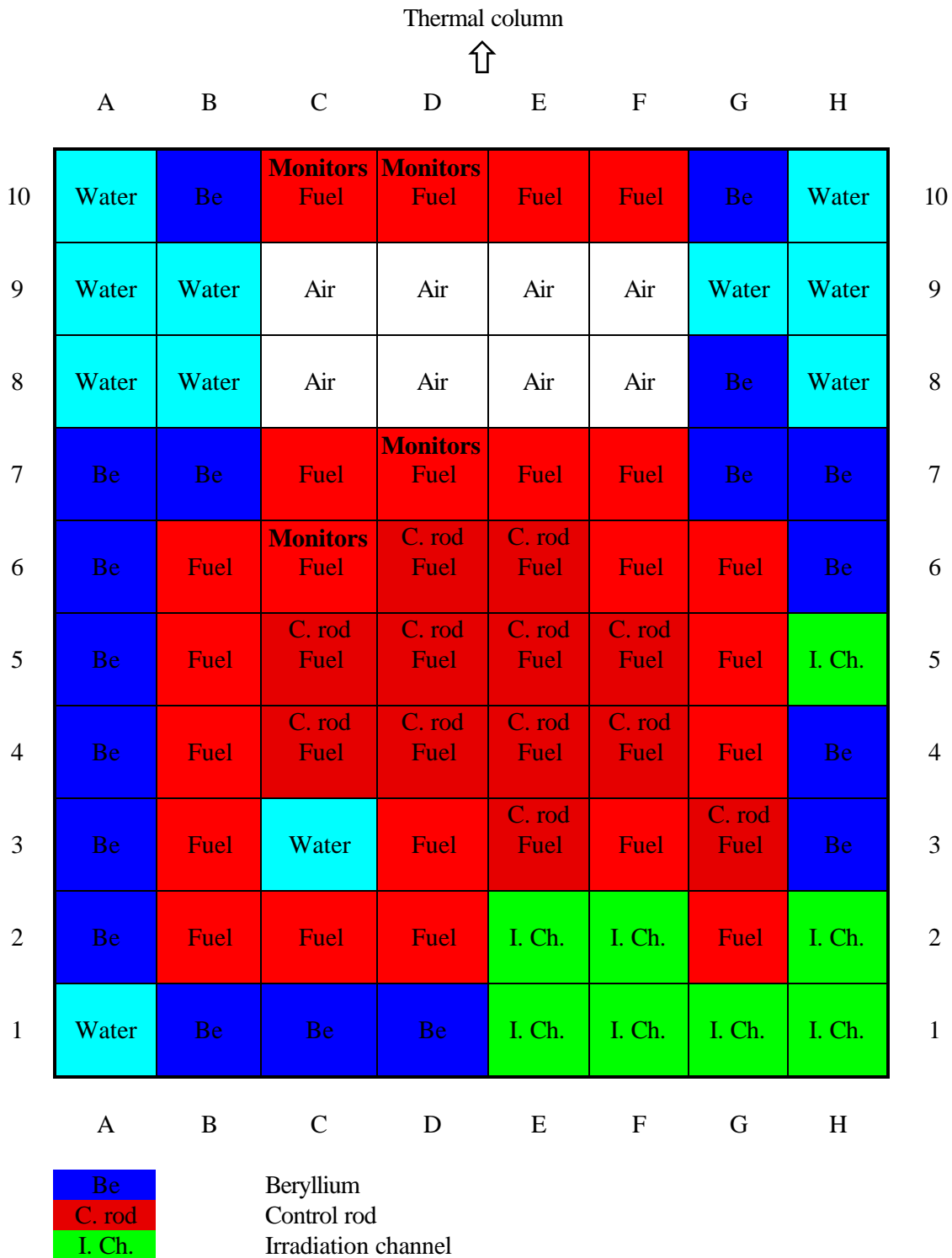
Figure 1. LVR-15 reactor core on 24. June 1999.
