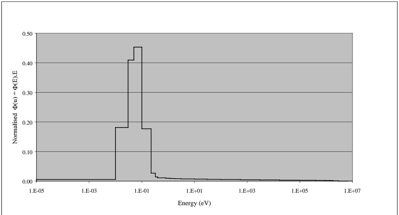
Figure 3. Energetic distribution of the neutron flux in Graphite B
