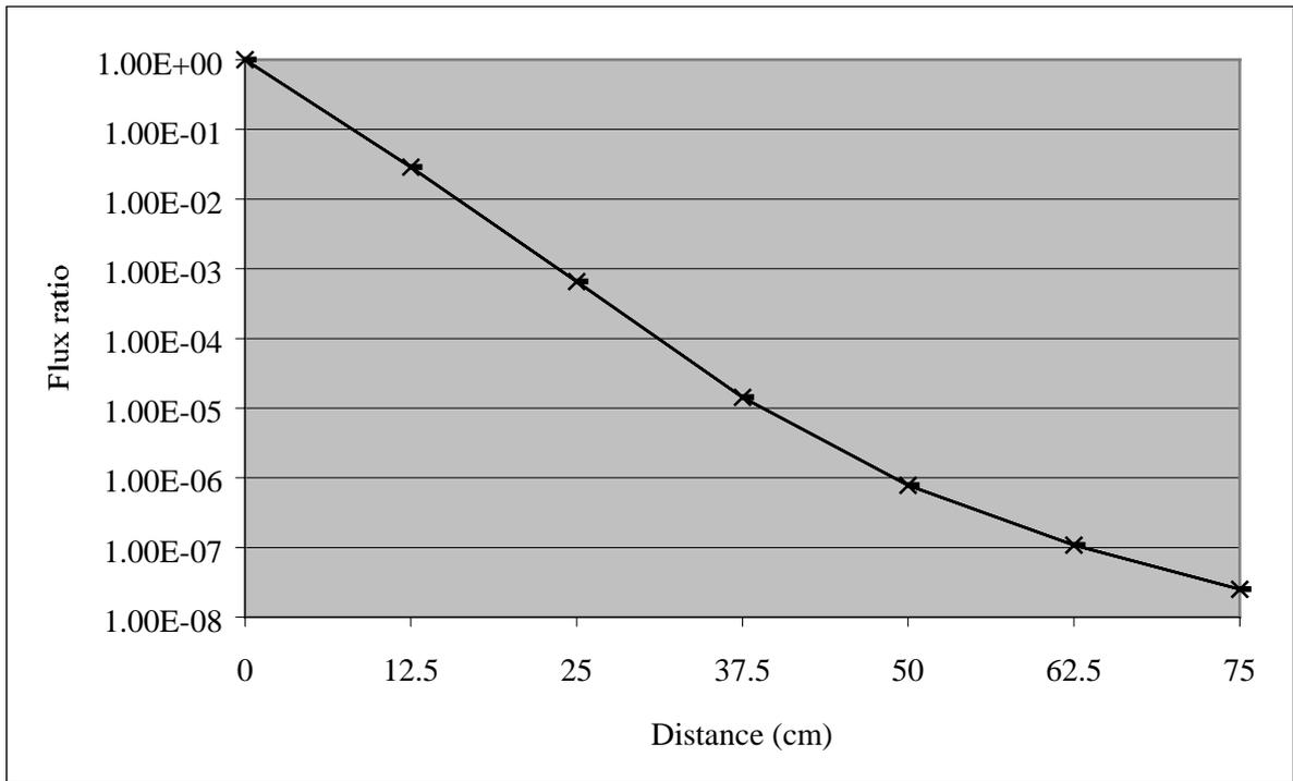
Figure 9. Flux depression in Concrete ( $\psi=45^\circ$ )
