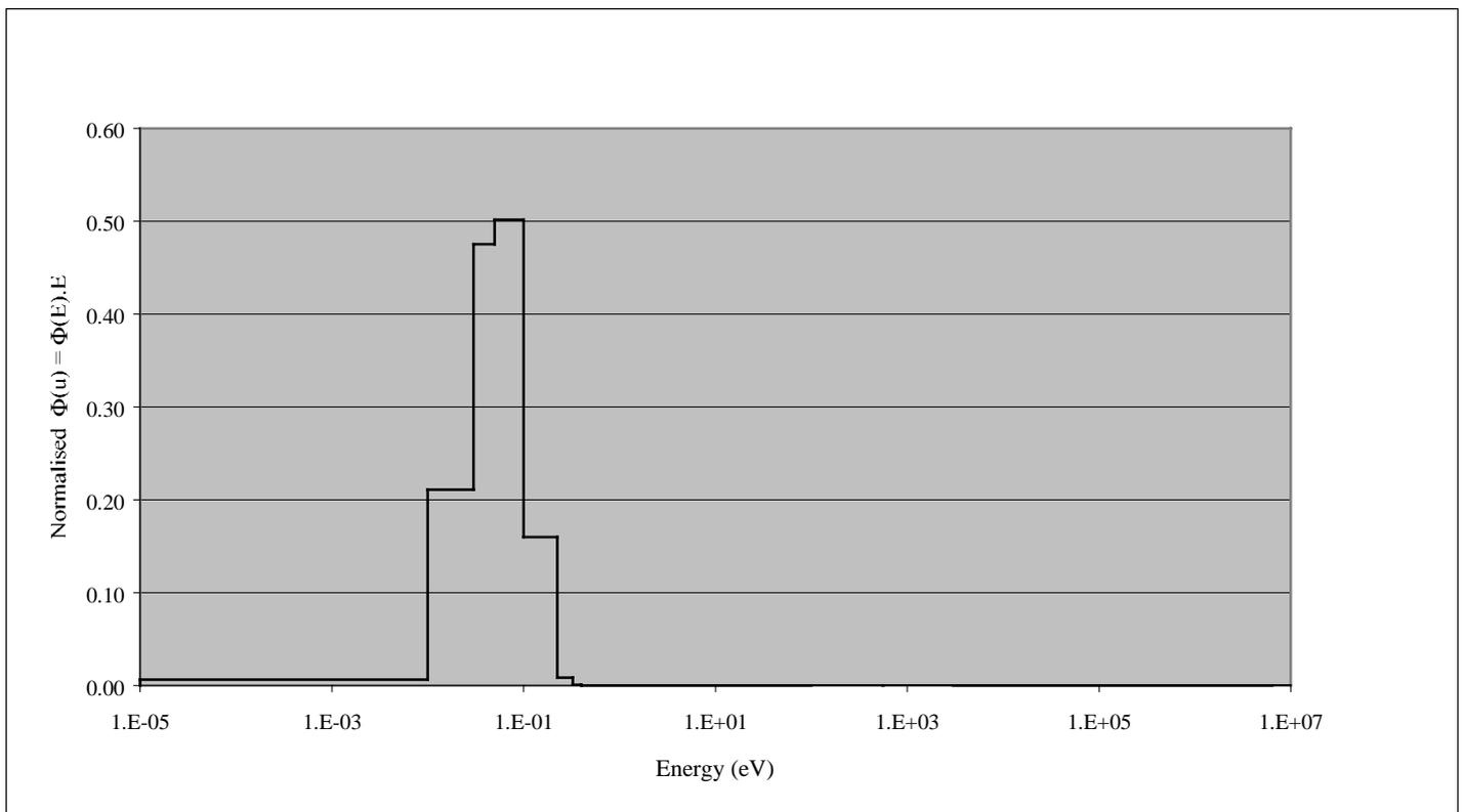
Figure 4. Energetic distribution of the neutron flux in Concrete
