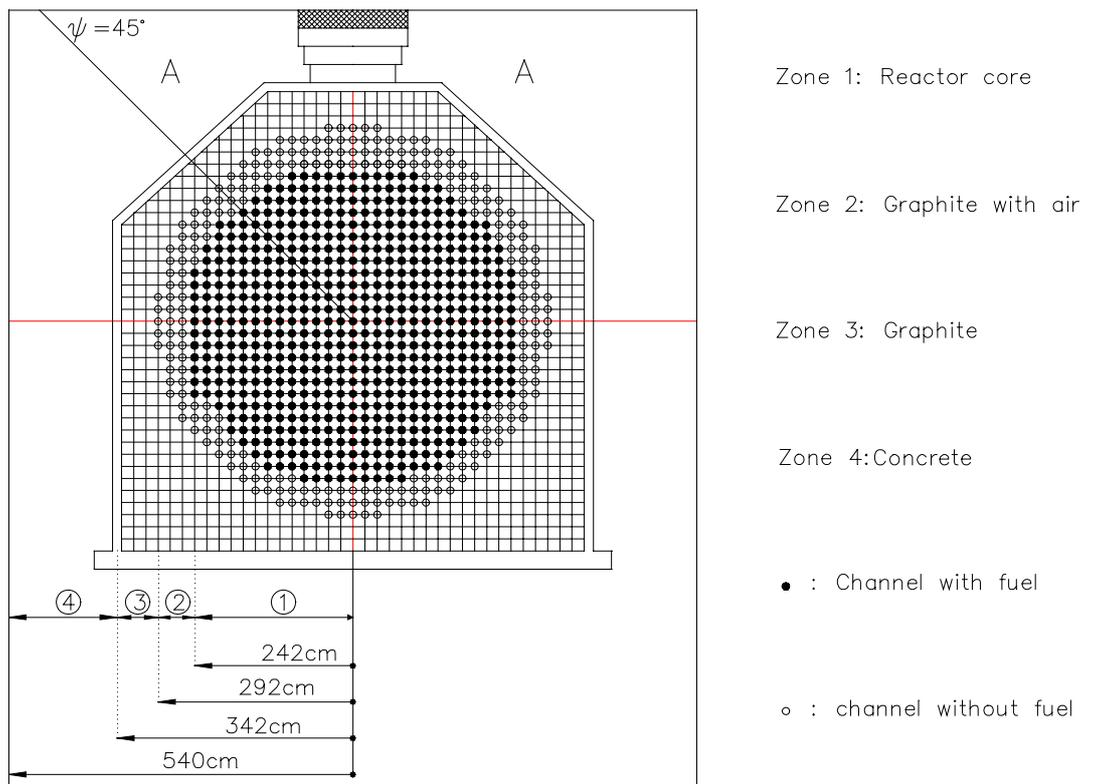
Figure 1. Axial schematic view of the BR1 reactor
