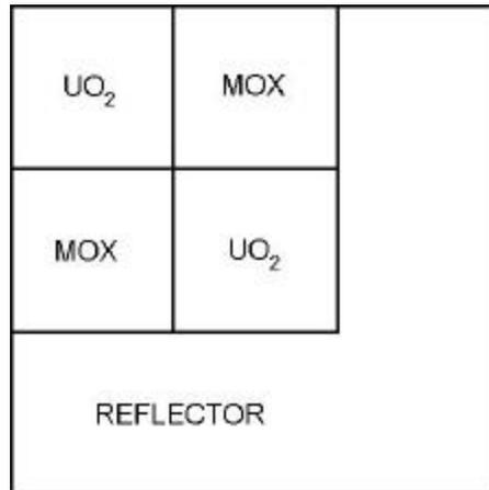
Figure. 2. Core Configuration for the C5 Benchmark Problem
