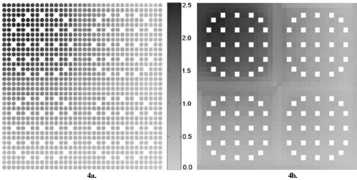
Figure 4. a) Fuel Pin Powers for the C5 Problem without Homogenization
