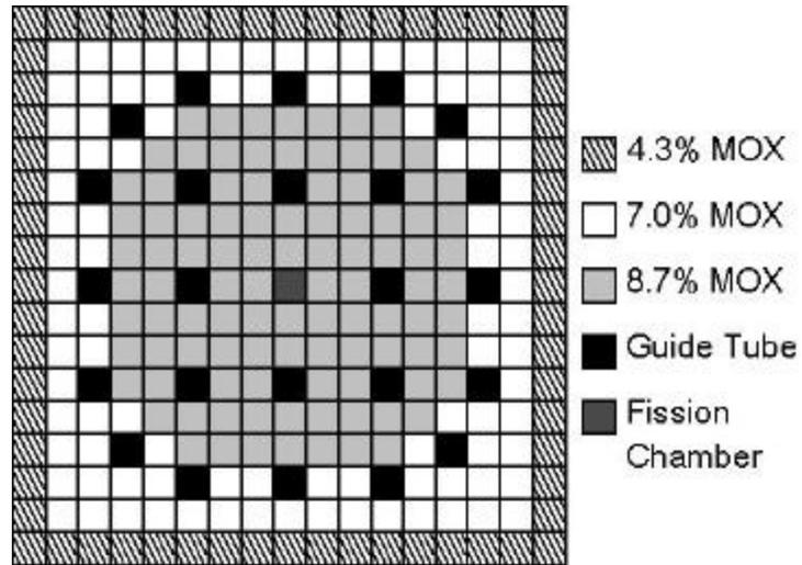
Figure 3. Composition Structure for a MOX Fuel Assembly
