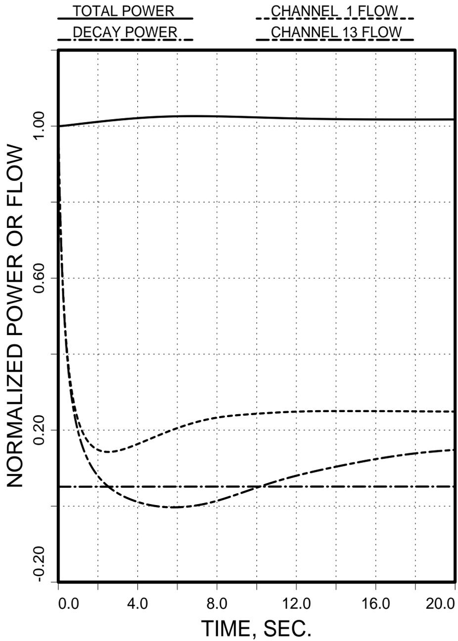
Fig. 6. Normalized Power and Flow Histories for Coolant Flow Transient.
