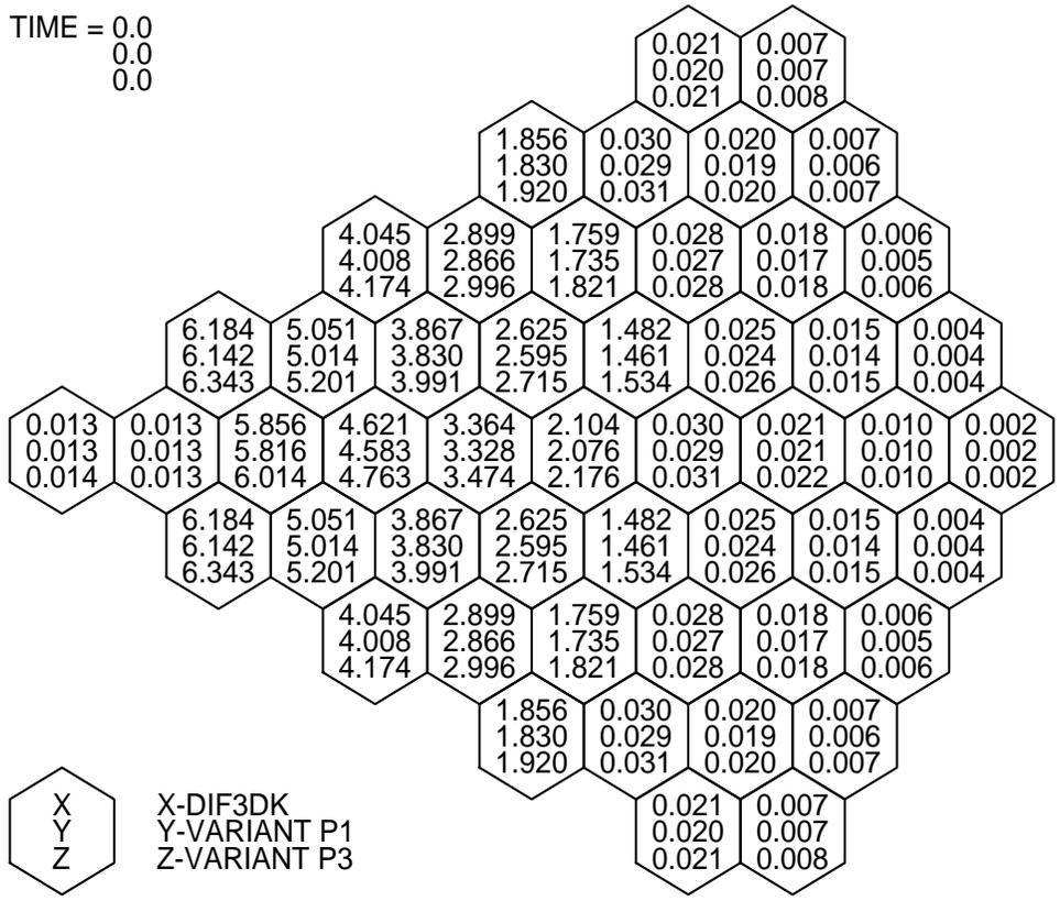
Fig. 2. Steady-State Subassembly Powers (MW) for Minor Actinide Burner Conceptual Design.
