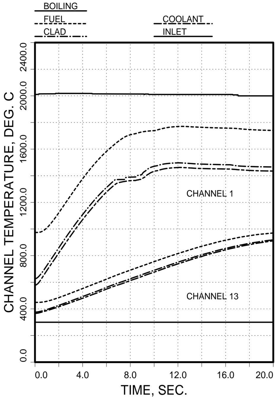
Fig. 7. Temperature Histories for Coolant Flow Transient.
