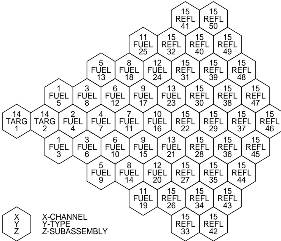
Fig. 1. Channel to Subassembly Assignment for Minor Actinide Burner Conceptual Design.
