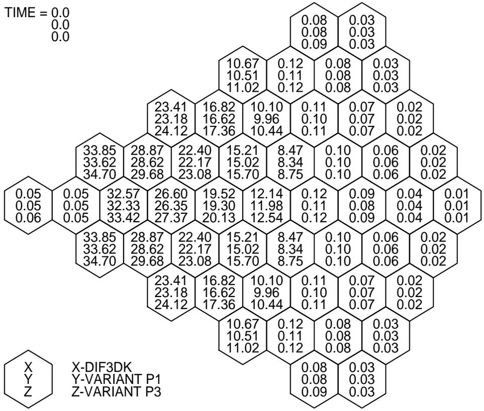
Fig. 3. Steady-State Linear Powers (kW/m) for Minor Actinide Burner Conceptual Design.
