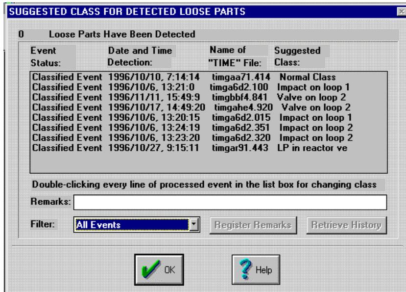
Figure 7. Example of the expert system display of HELPS loose parts monitoring system
