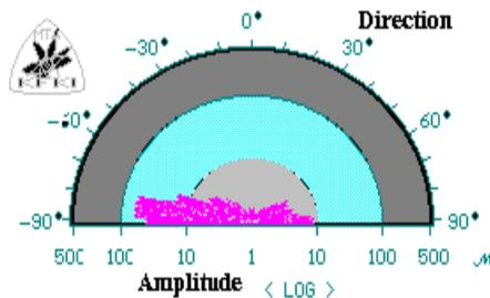
Figure 3b. Core barrel motion larger than 10 microns (less than 100 microns) was detected into 80 degree direction when one primary loop was closed.
