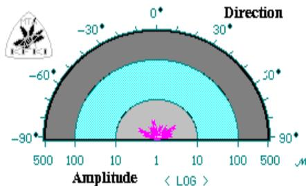
Figure 3a. Core barrel motion less than 10 micron (no motion) was observed
