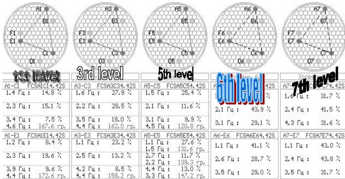
Figure 4. An example of the expert support display. Solid lines show in phase, dash lines show antiphase behaviour at different elevations between SPND signals at different frequencies (see table, in Russian)
