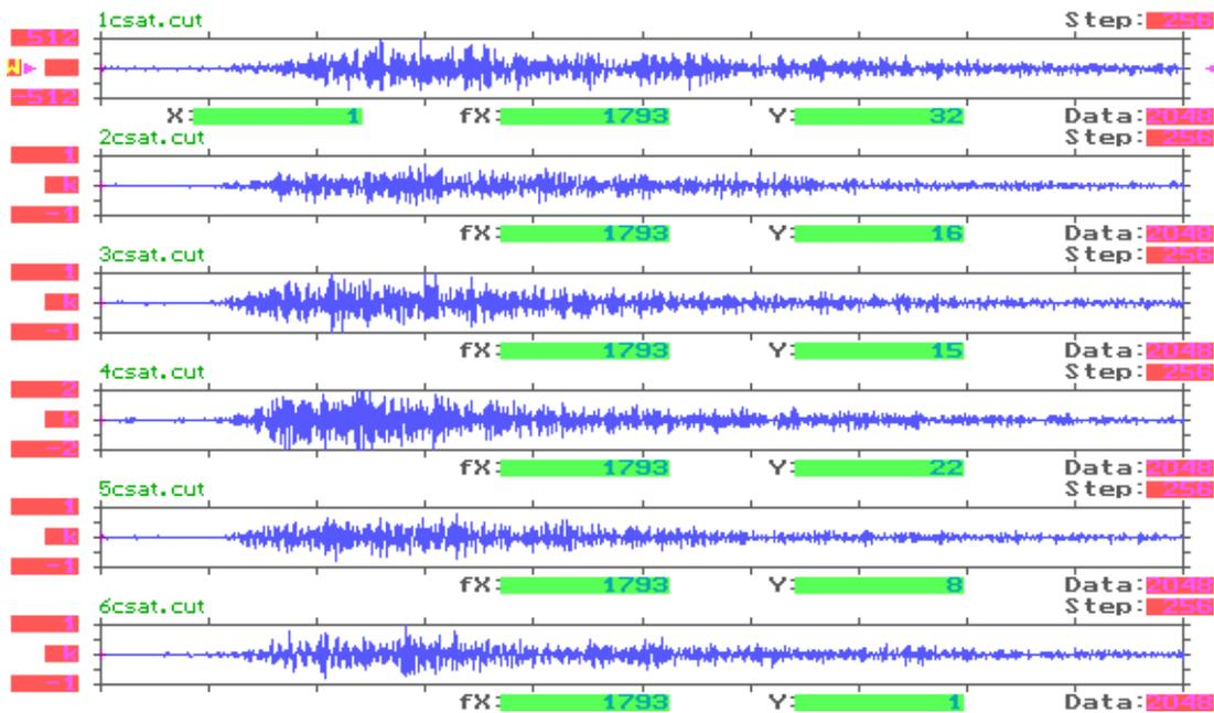
Figure 6. Screen of the HELPS loose part monitoring system during analysis of an event
