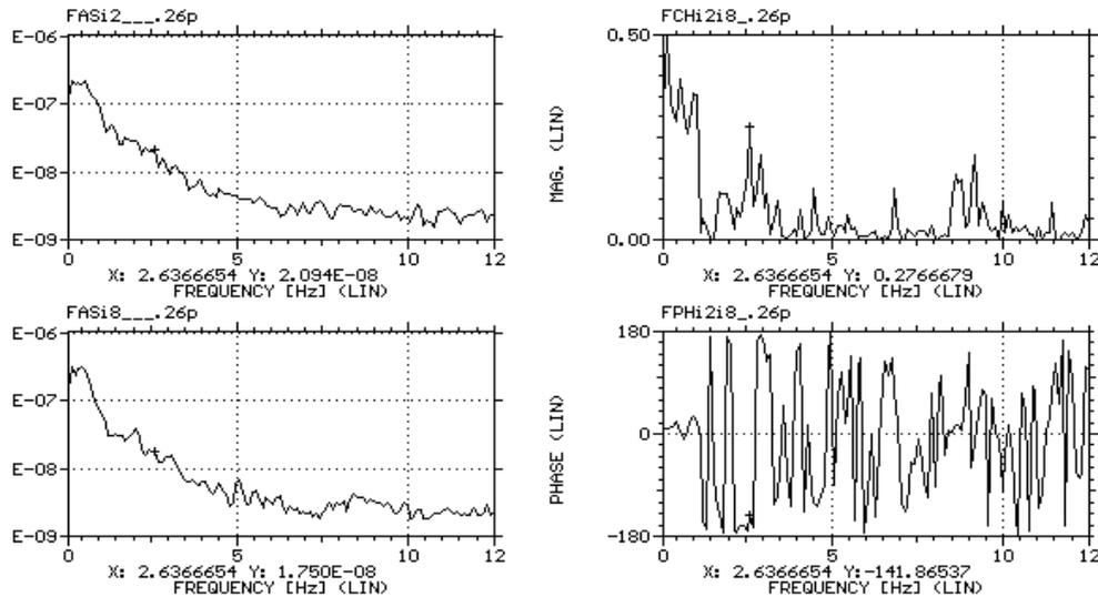
Figure 2. APSD, Phases and Coherence between ex-core detectors. Pedular motion would exhibit a peak, which is not found in the frequency range from 2 to 6 Hz, where antiphase was detected.
