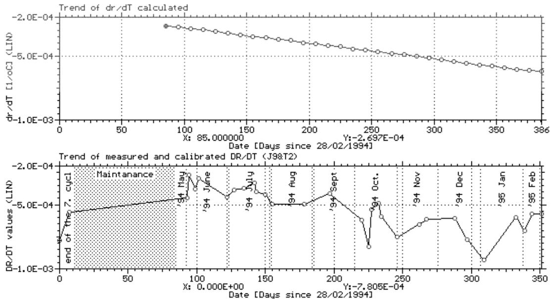
Figure 5. Estimated and actually measured (using noise method) values of temperature reactivity coefficient during a fuel campaign
