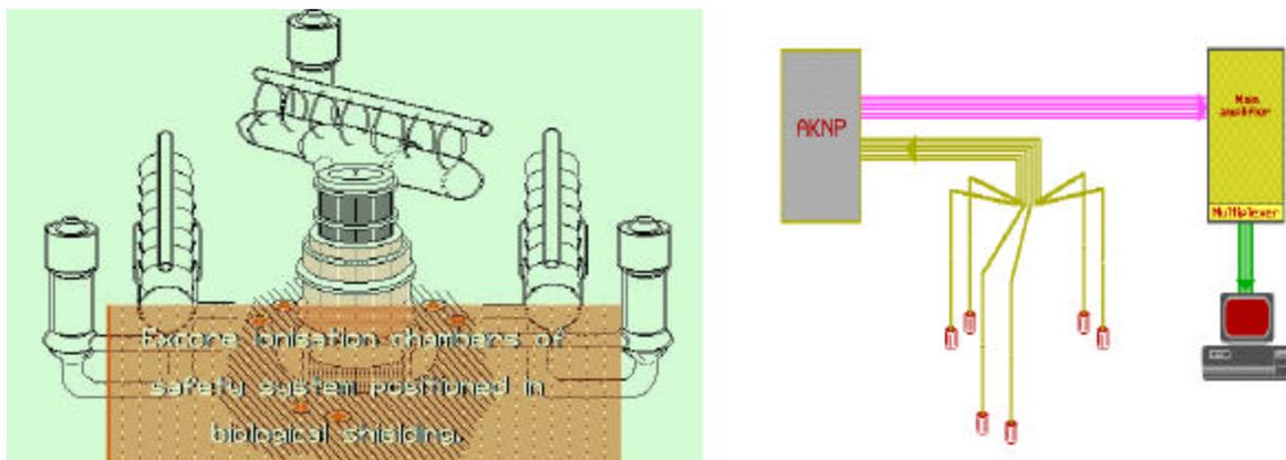
Figure 1. Physical positioning and electronics using the six state excore ionisation detectors of the AKNP safety system, which are positioned around the reactor vessel, for core barrel monitoring in WWER type reactors
