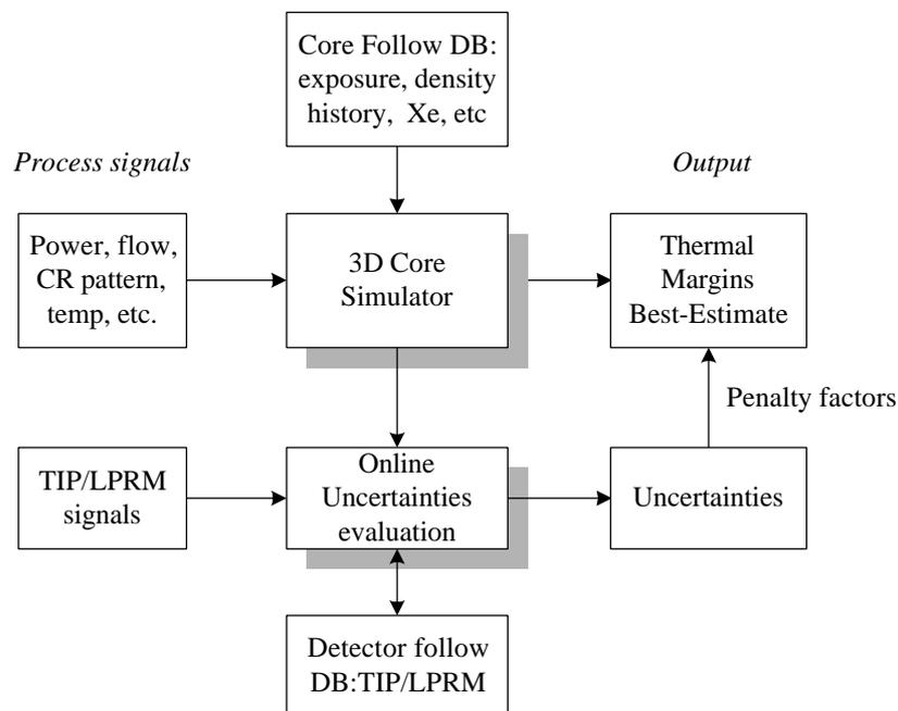
Figure 1 – Core Watch structure
