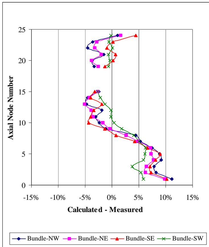
Figure 6 – Axial nodal deviations for 4 neighboring bundles at a TIP-string location
