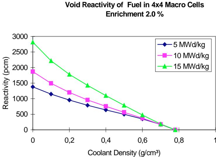
Figure 1: Void reactivity as function of coolant density for a macro-cell consisting of 4x4 fuel channels with an enrichment of 2.0% and different burnup states.
