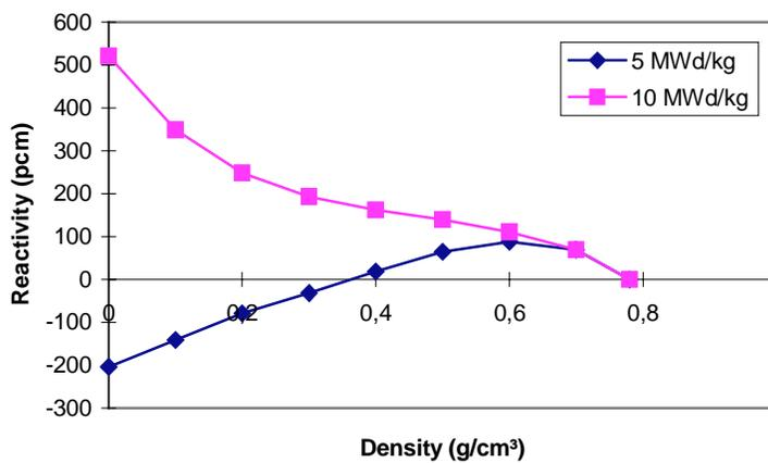
Figure 4: Void reactivity of a macro-cell, replacing three fuel channels by two water columns and one additional absorber.
