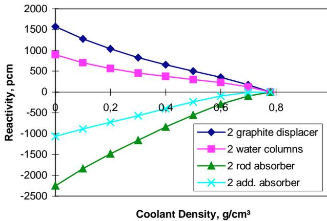
Figure 3: Macro-cell studies of void reactivity. Two fuel channels are replaced by non-fuel components
