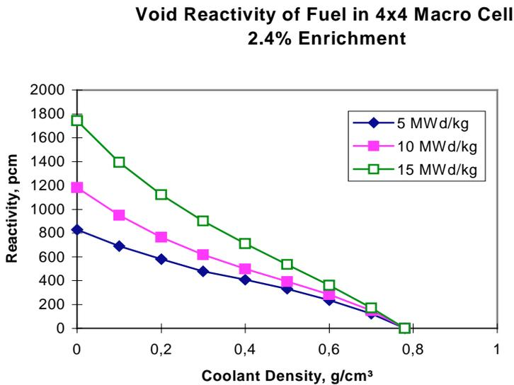
Figure 2: Void reactivity as function of coolant density for a macro-cell consisting of 4x4 fuel channels with an enrichment of 2.4% and different burnup states.
