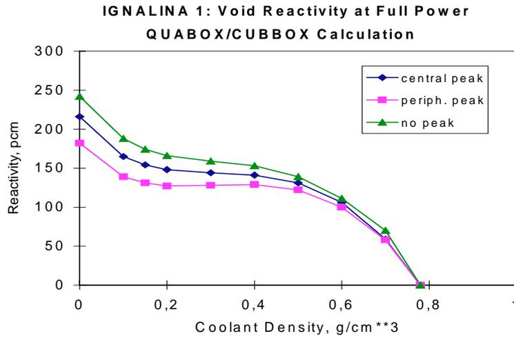
Figure 5: Void reactivity behaviour of Ignalina 1, March 94, depending on coolant density for an operational condition and two conditions with disturbed peaking power distributions.
