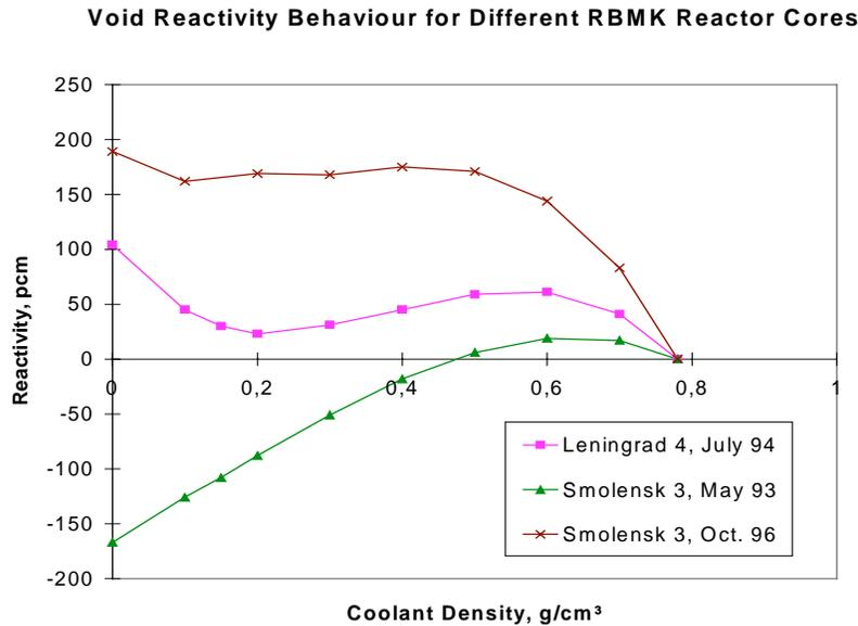
Figure 6: Void reactivity studies of operational states. Two different operational conditions of the plant Smolensk 3 and for comparison a state of Leningrad 4 are shown.
