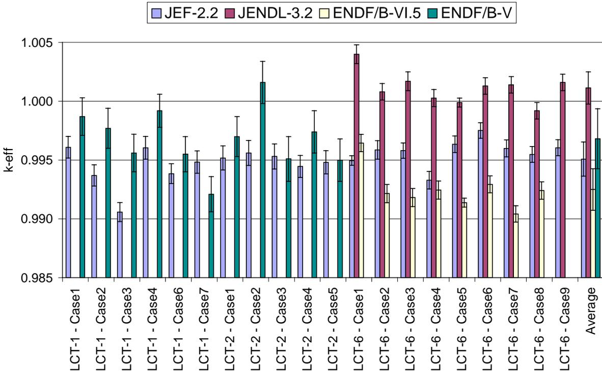
Figure 5.  $k_{\text{eff}}$  calculated by MCNP with different nuclear data for LEU-COMP-THERM benchmarks (UOX LWR lattices). Values for ENDF/B-V and JENDL-3.2 from [8].
