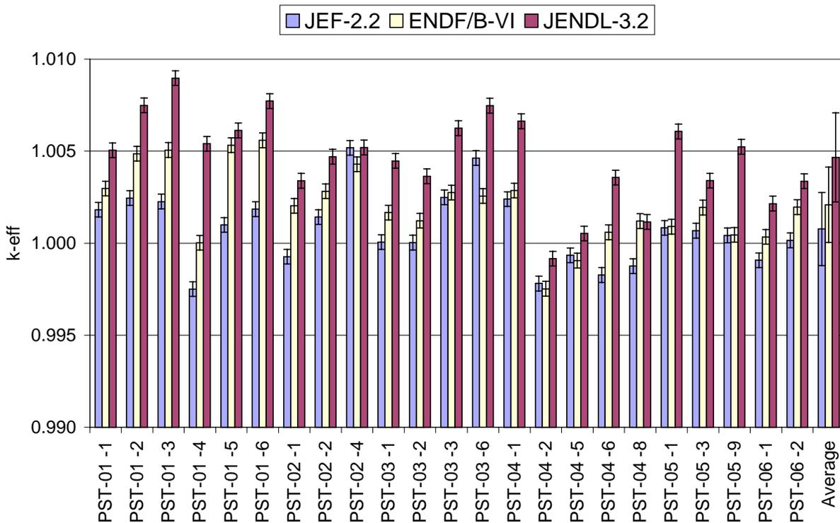
Figure 2.  $k_{\text{eff}}$  for the benchmarks PU-SOL-THERM-001 – 006 (PNL-Experiments) calculated with MCNP and different nuclear data.
