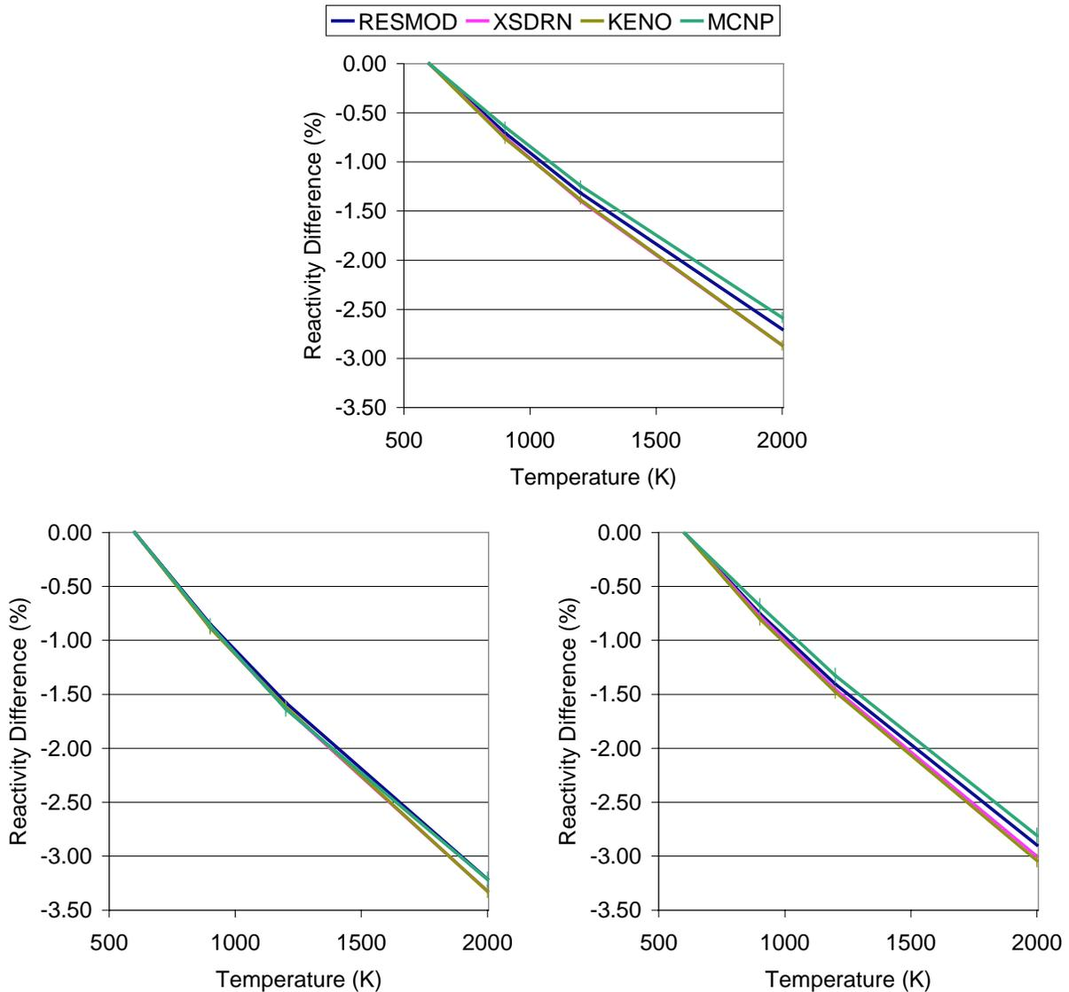
Figure 10. Reactivity change as a function of fuel temperature for pin cells defined in the ROWLANDS benchmark. Calculations were performed with JEF-2.2 data.
