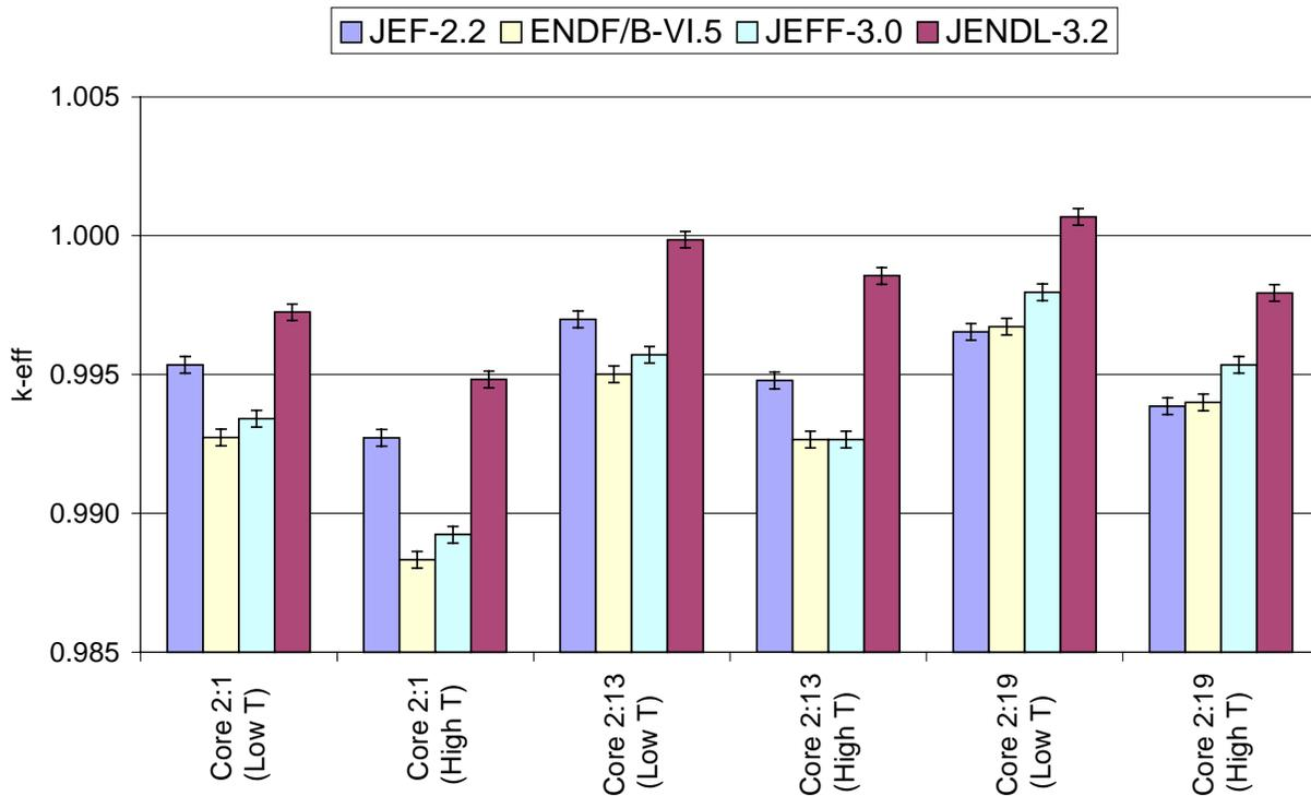
Figure 9. MCNP results for KRITZ benchmarks core 2:1, 2:13, and 2:19, each at room and high temperatures, with different data evaluations.
