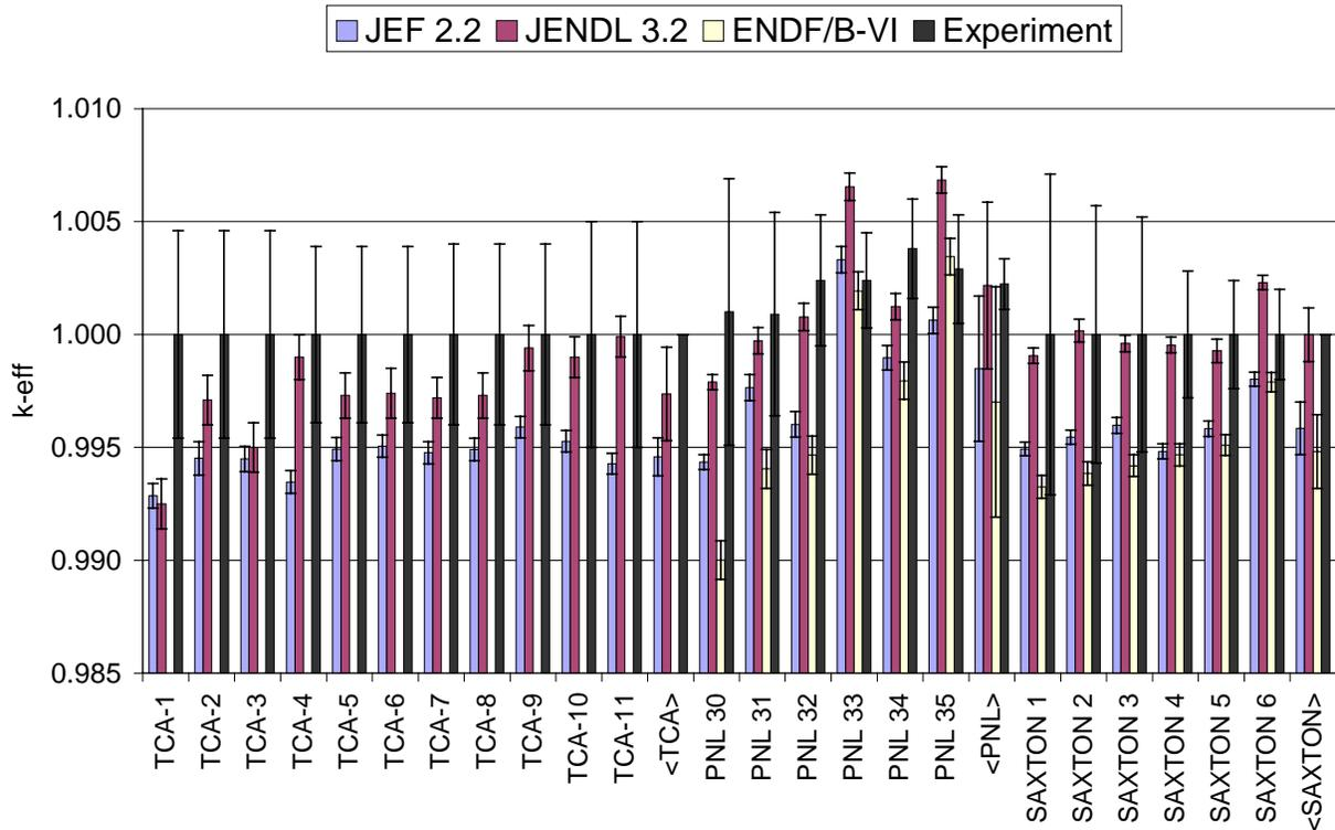
Figure 8.  $k_{\text{eff}}$  calculated by MCNP with different data libraries for MIX-COMP-THERM benchmarks (MOX LWR lattices) compared with experiment.
