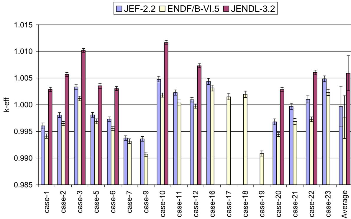
Figure 4.  $k_{\text{eff}}$  for SPERT-D Experiments, HEU-MET-THERM-006: MCNP calculations based on different cross section libraries.
