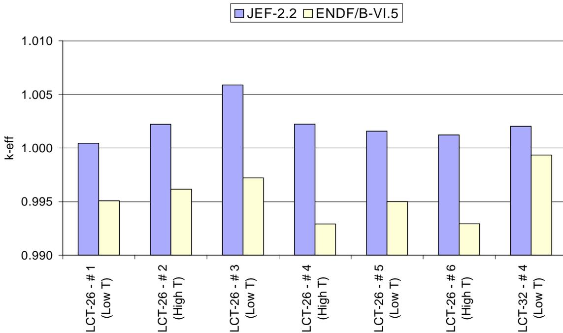
Figure 7. MCNP results for hexagonal LEU LWR lattices at room and higher temperatures.
