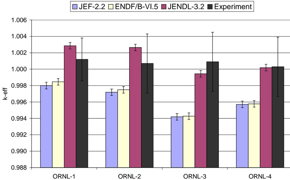
Figure 1.  $k_{\text{eff}}$  for ORNL Experiments 1–4: MCNP calculations with different data libraries compared to measured values.
