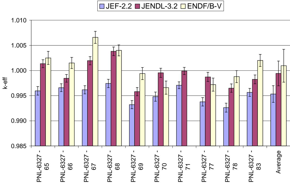
Figure 3.  $k_{\text{eff}}$  for benchmarks MIX-SOL-THERM-004 (PNL-Experiments). MCNP calculations based on different cross sections. ENDF/B-V results are taken from [8].
