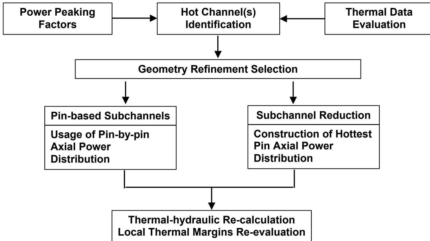
Fig 1. Procedure of the Integrated Local Safety Margin Evaluations
