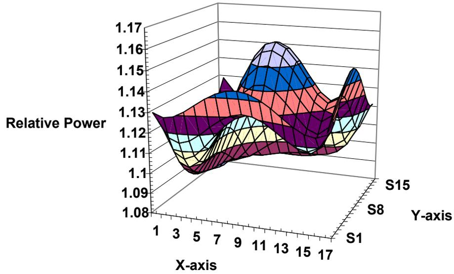
Fig 4. Radial Pin Relative Power Profile in the Hottest Node for Steady State MSLB TMI Model
