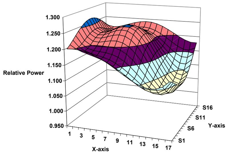
Fig 6. Radial Pin Relative Power Profile in the Hottest Node at 8.7 sec in the Transient of MSLB TMI Model
