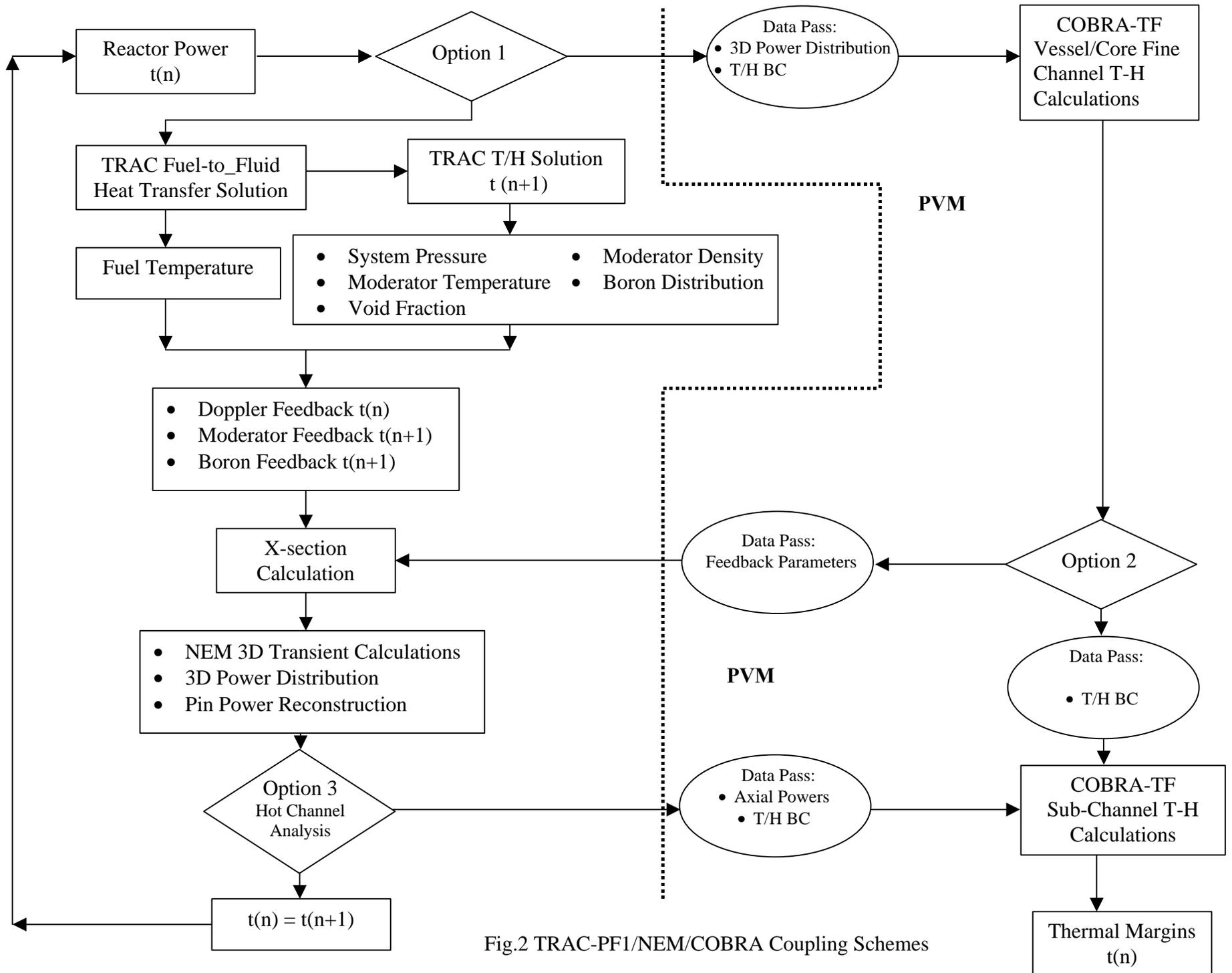
Fig.2 TRAC-PF1/NEM/COBRA Coupling Schemes
