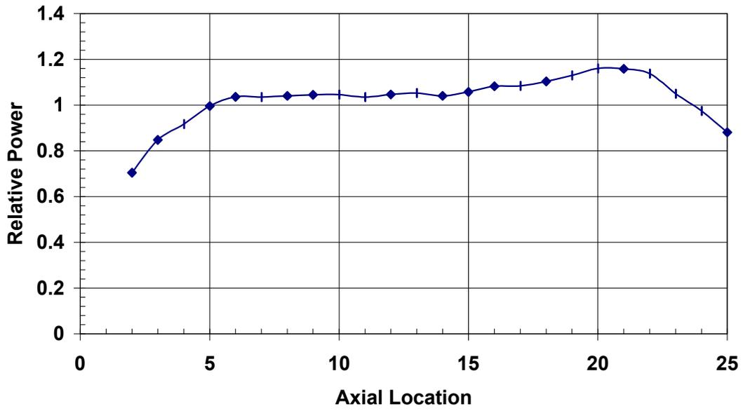
Fig 3. Axial Peak Pin Relative Power Profile in the Hottest Assembly for Steady State MSLB TMI Model
