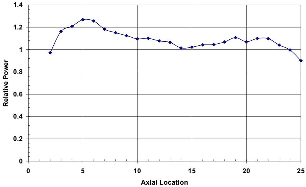
Fig 5. Axial Peak Pin Relative Power Profile in the Hottest Assembly at 8.7 sec in the Transient of MSLB TMI Model
