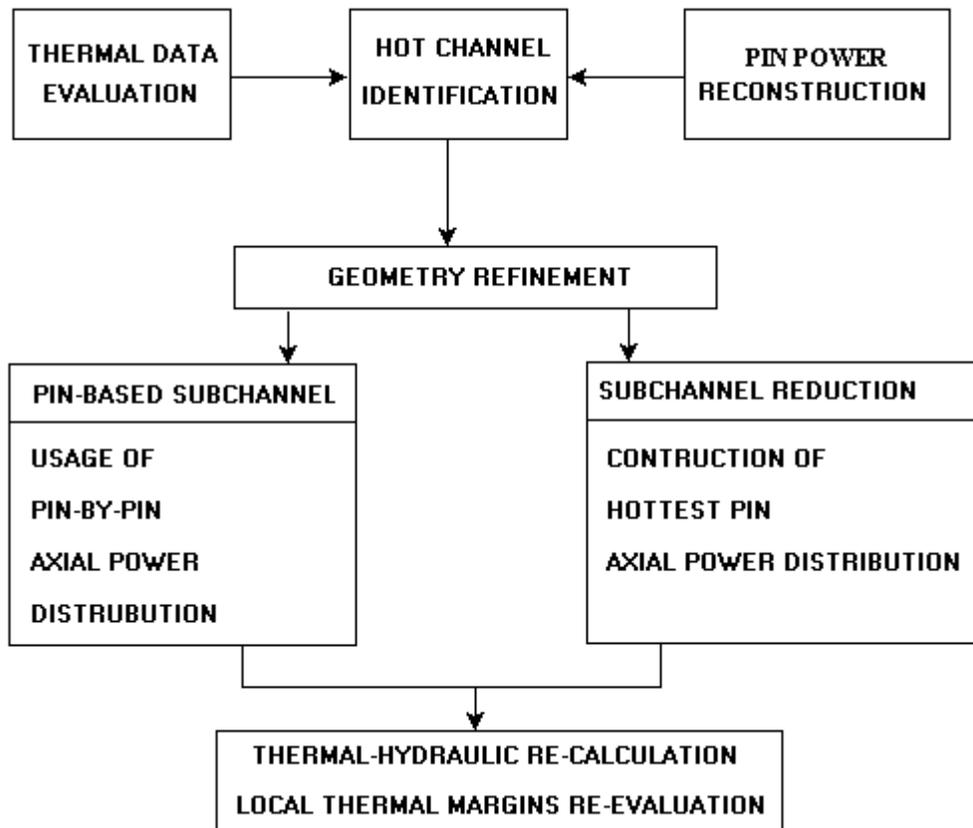
Figure 5. Scheme of the integrated local safety margin evaluation
