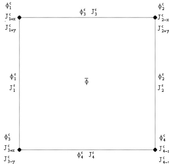
Figure 1. Flux and current data needed for a high order interpolation
