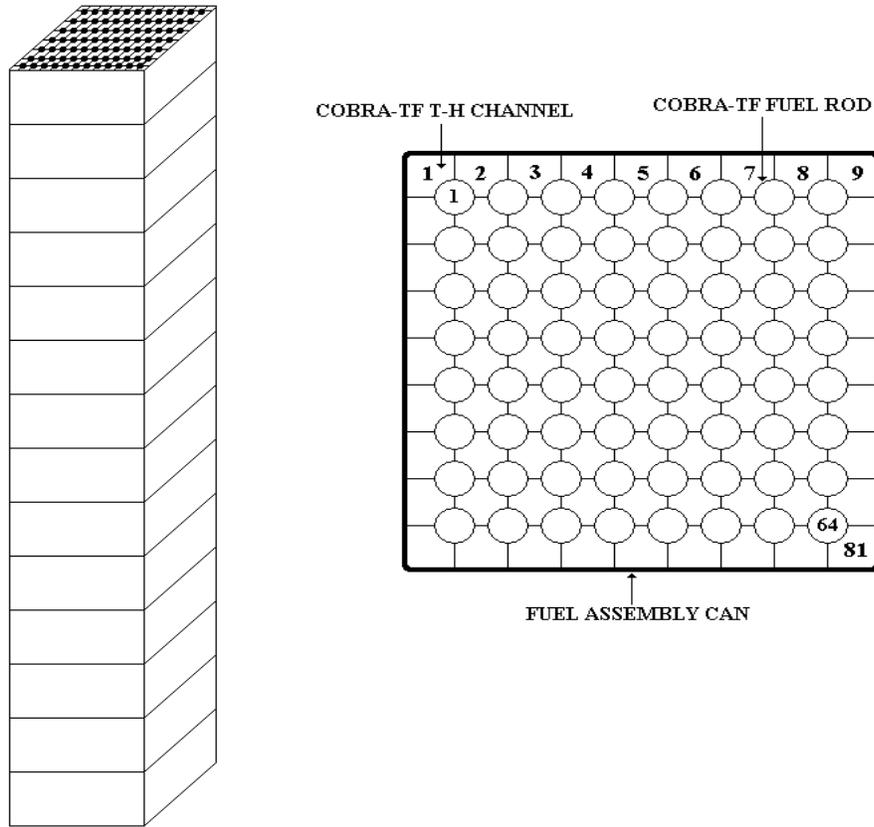
Figure 8. Typical 8x8 fuel Rod Array COBRA-TF Hot-Channel Model
