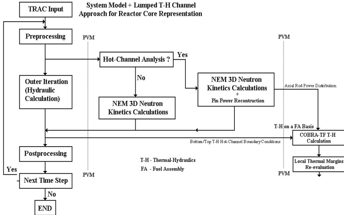
Figure 4. TRAC-BF1/NEM Hot-Channel Coupling Approach Using PVM
