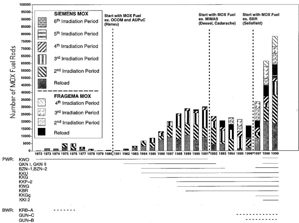
Figure 1. Core Management Experience with Commercial MOX Insertion in BWR and PWR by SIEMENS KWU Group (Status: End of 1999)
