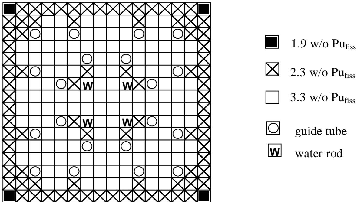
Figure 2. Standard MOX FA (16x16), Carrier Material  $U_{nat}$ , 2.91 w/o Average  $Pu_{fiss}$  Content
