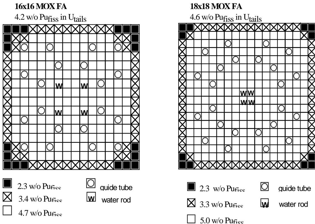
Figure 3. Different MOX-FA Designs for Higher Burnup for 16x16 and 18x18 FAs
