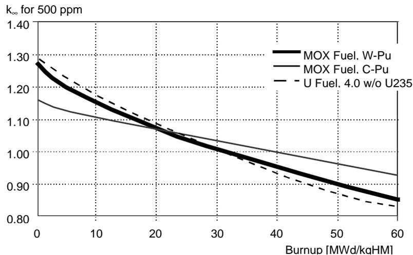
Figure 6. Comparison of Reactivity-Behavior for PWR-FAs
