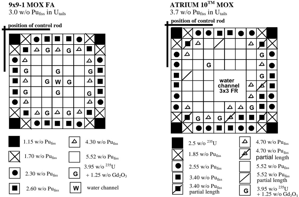
Figure 5. Different MOX-FA Designs for BWRs (9x9 and 10x10 Rod Lattice Type)
