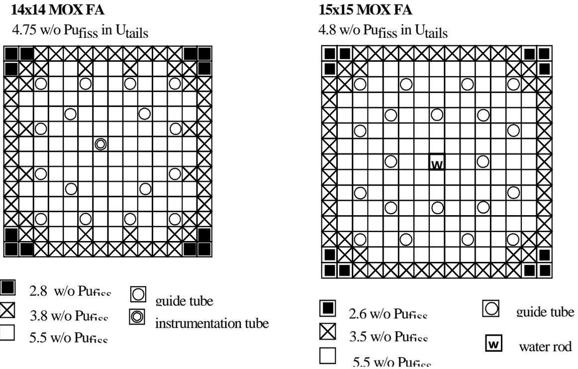
Figure 4. MOX-FA Designs for Higher Burnup for 14x14 and 15x15 MOX FAs
