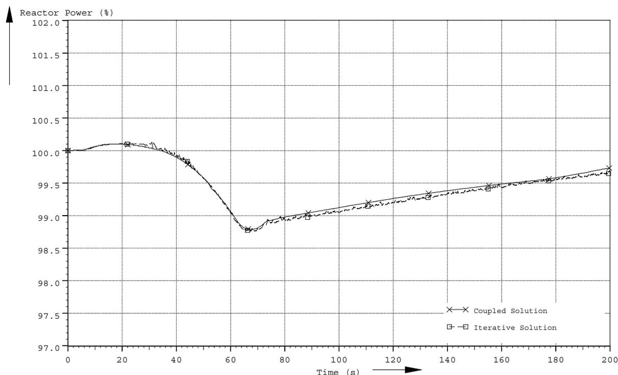
Figure 3. Inadvertent Opening of a Pressurizer Relief Valve: Comparison between Iterative (4 iterations) and Coupled Solution
