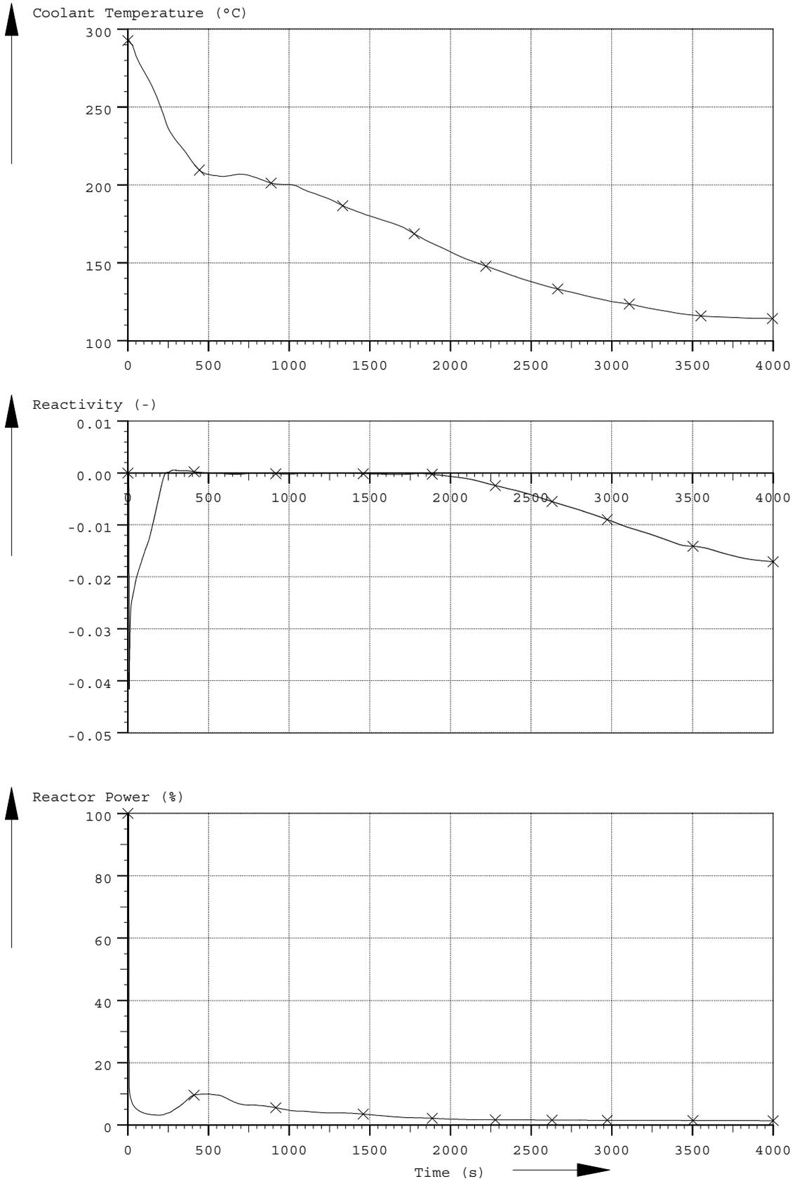
Figure 4. R/P/C Results for a Multiple Steam Line Leak
