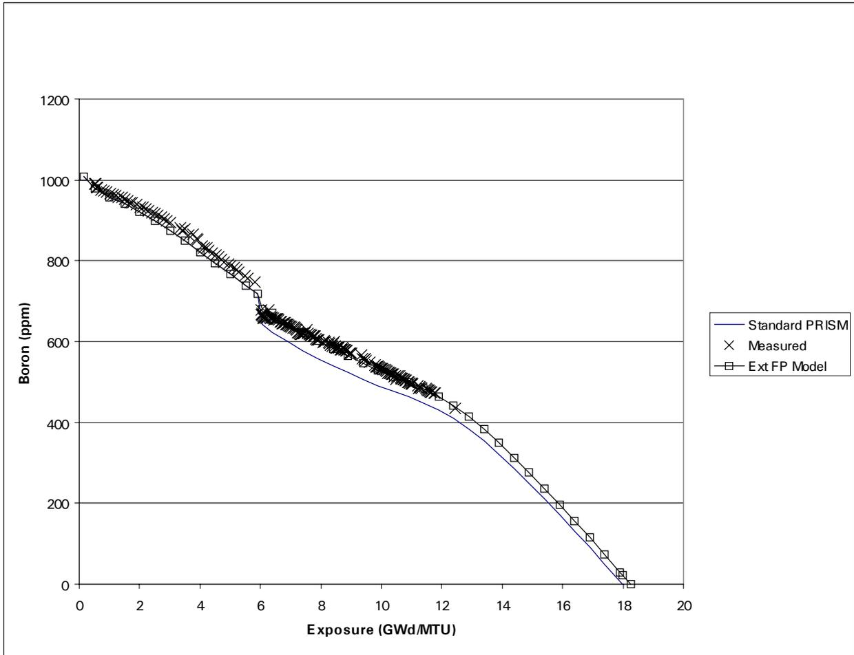
Figure 2. Critical Boron Concentration for Operation Before and After Extended Shutdown
