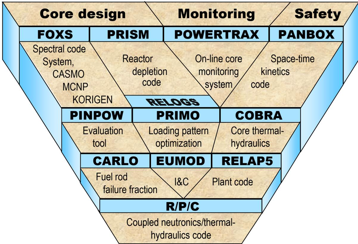
Figure 1. Integrated Code System CASCADE-3D for Advanced Core Design and Safety Analysis
