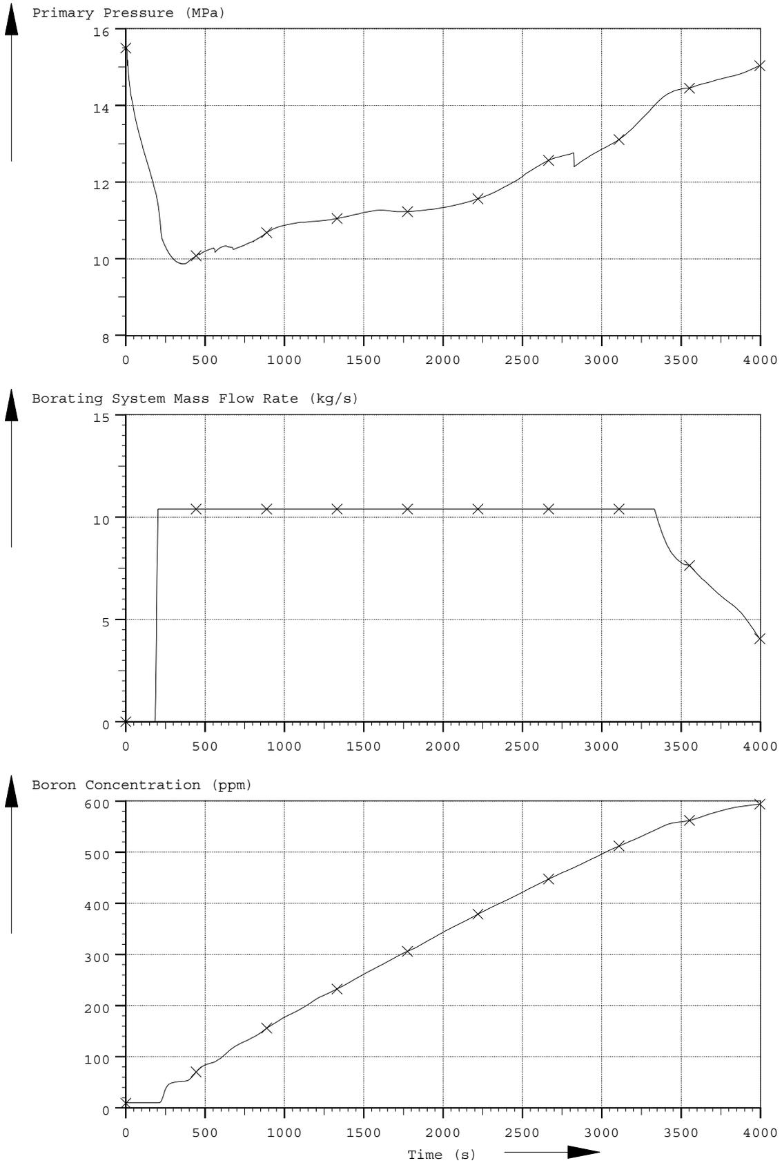
Figure 5. R/P/C Results for a Multiple Steam Line Leak
