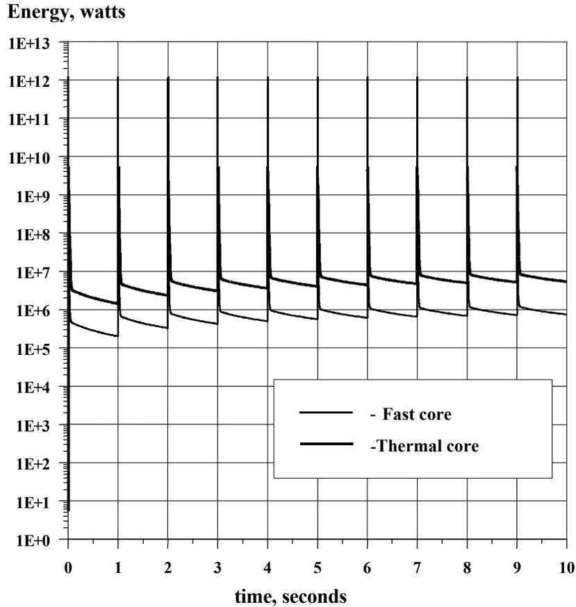
**Figure 3.** Transient processes in blanket zones for pulse-periodical mode.
