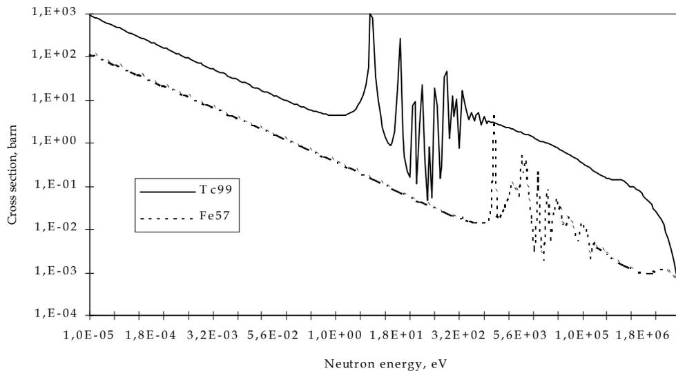
**Figure 4.** Energy dependencies of radiation capture cross-sections for  $\text{Tc}^{99}$  and  $\text{Fe}^{57}$ .
