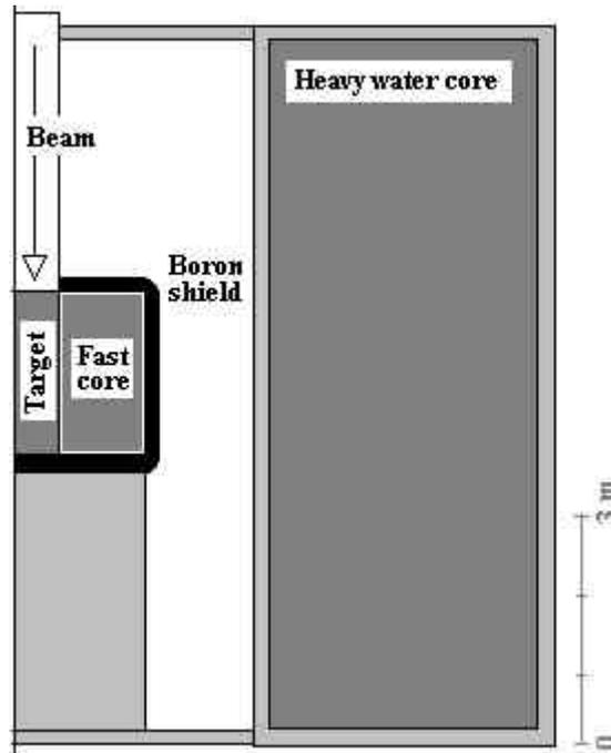
**Figure 2.** Coupled fast/thermal spectrum blanket system.
