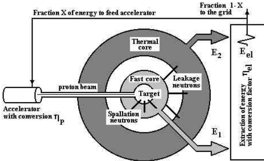
Figure 1. Schematic of the ADS.
