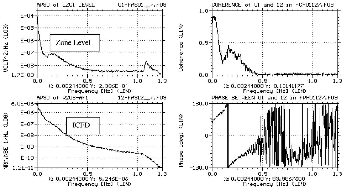
Figure 15. Normalized APSD, coherence and phase functions of the Liquid Zone Level noise and the RRS-B ICFD noise measured in Zone 1 in Pickering-B Unit 6.
