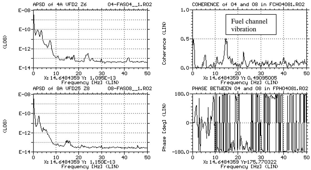
Figure 12. Normalized APSD, coherence and phase functions of flux noise signals from RRS-A ICFDs in Zones 6 and 8, lined up along the same set of fuel channels in Darlington **Unit 2**.
