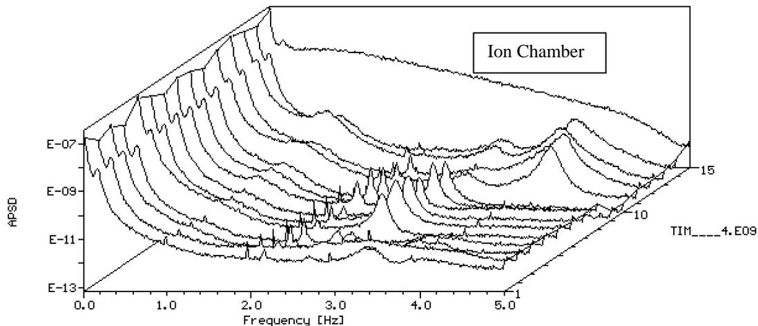
Figure 1. Normalized APSP functions of fourteen ICFD noise signals and the ion chamber noise signal from Channel A of the Reactor Regulating System (RRS-A), measured in Pickering-B Unit 5.
