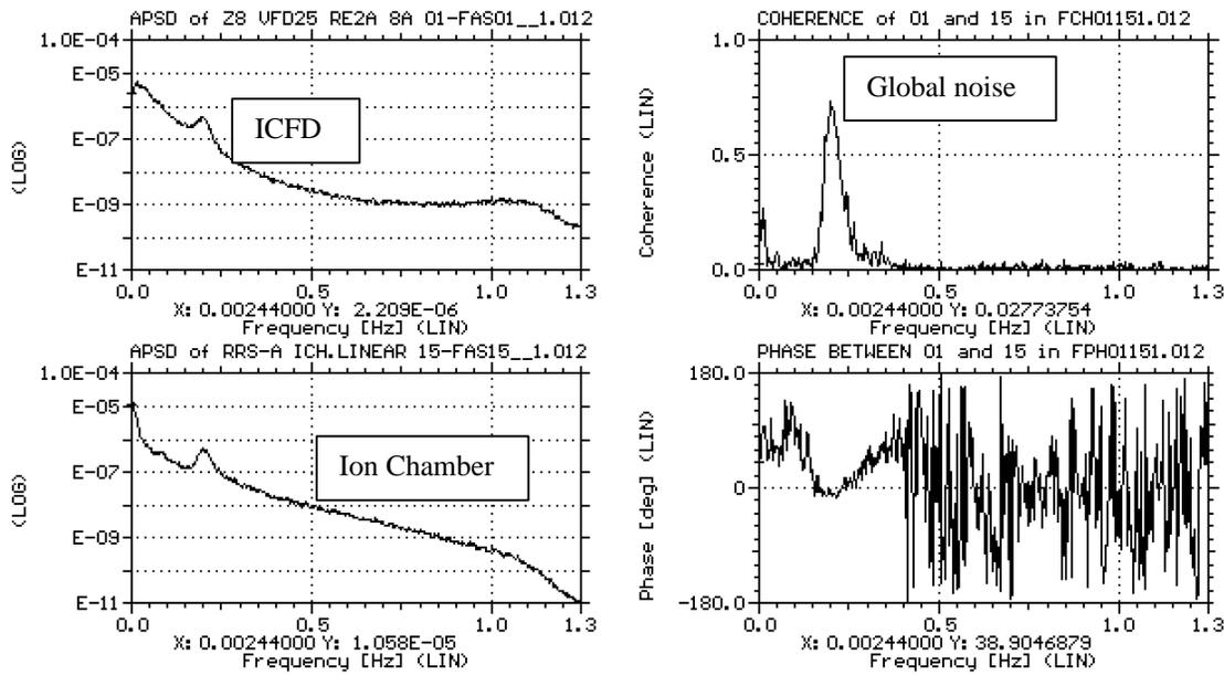
Figure 3. Normalized APSD, coherence and phase functions of flux noise signals from Zone 8 ICFD VFD25-RE2A and RRS-A ion chamber. The peak at 0.2 Hz is a global reactivity oscillation caused by the global oscillations of liquid zone levels in the 14 light water compartments in Bruce-B Unit 7.
