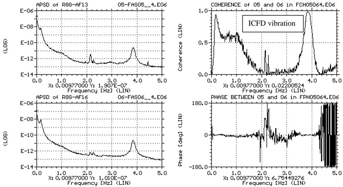
Figure 5. Normalized APSD, coherence and phase functions of flux noise signals from two SDS2-G ICFDs located in the same horizontal detector tube, HFD8, measured in Pickering-B Unit 5.
