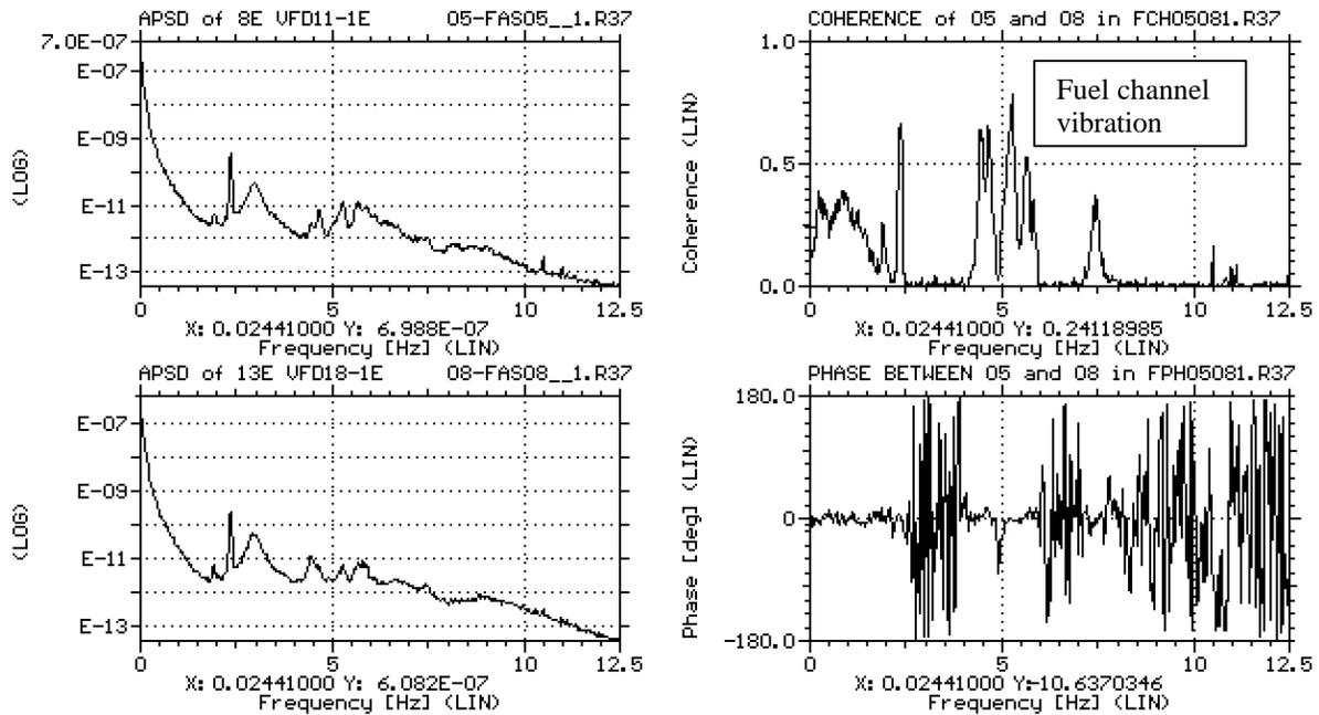
Figure 10. Normalized APSD, coherence and phase functions of flux noise signals from ICFDs VFD11-1E and VFD18-1E lined up along the same set of fuel channels in Zones 6 and 8 in Darlington Unit 2.
