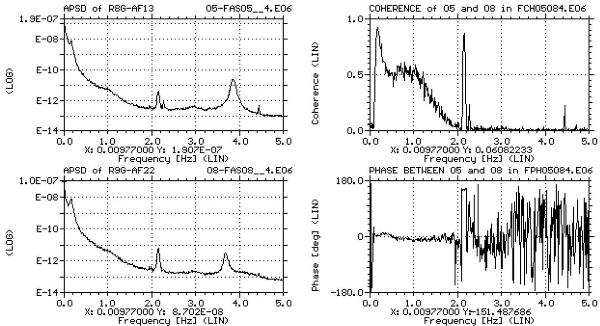
Figure 6. Normalized APSD, coherence and phase functions of flux noise signals from two SDS2-G ICFDs located in different horizontal detector tubes, HFD8 and HFD9, measured in Pickering-B Unit 5.
