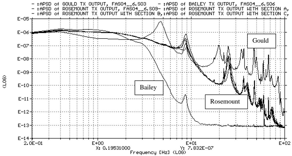
Figure 17. Normalized APSD functions of flow noise signals from Rosemount, Gould, and Bailey flow transmitters installed on safety system flow loop FT-3J in Darlington Unit 3.
