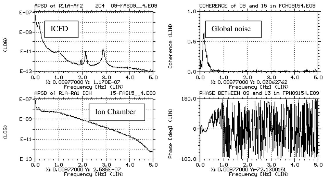
Figure 2. Normalized APSP, coherence and phase functions of noise signals of ICFD R11A-AF2 from Zone 4 and the linear output of the ion chamber from RRS-A. The peak at 0.2 Hz is a global reactivity oscillation caused by the global oscillations of liquid zone levels in the 14 light water compartments in Pickering-B Unit 5.
