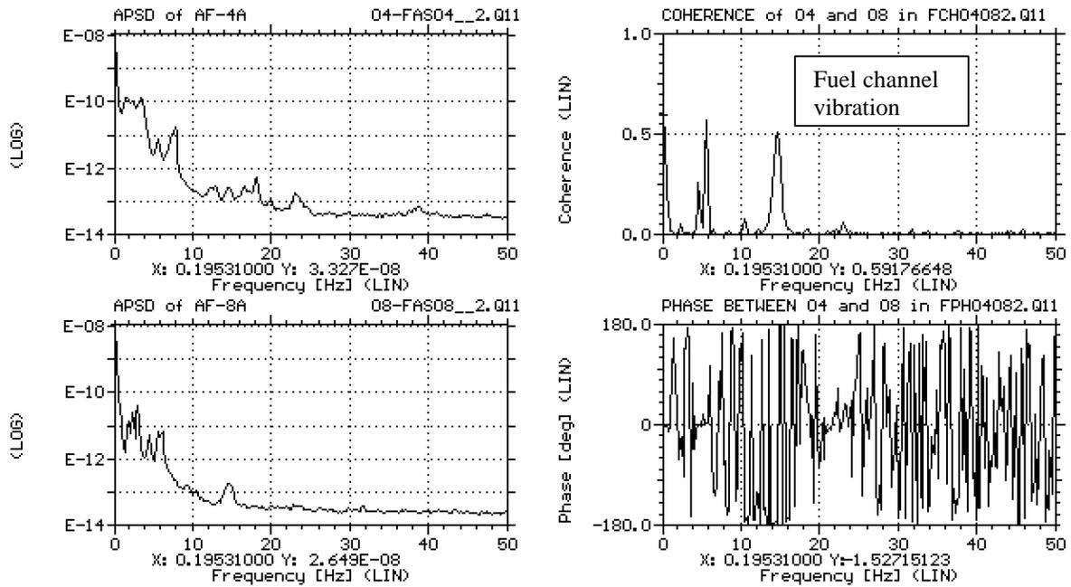
Figure 11. Normalized APSD, coherence and phase functions of flux noise signals from RRS-A ICFDs in Zones 6 and 8, lined up along the same set of fuel channels in Darlington **Unit 1**.
