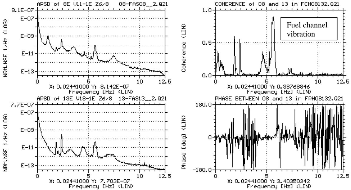
Figure 9. Normalized APSD, coherence and phase functions of flux noise signals from ICFDs VFD11-1E and VFD18-1E lined up along the same set of fuel channels in Zones 6 and 8 in Darlington Unit 1.
