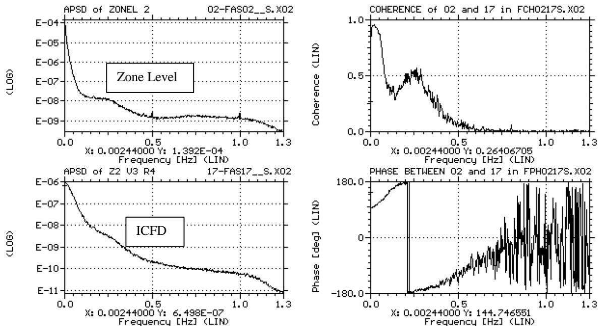
Figure 16. Normalized APSD, coherence and phase functions of the Liquid Zone Level noise and the RRS-A ICFD noise measured in Zone 2 in Darlington Unit 3.
