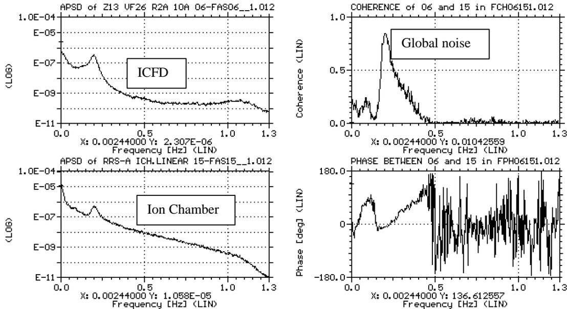
Figure 4. Normalized APSD, coherence and phase functions of flux noise signals from Zone 13 ICFD VFD26-RE2A and RRS-A ion chamber. The peak at 0.2 Hz is a global reactivity oscillation caused by the global oscillations of liquid zone levels in the 14 light water compartments in Bruce-B Unit 7.
