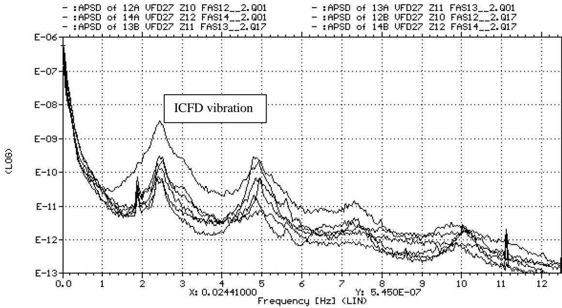
Figure 7. Normalized APSD functions of flux noise signals from ICFDs located in the same vertical flux detector tube, VFD27, measured in Darlington Unit 1 at full power operation.
