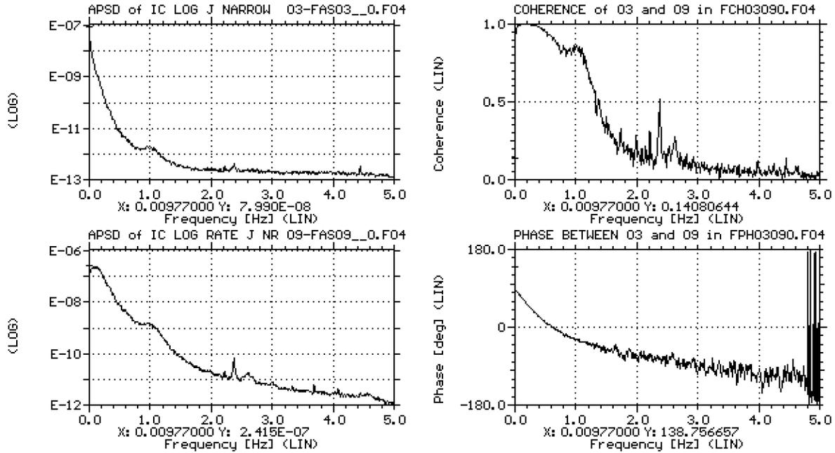
Figure 13. Normalized APSD, coherence and phase functions of Ion Chamber Log N and Log Rate noise signals from SDS2 Channel J, sampled at 10 Hz at full power in Pickering-B Unit 6.
