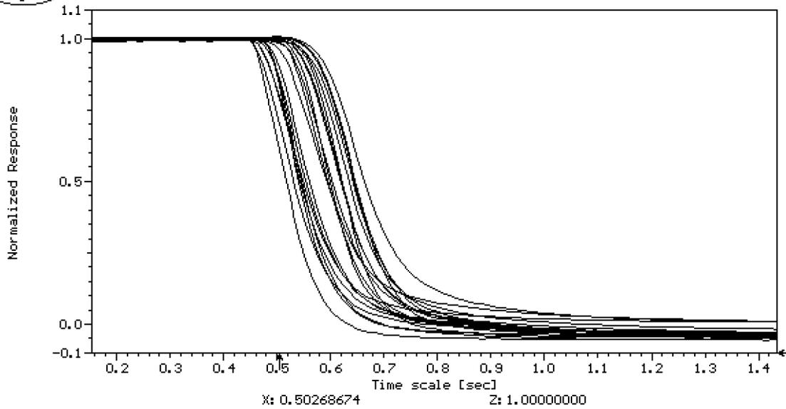
Figure 20. Normalized rundown signals of SDS1 Channel F overprompt ICFDs and Channel F/H ion chambers measured in an SDS2 trip in Darlington Unit 4 in April 1999.
