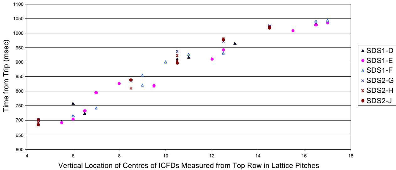
Figure 22. Prompt fractions and 50%-level crossing times of the new ICFDs in an SDS1-initiated trip in Pickering Unit 5 (ICFD commissioning test in June 1999).
