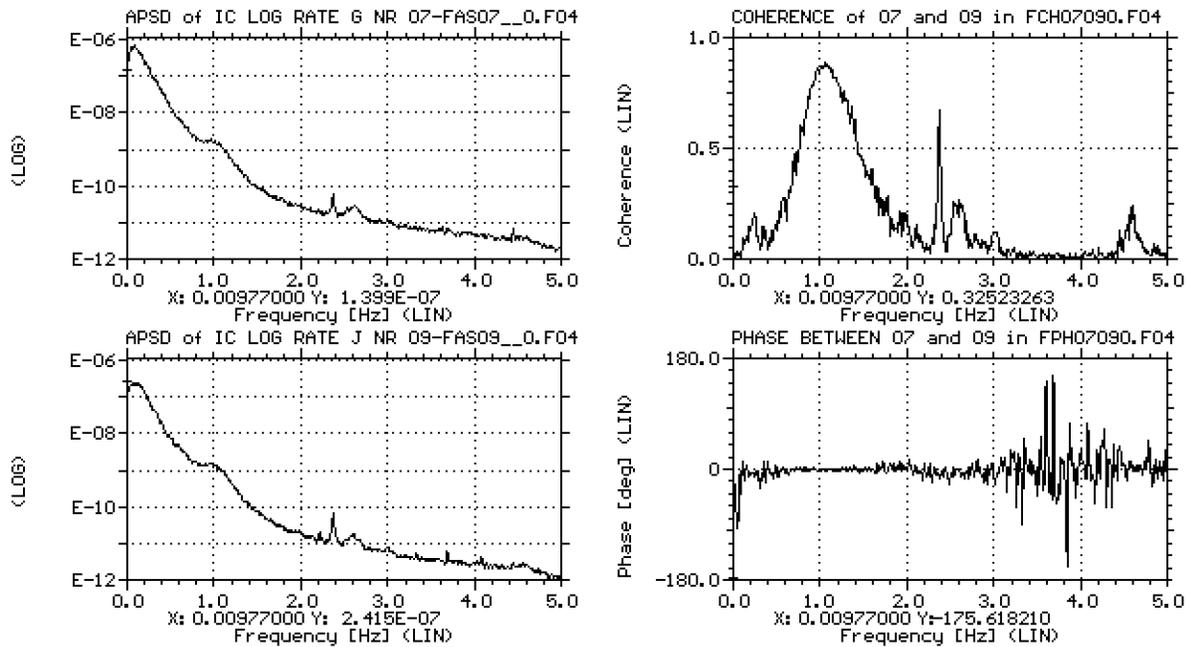
Figure 14. Normalized APSD, coherence and phase functions of Ion Chamber Log Rate noise signals from SDS2 Channels G and J, sampled at 10 Hz at full power in Pickering-B Unit 6.
