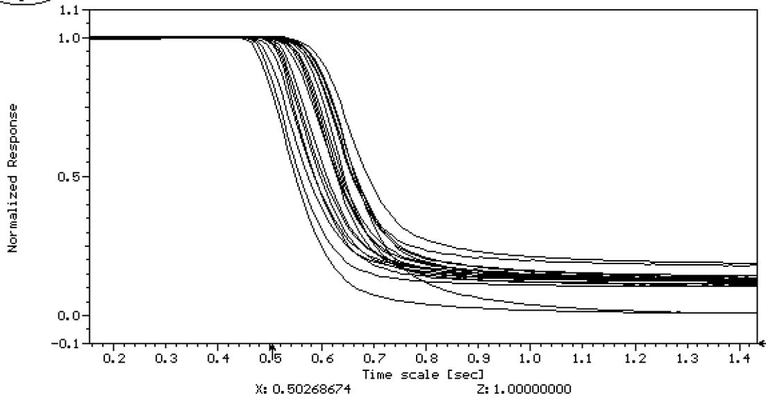
Figure 21. Normalized rundown signals of SDS2 Channel H underprompt ICFDs and Channel F/H ion chambers measured in an SDS2 trip in Darlington Unit 4 in April 1999.
