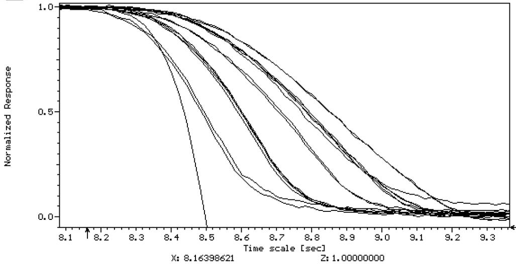
Figure 19. Rutdown response signals of RRS-B ICFD and ion chamber signals normalized by their pre-trip signals in an SDS1-initiated trip from 60% of full power in Darlington Unit 1.
