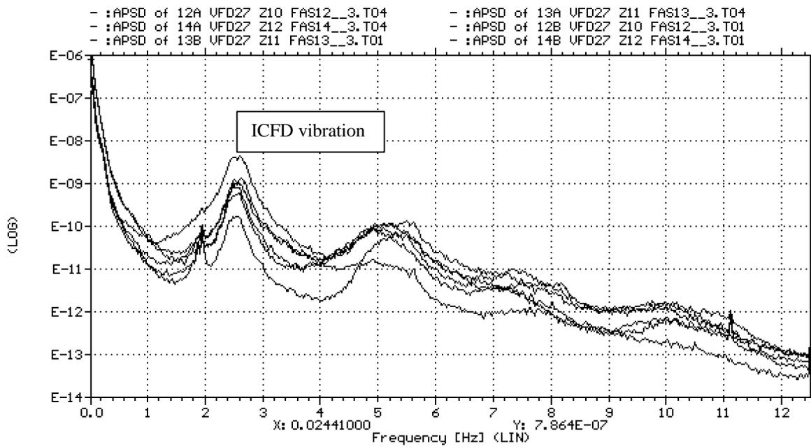
Figure 8. Normalized APSD functions of flux noise signals from ICFDs located in the same vertical flux detector tube, VFD27, measured in Darlington Unit 4 at full power operation.
