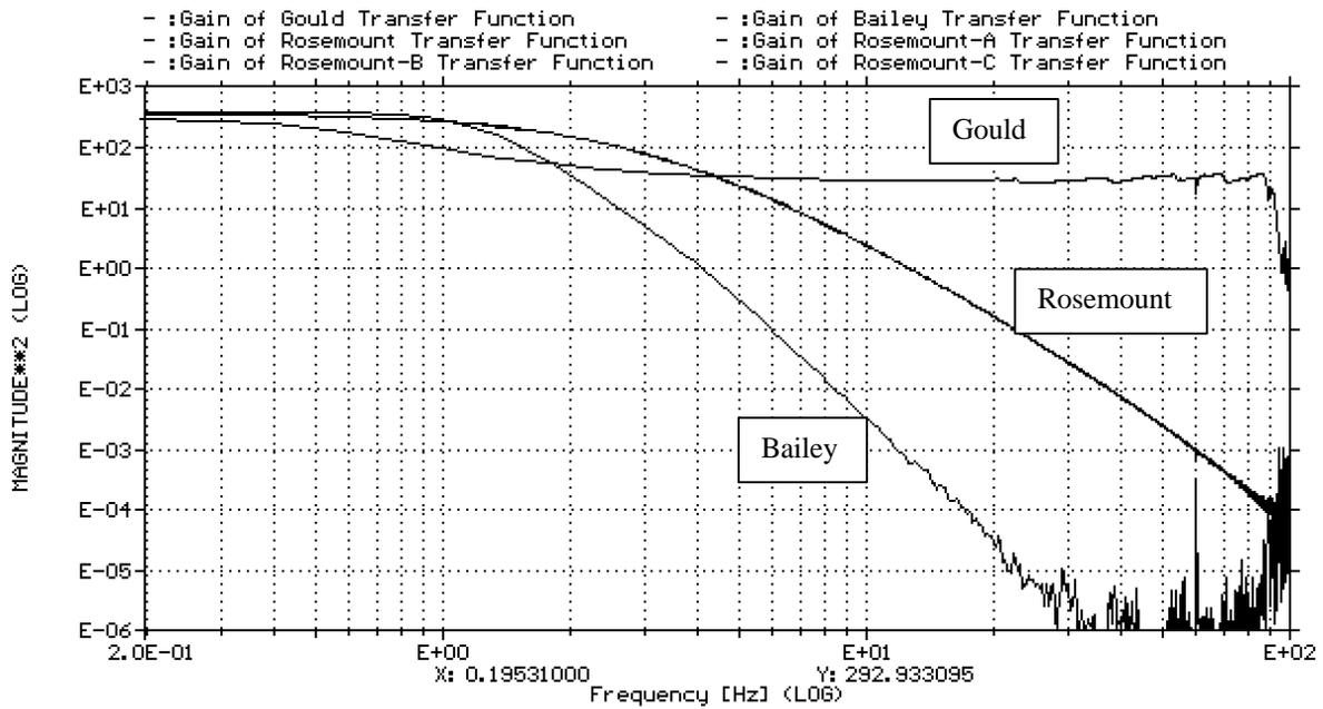
Figure 18. Magnitude of the dynamic transfer functions of Rosemount, Gould, and Bailey flow transmitters derived from in-situ noise measurements in safety system flow loop FT-3J in Darlington Unit 3.
