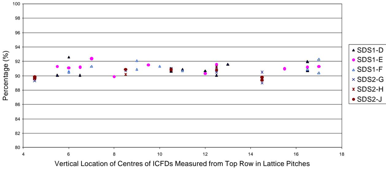
50% Level Crossing Times of SDS1 and SDS2 ICFD signals in an SDS1-trip in Pickering Unit 5 HESIR ICFD Commissioning June 1999
