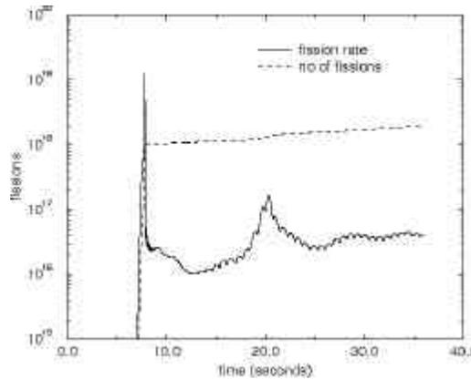
**Fig.3** Time evolution of fission rate and no. of fissions for continuously filled drum
