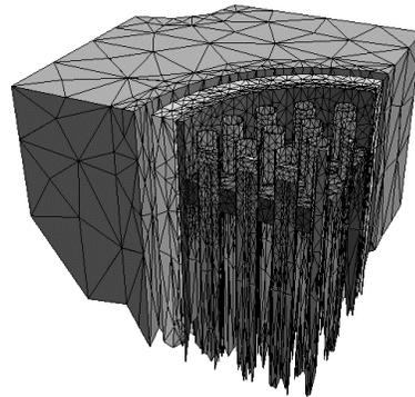
Adapted Finite Element Mesh for AGR – top section
