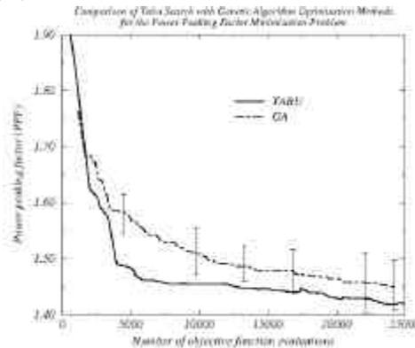
**Fig. 1** Comparison of Tabu Search with Genetic Algorithm for optimisation of PWR power peaking factor
